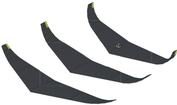
FIG 2: Different settings of the morphing wing-tip DoF.
