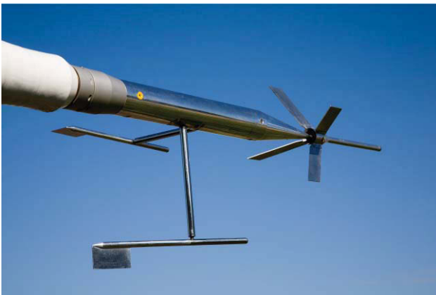
FIG.2. FHS noseboom with airflow and pitot sensors
