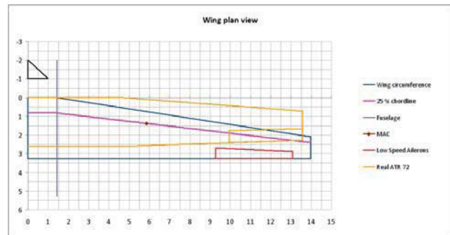
FIG 16. Wing shape V04 to real ATR 72
