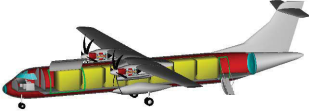
FIG 8. PrADO model of the original ATR 72 full freighter version
