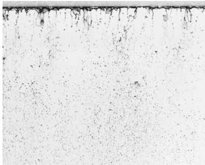
Figure 2: Airblast atomizer image. Air flow is from top to bottom
