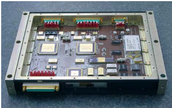
Figure 6: Channel Coding Unit Core Layout
