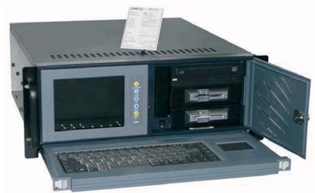
Figure 8: Ground Crypto Unit
