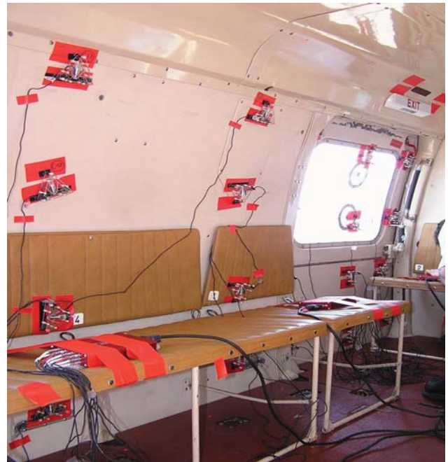
FIG. 3. 45 Sensors applied on left side of the helicopter compartment (same for right side)
