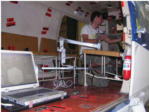
FIG. 9. Microflown 3D geometry measuring unit inside helicopter compartment
