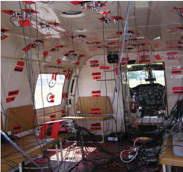
FIG. 1. 45 Sensors applied on the roof
