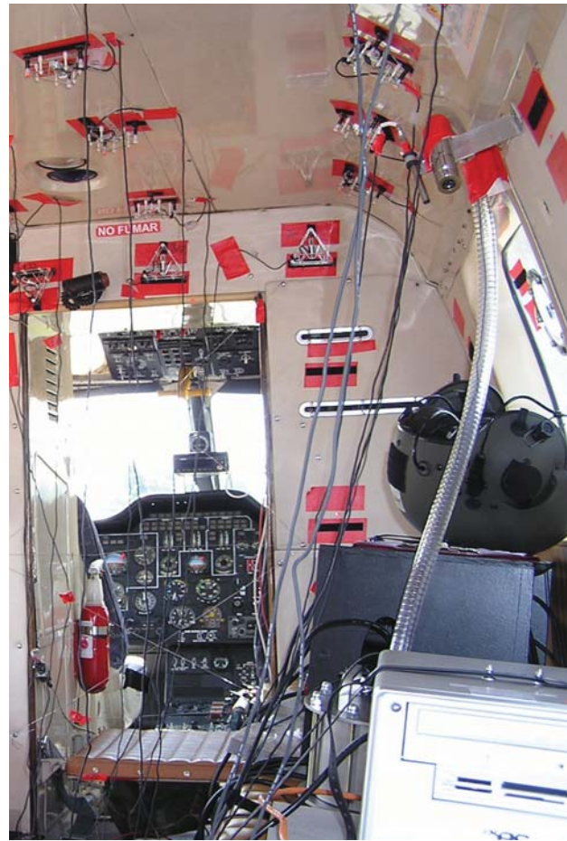
FIG. 8. Measurement of the airborne noise transfer functions
