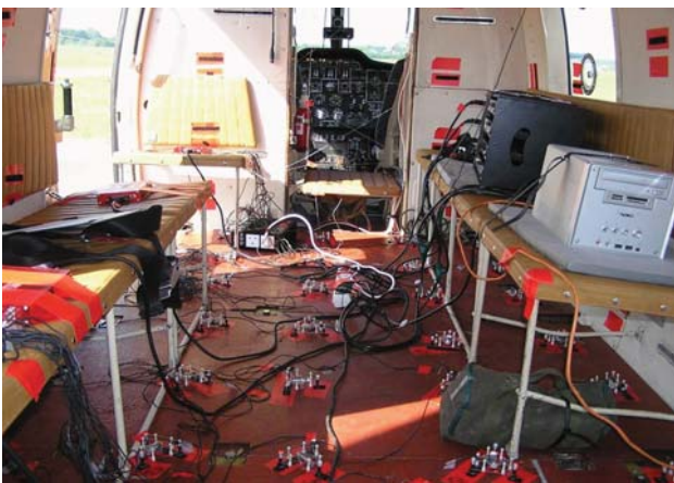
FIG. 2. 45 Sensors applied on the bottom
