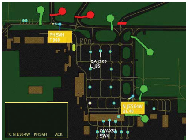
Figure 3. Controller Screen with Separation Bubble Alert
