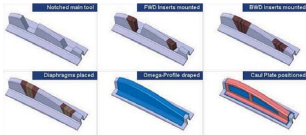
BILD 5. Schematic manufacturing and tooling concept for integrally formed diaphragms
