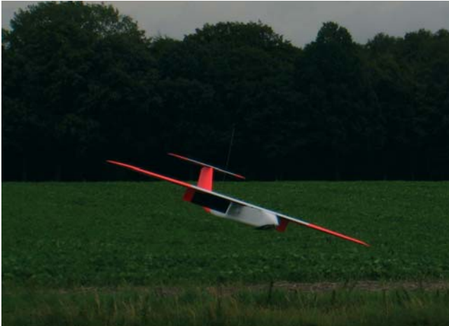
Figure 1: The mini UAV CAROLO P200 used for automated aerial photography during landing approach.
