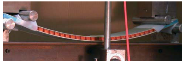
Figure 6: Foldcore sandwich beam during flexural test.
