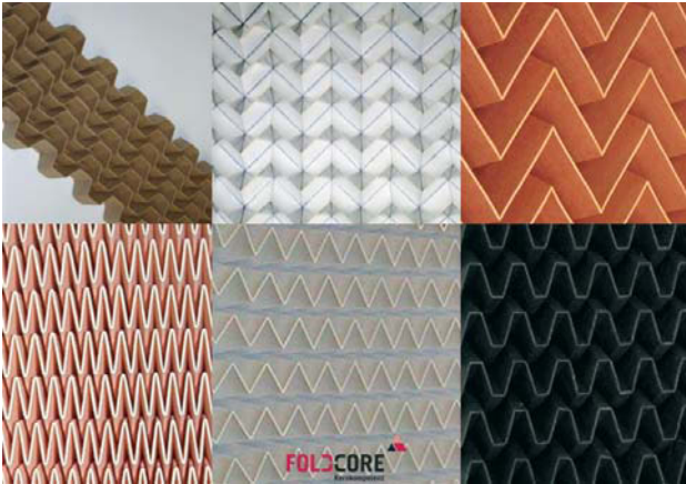
Figure 7: Foldcores made out of: paper, aluminum, aramide paper, synthetic paper, thermoplastic, CFRP.
