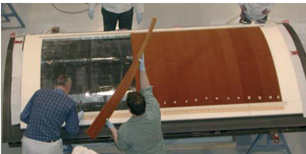
Figure 9: Cylindrical foldcore test shell: Assembly of 165.000 creases. Source: Airbus Deutschland GmbH
