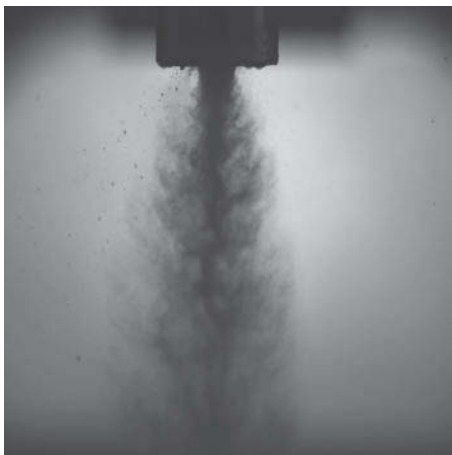
Figure 3: Shadowgraph image of impingement-dome injector spray with water
