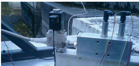
Figure 13: Frozen water on the valve with attached Venturi tube
