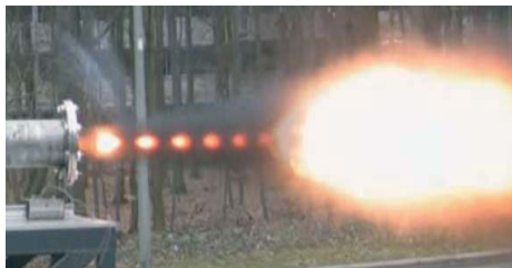
Figure 9: Under expansion and mach diamonds shortly after ignition
