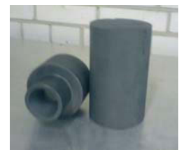
Figure 6: TOP nozzle (graphite)
