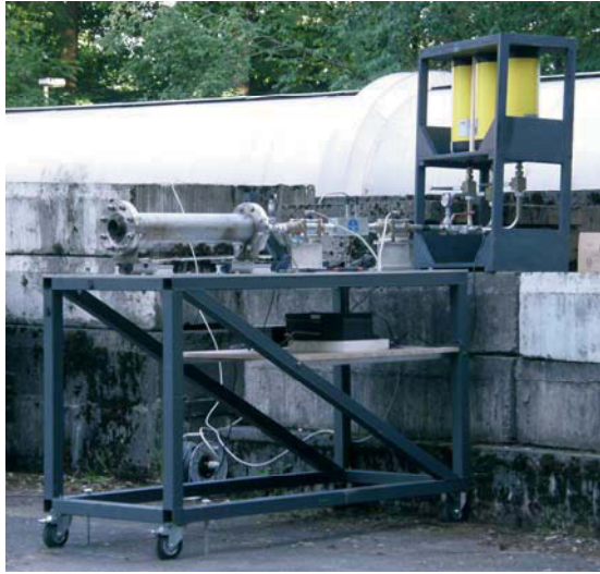
Figure 8: Mobile test bench with oxidizer supply system and engine
