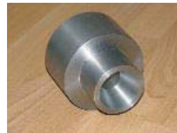
Figure 7: Laval nozzle (steel)
