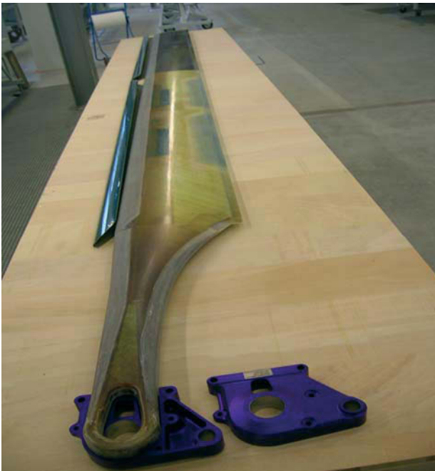
Fig. 10. The rotor blade of the EC 145 with load introduction fitting and metallic erosion strip, bonded to the composite blade structure
