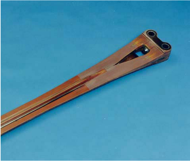
Fig. 6. 3-Dimensional structure of the EC 135 "Flex-beam" attachment, "flapping hinge" and cruciform torsional structural element (from right to left)
