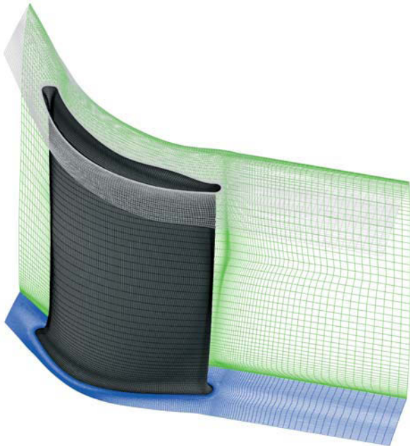
FIG 3. Details of the stator grid domain used for the HYDRA calculations.
