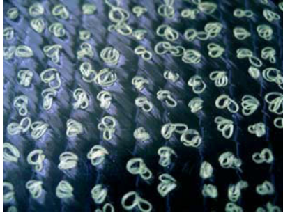
FIGURE 7. Tufting loops bonded to laminate after curing
