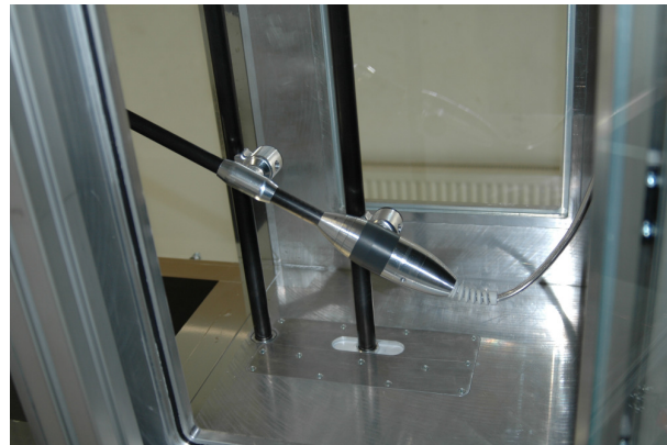
Fig. 3. Picture of model support applied in wind tunnel
