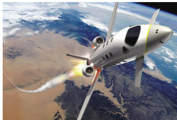
FIG 12. EADS Astrium single stage suborbital space tourism vehicle [11]
