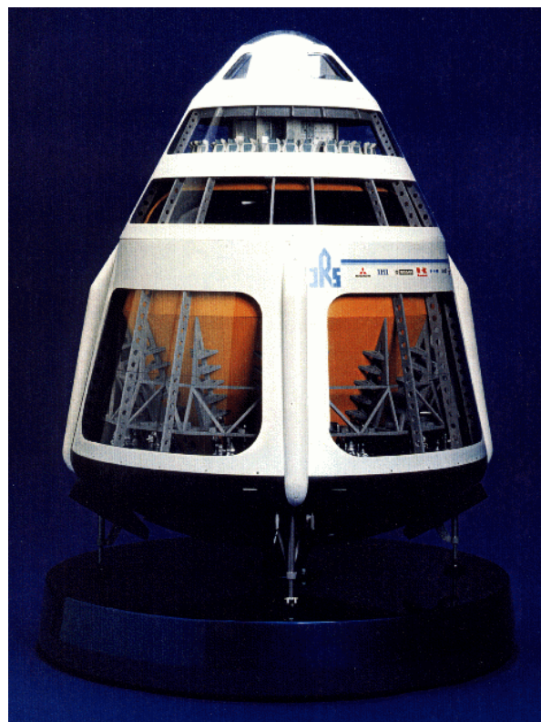
FIG 13. Kankoh Maru SSTO Passenger Carrier (50 passengers, 550t GLOW, 50t dry weight) [12]
