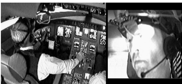
FIG. 3: Eye movement analysis system "SMI iView X HED"
