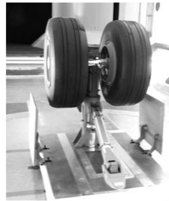
Figure 8 1/3 scaled A340 centre landing gear in the Airbus Filton low speed wind tunnel
