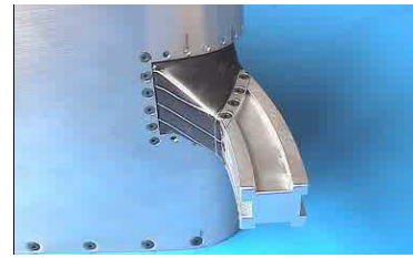
Figure 10 Low noise slat track/wing-cut-out modification
