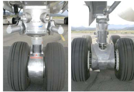
Figure 1 A340 nose and main landing gears with noise reduction add-on fairings for flight test evaluation
