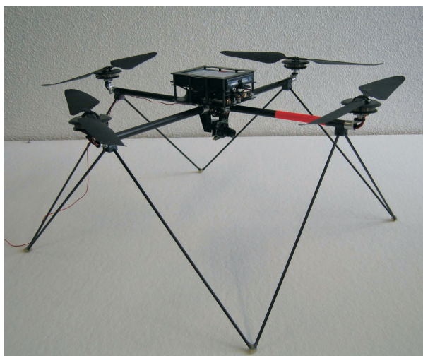
Fig. 1: The UAV with the camera used for acquiring image data. Take-off weight is below 1 kg, diameter is 52 cm.
