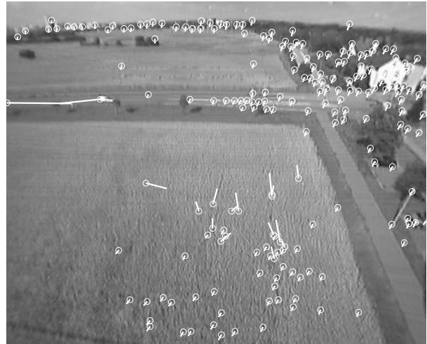
Fig. 2: One frame of a preprocessed UAV-camera sequence with tracked feature points.
