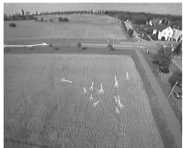
Fig. 3: The outliers: wrongly matched feature pairs and features belonging to a moving car.
