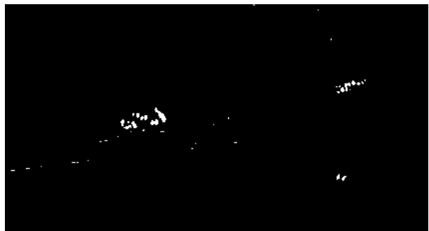
Fig. 6: Differential image after applying a threshold.
