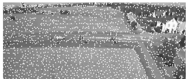
Fig. 9: Extracted feature points for calculating a relatively dense optical flow field.
