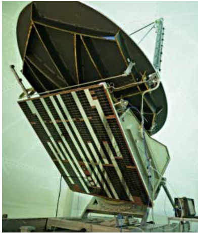
Figure 7: OHB SAR-Sat Platform (SAR-Lupe mission)
