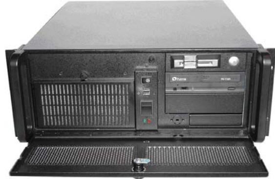
Figure 17: GCU case with Session Key Smartcard slot
