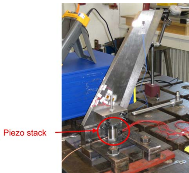
Figure 17: Basic excitation test with a pre-model
