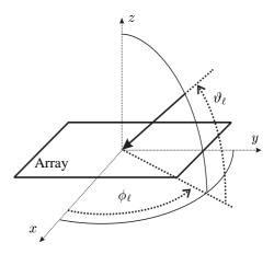
**Fig. 1.** Definitions of Azimuth  $(-180^{\circ} < \phi_{\ell} \le 180^{\circ})$  and Elevation  $(0^{\circ} \le \vartheta_{\ell} \le 90^{\circ})$ .
