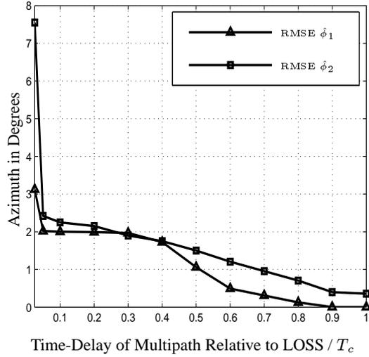
**Fig. 7.** RMSE of the azimuth of the LOSS and the multipath versus its relative time-delay  $/ T_c$ . Parameters:  $L = 2$ ,  $M = 9$ ,  $\phi_1 = -24^\circ$ ,  $\vartheta_1 = 30^\circ$ ,  $\phi_2 = 10^\circ$ ,  $\vartheta_2 = 20^\circ$ .
