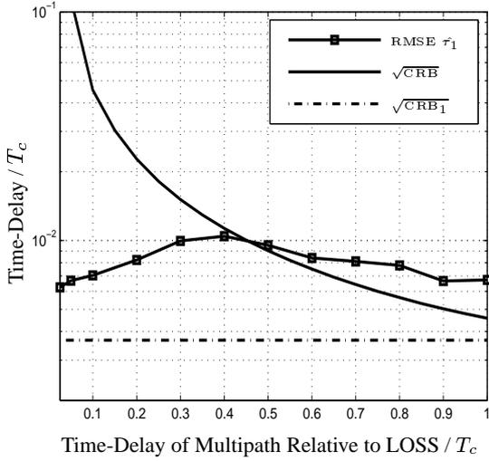
**Fig. 5.** RMSE of the time-delay of the LOSS  $/ T_c$  versus the relative time-delay of the multipath  $/ T_c$ . Parameters:  $L = 2$ ,  $M = 9$ ,  $\phi_1 = -24^\circ$ ,  $\vartheta_1 = 30^\circ$ ,  $\phi_2 = 10^\circ$ ,  $\vartheta_2 = 20^\circ$ .
