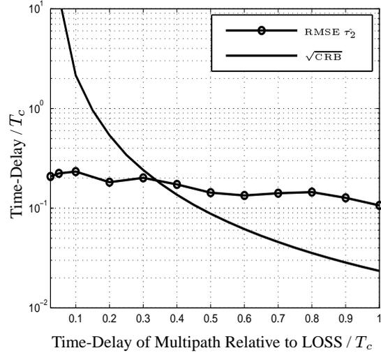
**Fig. 4.** RMSE of the time-delay of the multipath /  $T_c$  versus its relative time-delay /  $T_c$ . Parameters:  $L = 2$ ,  $M = 1$ .
