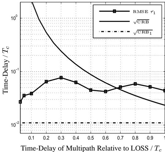
**Fig. 3.** RMSE of the time-delay of the LOSS /  $T_c$  versus the relative time-delay of the multipath /  $T_c$ . Parameters:  $L = 2$ ,  $M = 1$ .
