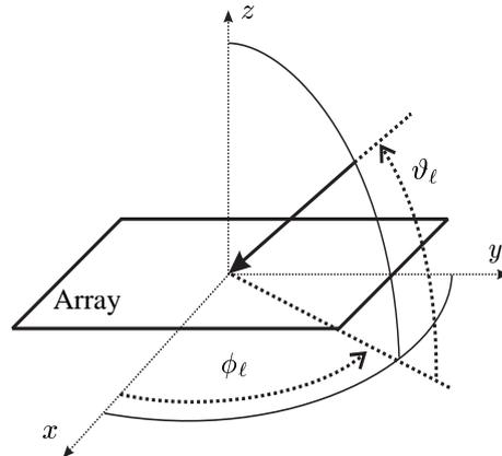
**Fig. 1.** Definitions of Azimuth ( $-180^\circ < \phi_\ell \leq 180^\circ$ ) and Elevation ( $0^\circ \leq \vartheta_\ell \leq 90^\circ$ ).
