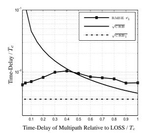
**Fig. 5**. RMSE of the time-delay of the LOSS /  $T_c$  versus the relative time-delay of the multipath /  $T_c$ . Parameters:  $L=2,~M=9,~\phi_1=-24^\circ,~\vartheta_1=30^\circ,~\phi_2=10^\circ,~\vartheta_2=20^\circ.$
