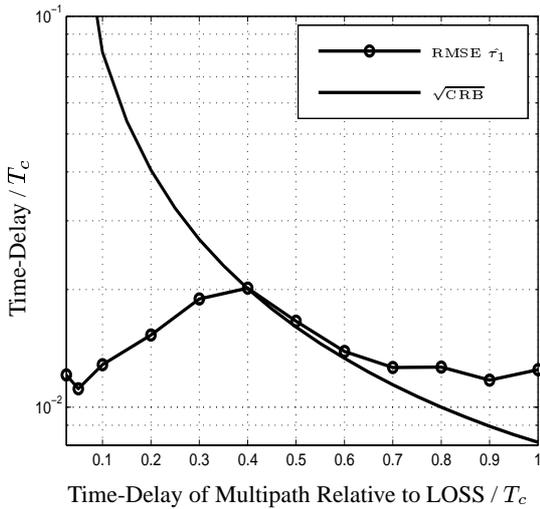
**Fig. 6.** RMSE of the time-delay of the multipath  $/ T_c$  versus its relative time-delay  $/ T_c$ . Parameters:  $L = 2$ ,  $M = 9$ ,  $\phi_1 = -24^\circ$ ,  $\vartheta_1 = 30^\circ$ ,  $\phi_2 = 10^\circ$ ,  $\vartheta_2 = 20^\circ$ .
