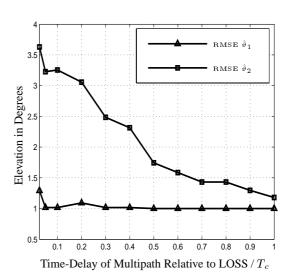
**Fig. 8**. RMSE of the elevation of the LOSS and the multipath versus the relative time-delay of the multipath /  $T_c$ . Parameters:  $L=2,~M=9,~\phi_1=-24^\circ,~\vartheta_1=30^\circ,~\phi_2=10^\circ,~\vartheta_2=20^\circ.$
