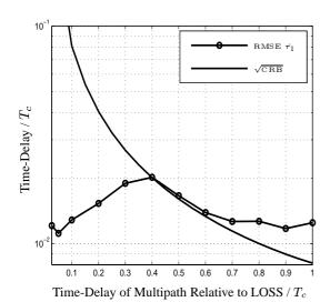
**Fig. 6.** RMSE of the time-delay of the multipath /  $T_c$  versus its relative time-delay /  $T_c$ . Parameters: L=2, M=9,  $\phi_1=-24^\circ$ ,  $\vartheta_1=30^\circ$ ,  $\phi_2=10^\circ$ ,  $\vartheta_2=20^\circ$ .
