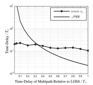
**Fig. 4.** RMSE of the time-delay of the multipath /  $T_c$  versus its relative time-delay /  $T_c$ . Parameters: L=2, M=1.
