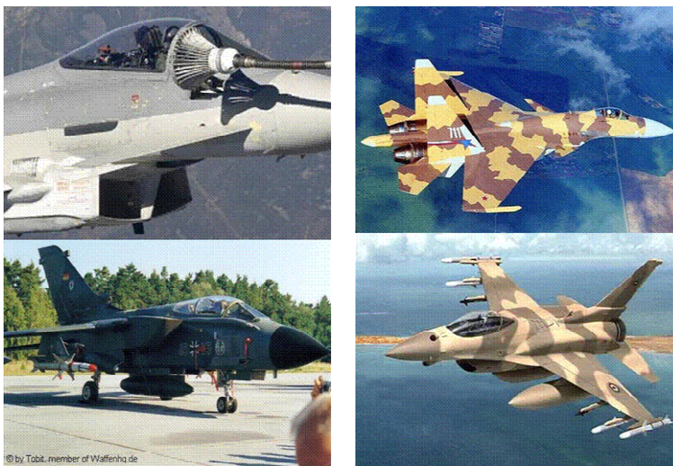
Fig. 4.5-2 Optical Signature Reduction by Camouflage Paint
