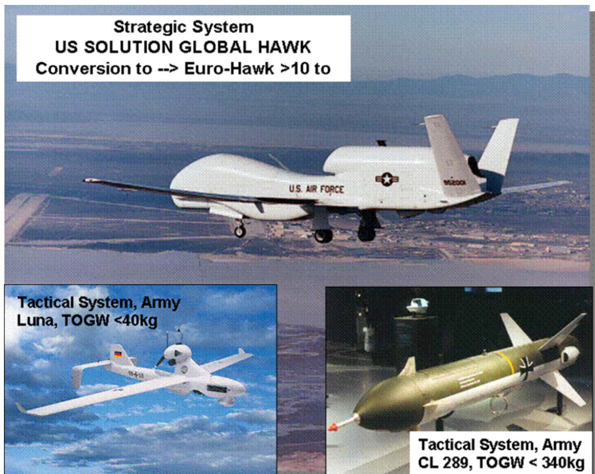
Fig. 5-14 Range of UAV's in use or planned for the German forces.
