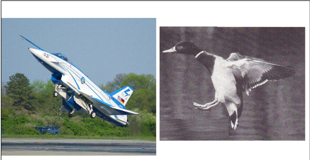
Fig. 4.4-31 Landing attitude at 24° approach, just before derotation
