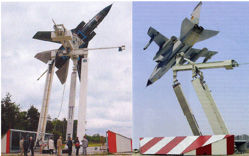
Fig. 4.5-22 Tornado RCS Tests, Manching
