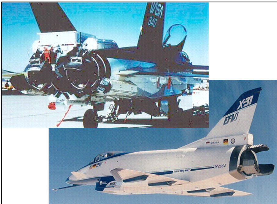
Fig. 4.4-17 General arrangement of TV vanes at X-31 and F-18 HARV
