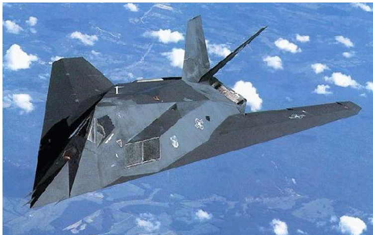
Fig. 4.5-11 First operational low signature aircraft: F-117, Lockheed
