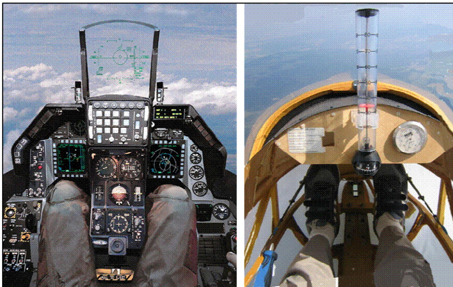
Fig. 4.2-2 Pilot Seating in an F-16 and an Ultra Light sailplane
