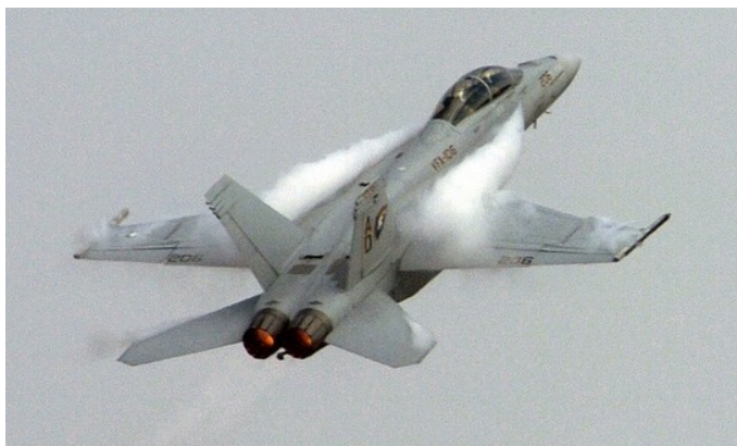
Fig. 3-13 F-18 Leading Edge Vortex Generation
