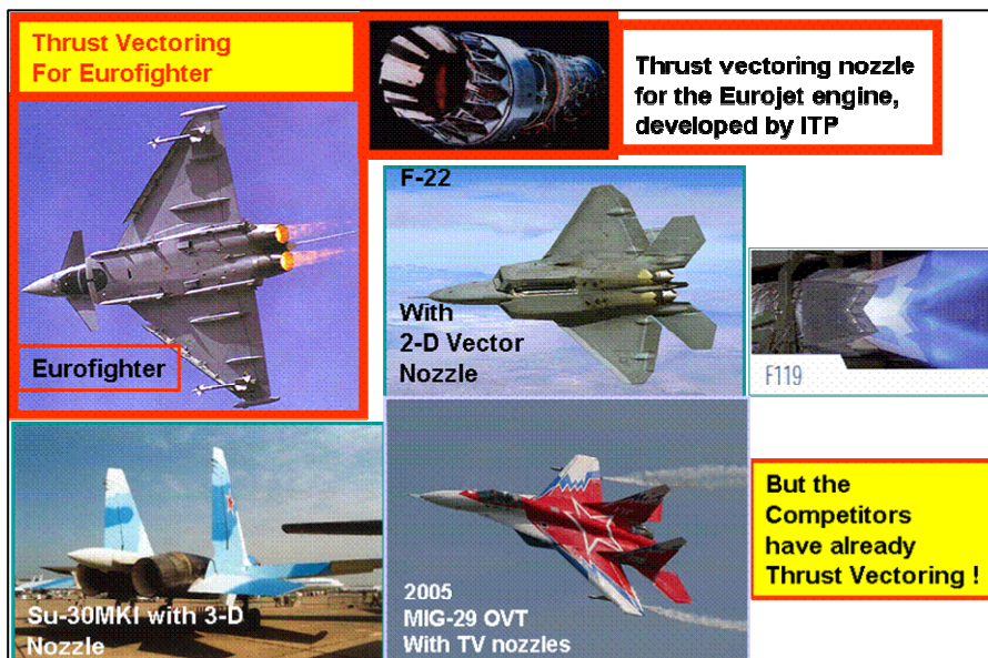
Fig. 4.4-32 Thrust Vectoring is a reality and used on operational aircraft of the US and Russia
