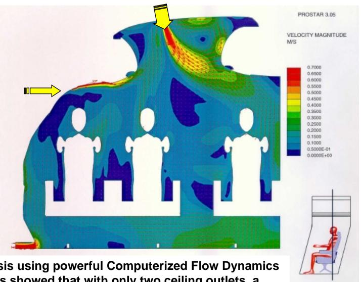
Extensive analysis using powerful Computerized Flow Dynamics (CFD) techniques showed that with only two ceiling outlets, a comparable comfort level with the A340-300 was not achievable
