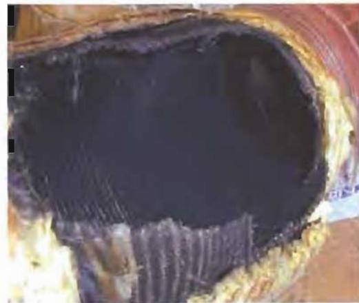
**A used duct removed from a BAE 146 airplane with a history of cabin odours but no reported crew symptoms (the duct had accumulated 26,061 flight hours)**
