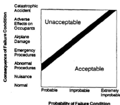
Figure 1: AMC - Probability vs Severity
