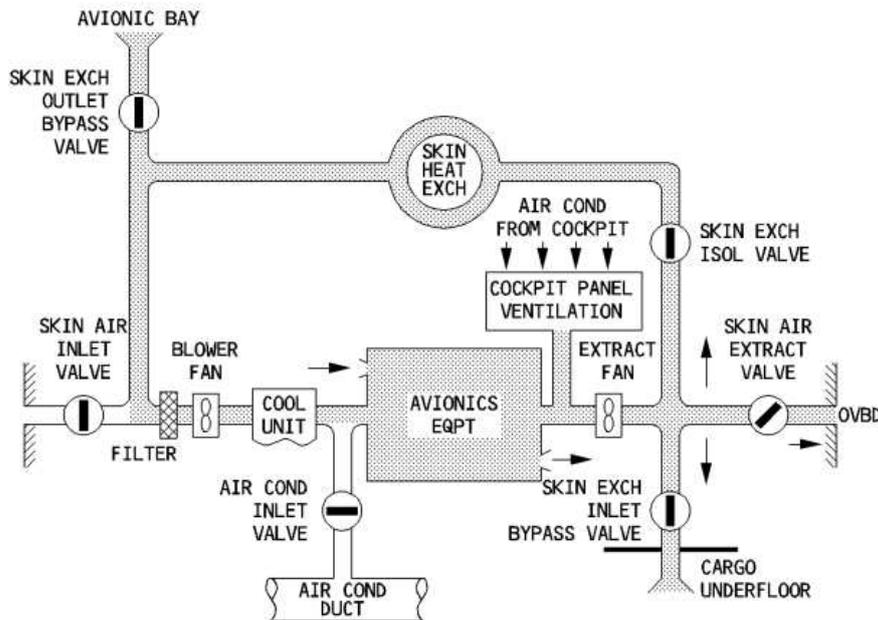
**Figure 4.5** Avionics ventilation, normal operation, intermediate config., Airbus A320, Smart Cockpit 2021a
