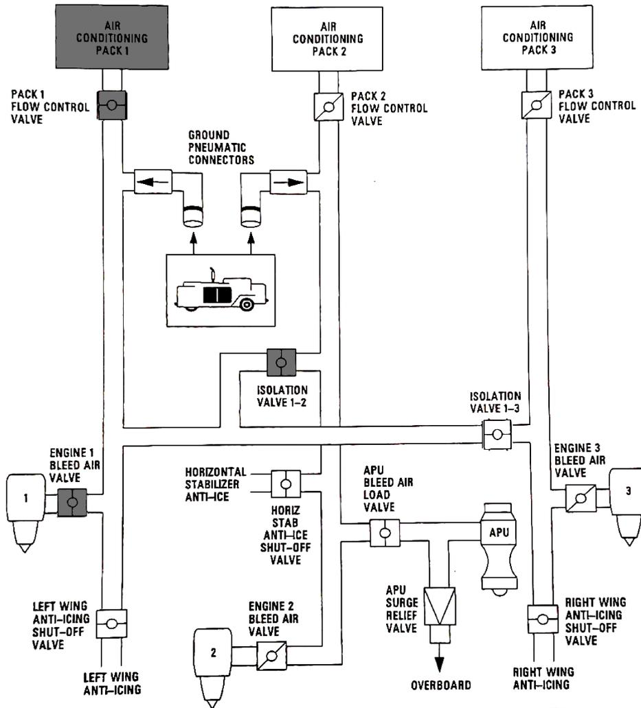
**Figure 4.22** Engine 1 Bleed air and Pack 1 off, 1-3 ISOL valve open, McDonnell Douglas MD-11, based on McDonnell Douglas 1993
