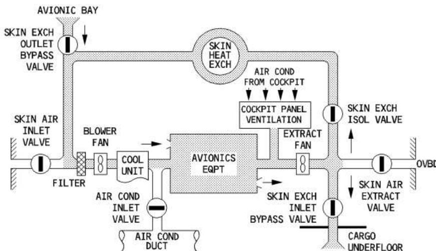
**Figure 4.4** Avionics ventilation, normal operation, close-circuit config., Airbus A320, Smart Cockpit 2021a
