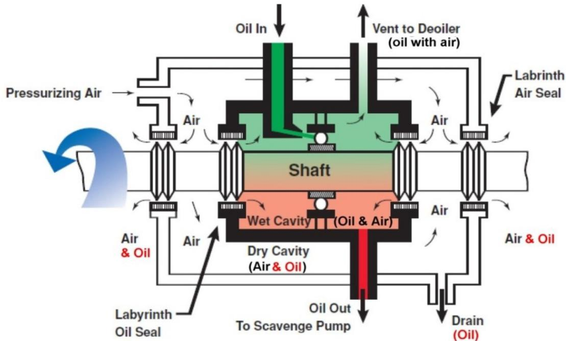
**Figure 2.2** Schematic of the lubrication and sealing system of the shaft bearings, Scholz 2019b
