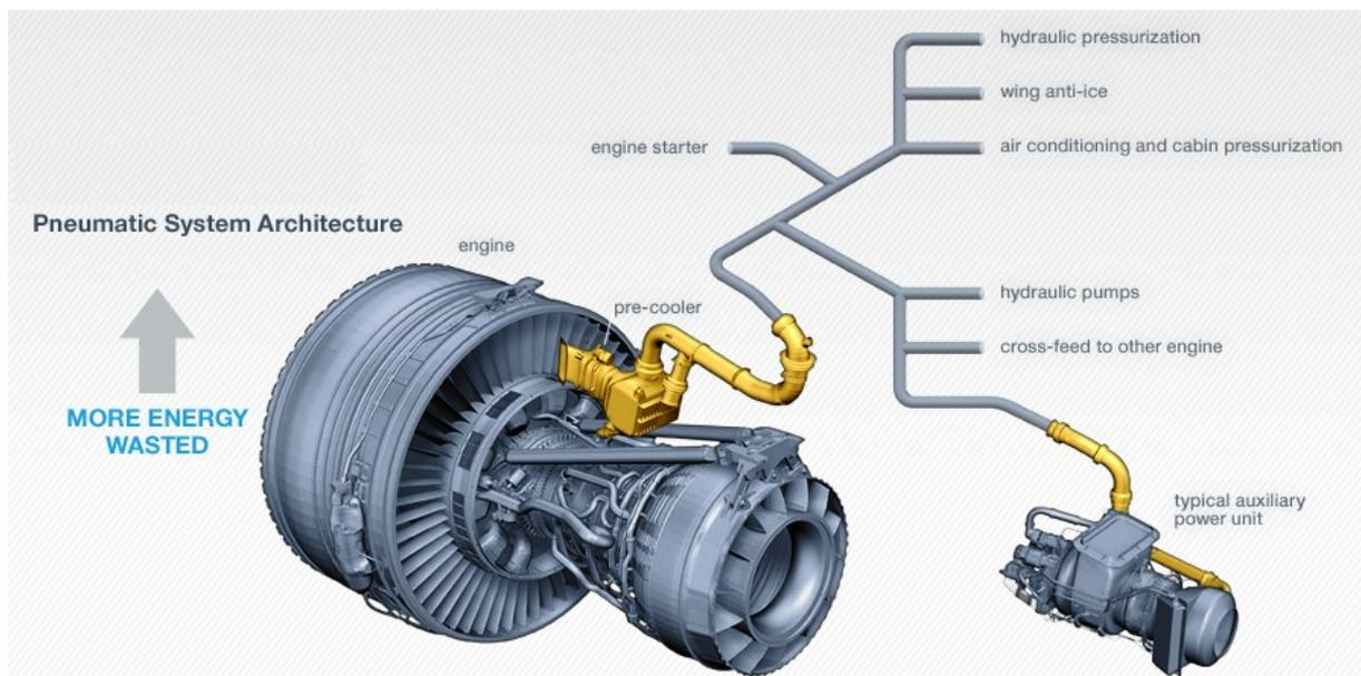
**Figure 2.1** Classical mixed bleed and electrical architecture with pre-cooler in pylon, Fehrm 2016
