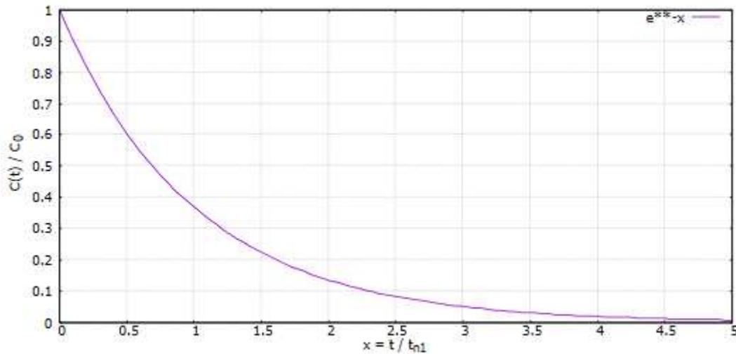
**Figure 4.30** Relative remaining concentration for a ventilation efficiency of  $\eta = 1$  over relative time, Scholz 2020b
