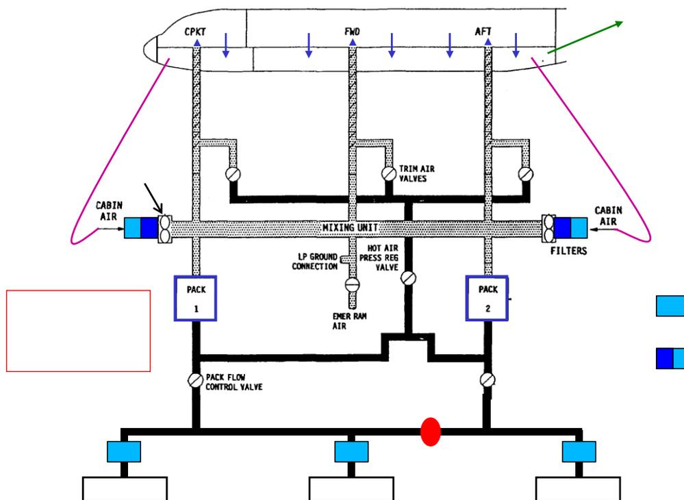
Figure 2.3 Filtration of cabin air option 1, Scholz 2018
