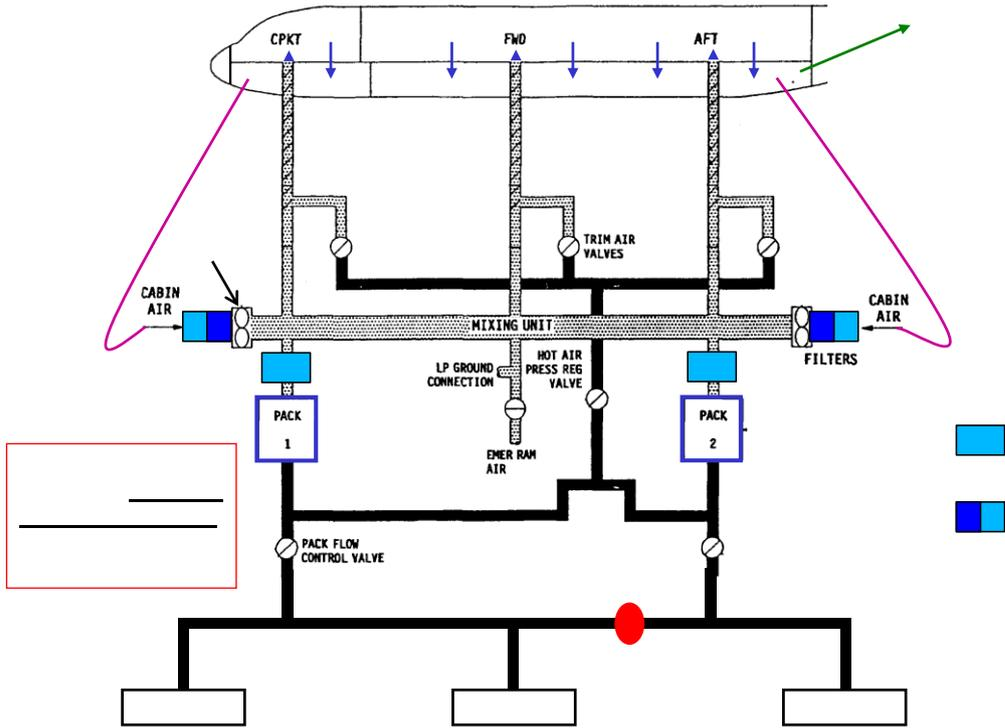
Figure 2.6 Filtration of cabin air option 3b, Scholz 2018
