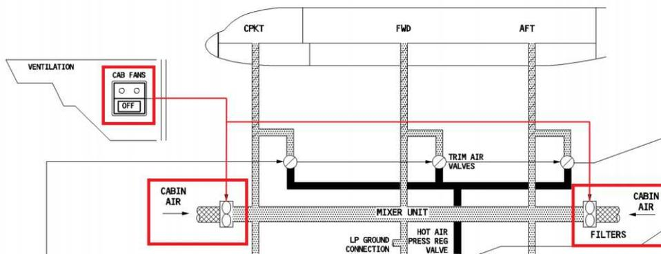
**Figure 4.3** CAB FANS off, Airbus A320, Smart Cockpit 2021a
