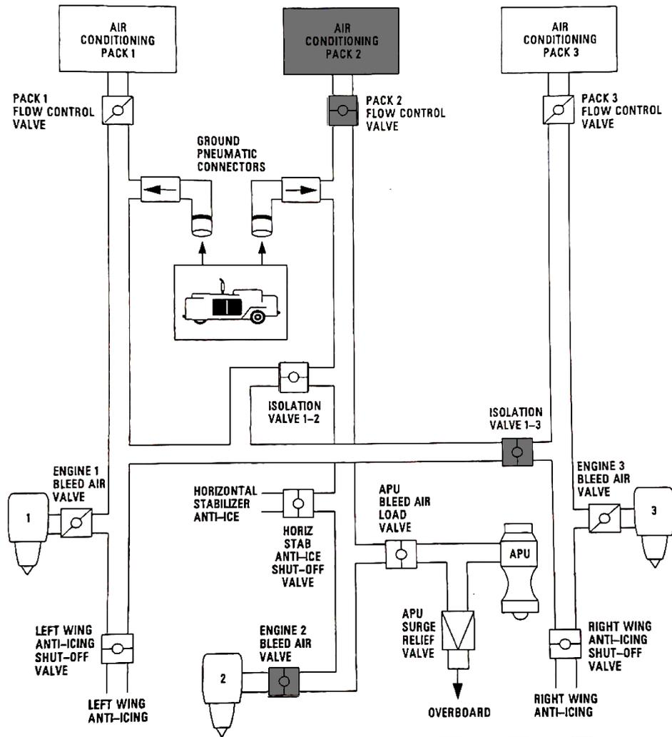
**Figure 4.24** Engine 2 Bleed air and Pack 2 off, 1-2 ISOL valve open, McDonnell Douglas MD-11, based on McDonnell Douglas 1993
