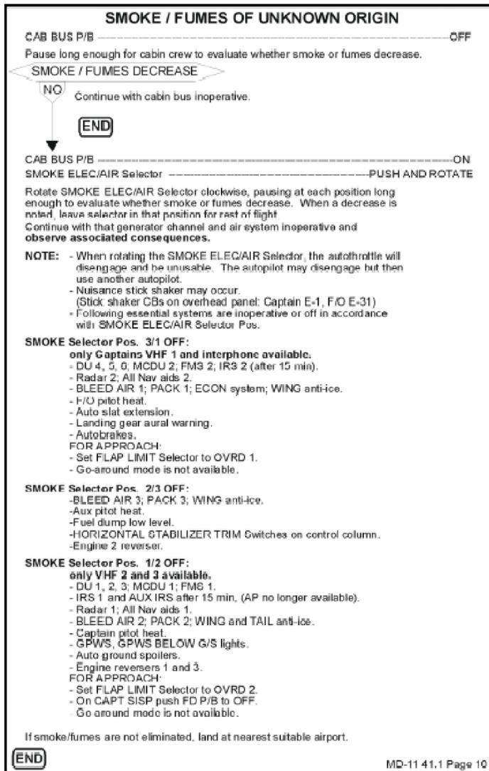
**Figure 4.25** EMC checklist smoke/fumes of unknown origin, McDonnell Douglas (Boeing) MD-11, Burian 2021
