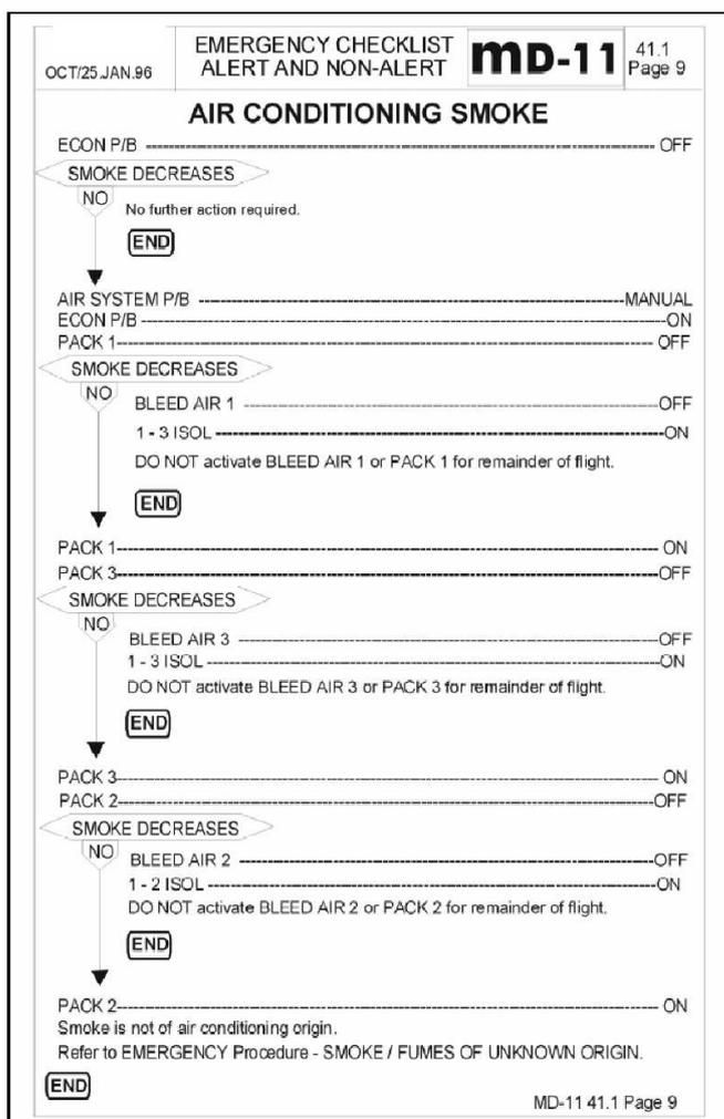
**Figure 4.18** EMC checklist air conditioning smoke, McDonnell Douglas MD-11, Burian 2021
