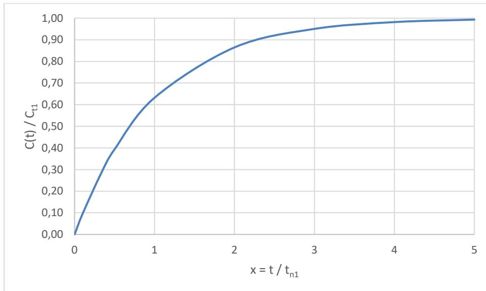
**Figure 4.34** Relative concentration development for a ventilation efficiency of  $\eta = 1$  over relative time
