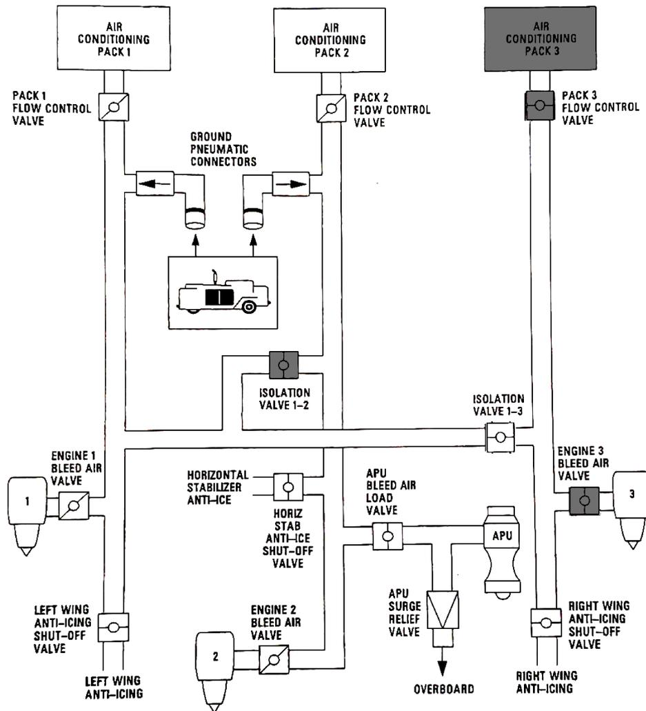
**Figure 4.23** Engine 3 Bleed air and Pack 3 off, 1-3 ISOL valve open, McDonnell Douglas MD-11, based on McDonnell Douglas 1993)
