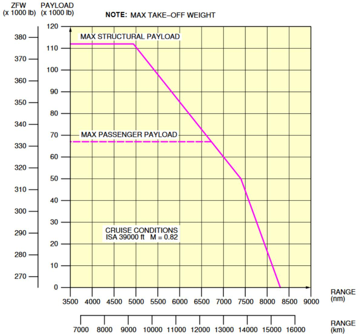
**Figure 5.4** Payload Range Diagram, A340-300, Airbus 2020
