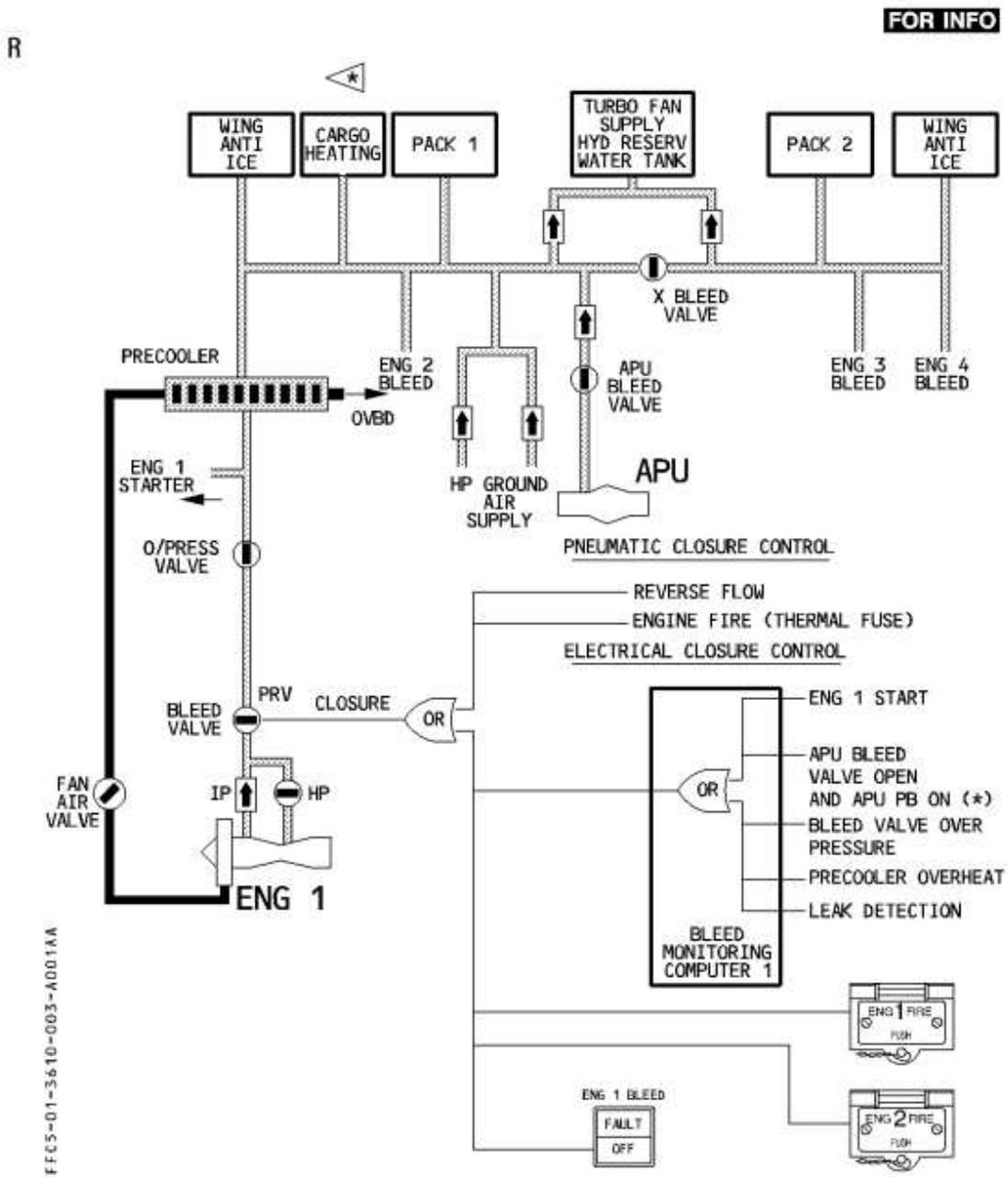
**Figure 4.12** Airbus A340, pneumatics, pneumatic closure control, Smart Cockpit 2021e
