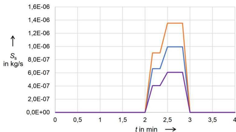
**Figure 4.31** TCP source strengths related to secondary event at S0, S1A and S1B, Lakies 2019a
