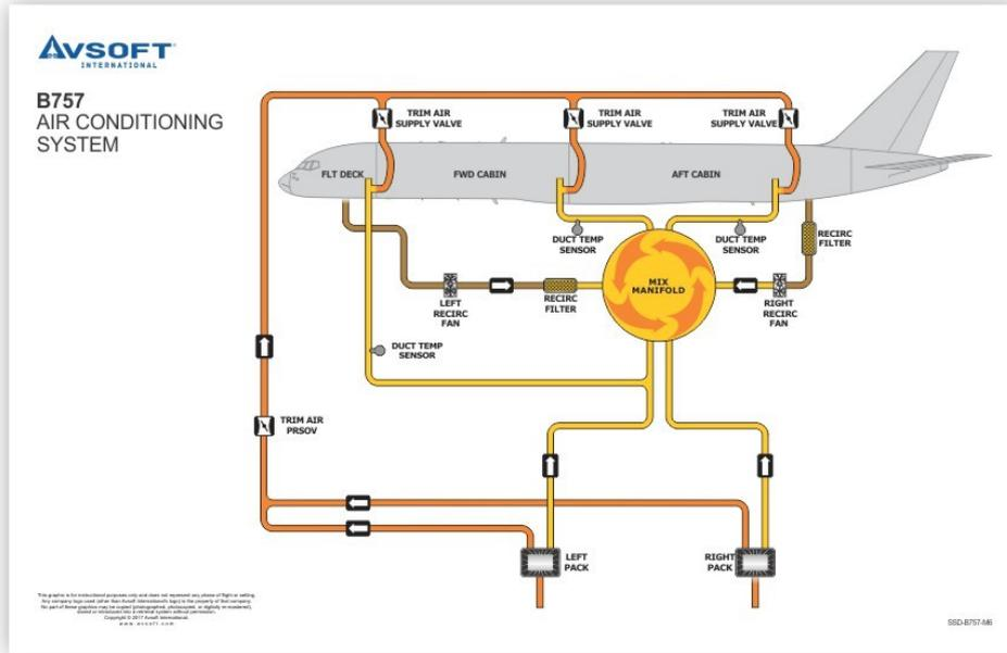
Figure 4.27 Boeing 757 Air Conditioning System, Avsoft 2018a
