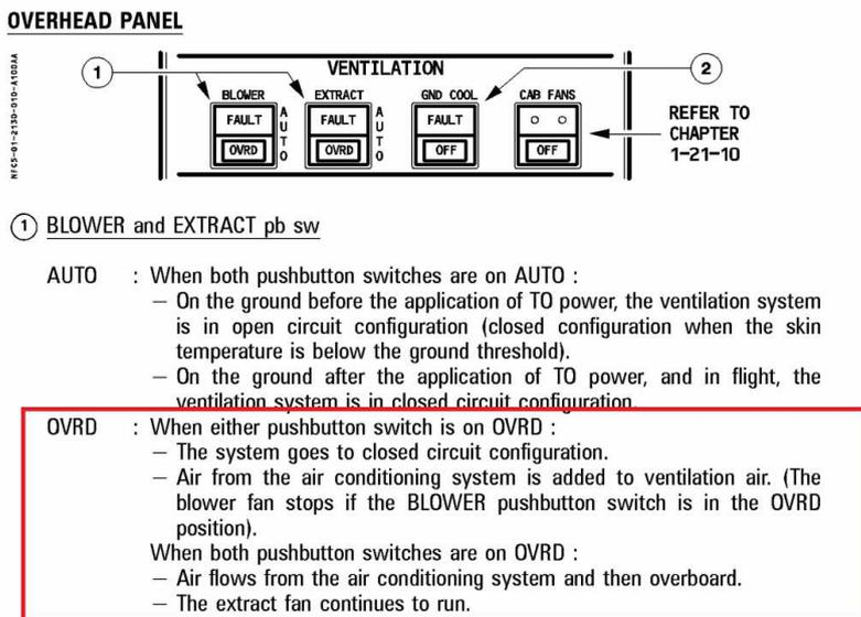
Figure 4.7 Overwrite Position BLOWER and EXTRACT Pushbutton, Overhead Panel, Airbus A320, Smart Cockpit 2021a
