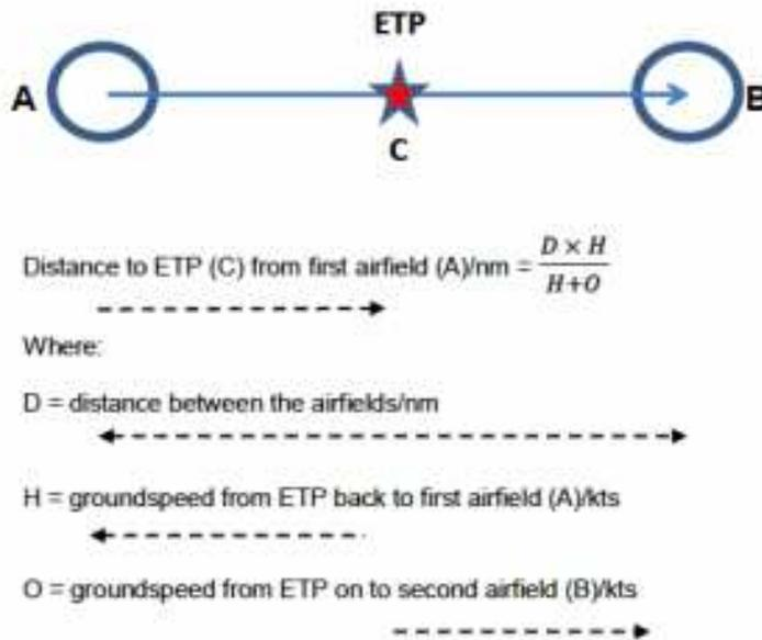
**Figure 5.7** Algebraic method for calculating Critical Point/Equal Time Point, SKYbrary 2017
