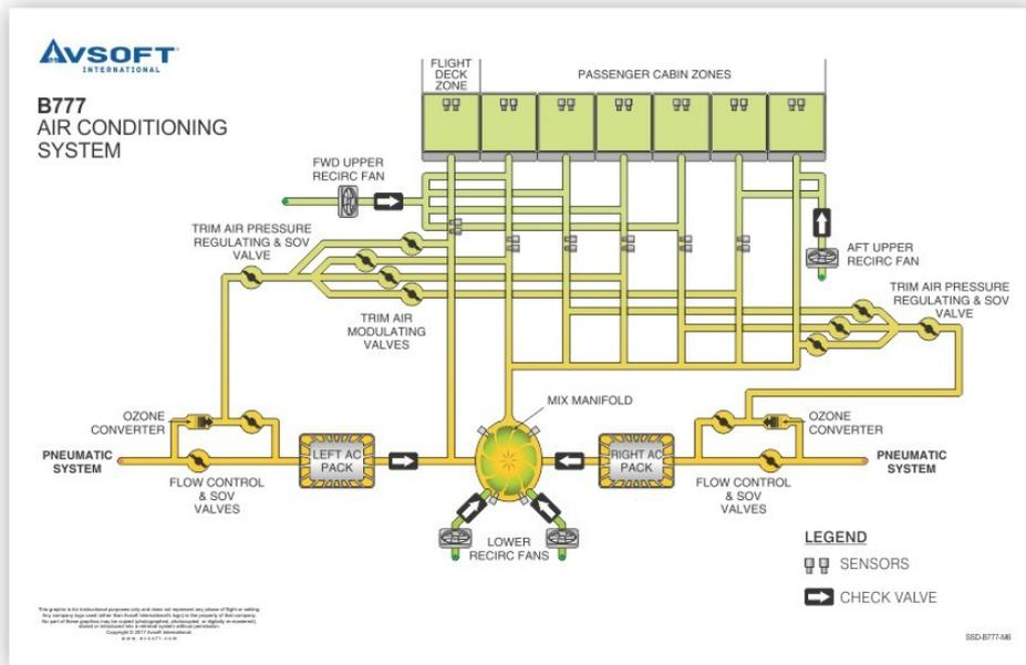
Figure 4.28 Boeing 777 Air Conditioning System, Avsoft 2018b
