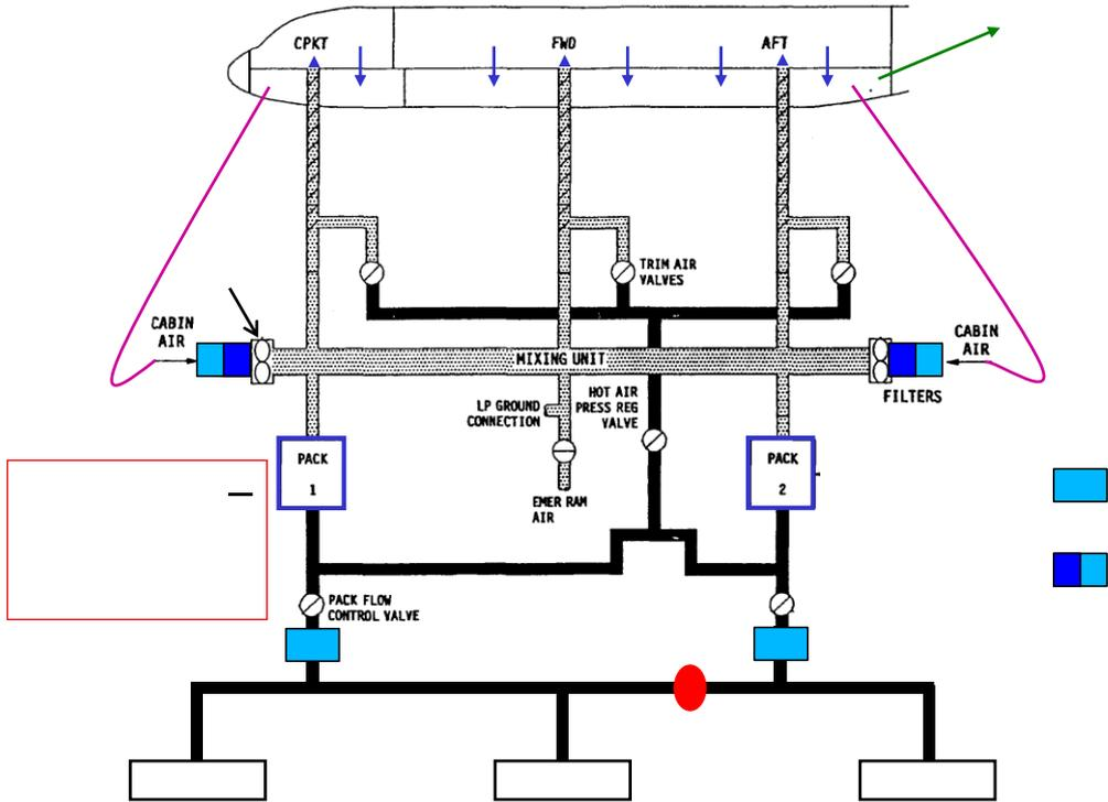
Figure 2.4 Filtration of cabin air option 2, Scholz 2018
