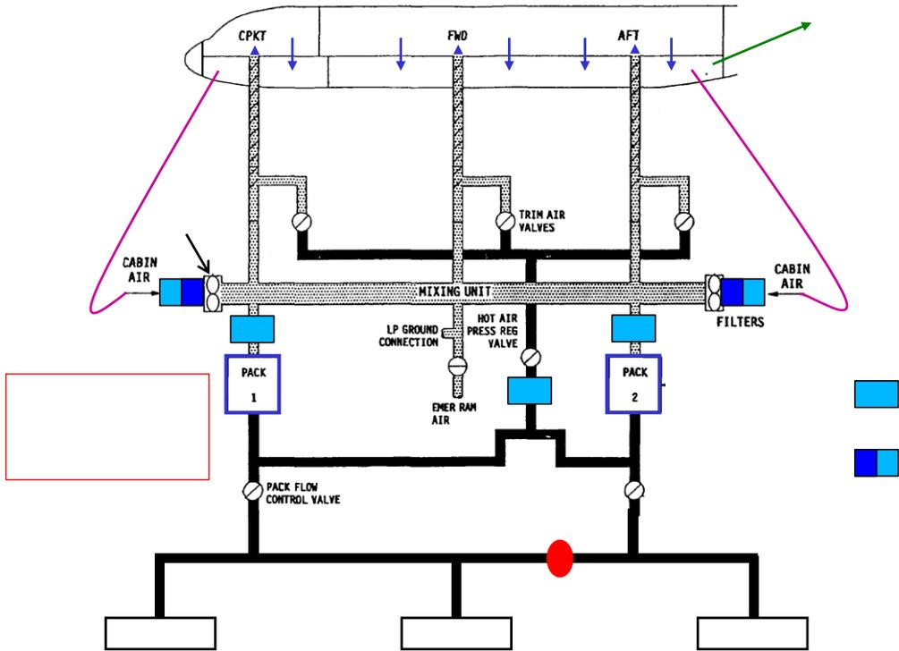
Figure 2.5 Filtration of cabin air option 3a, Scholz 2018
