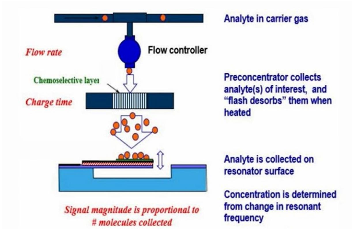
**Figure 3.2** Schematic structure of the PALL cabin air quality sensor, Mlcak 2019
