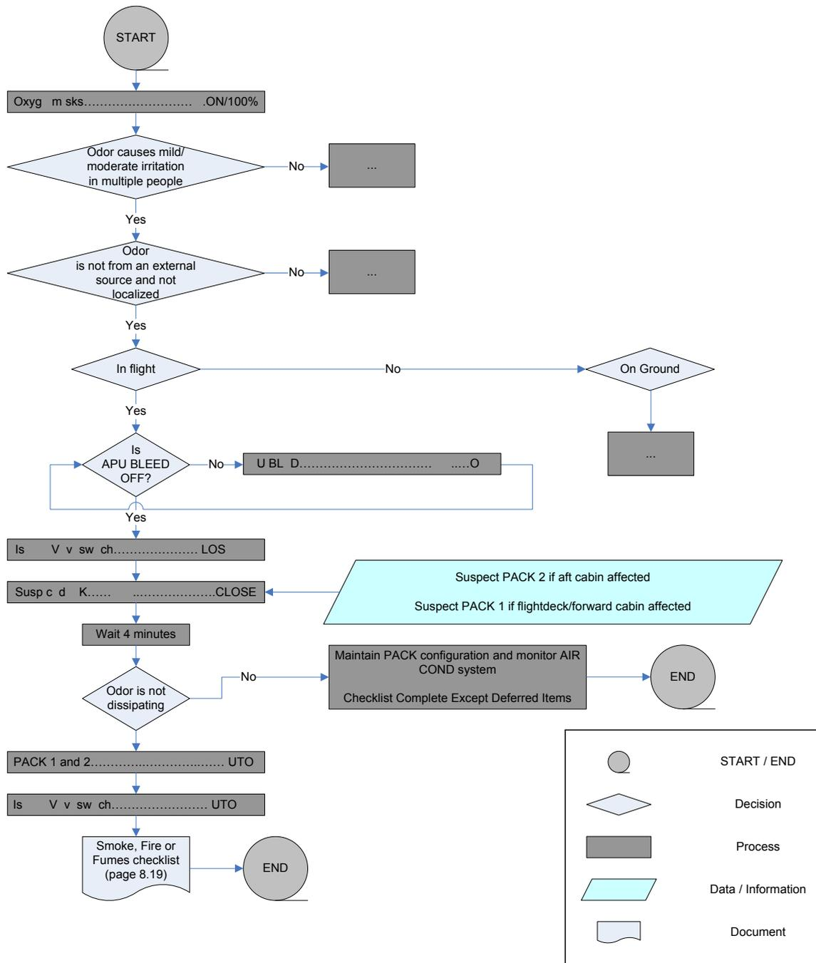
**Figure 4.29** EMC Checklist odors/toxic substances/volatile liquid, American Airlines, Boeing B737, based on Appendix A
