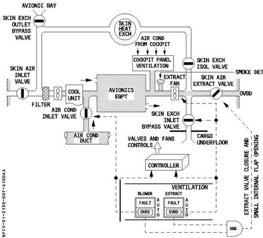
Figure 4.6 Avionics ventilation, smoke config., Airbus A320, Smart Cockpit 2021a
