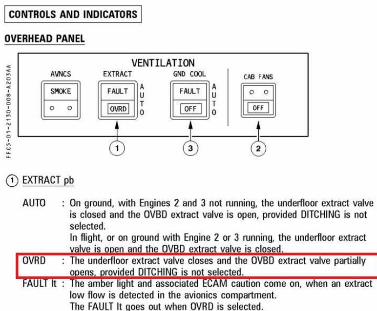
**Figure 4.8**      Overwrite position VENT EXTRACT Pushbutton, Overhead Panel, Airbus A340, Smart Cockpit 2021c
