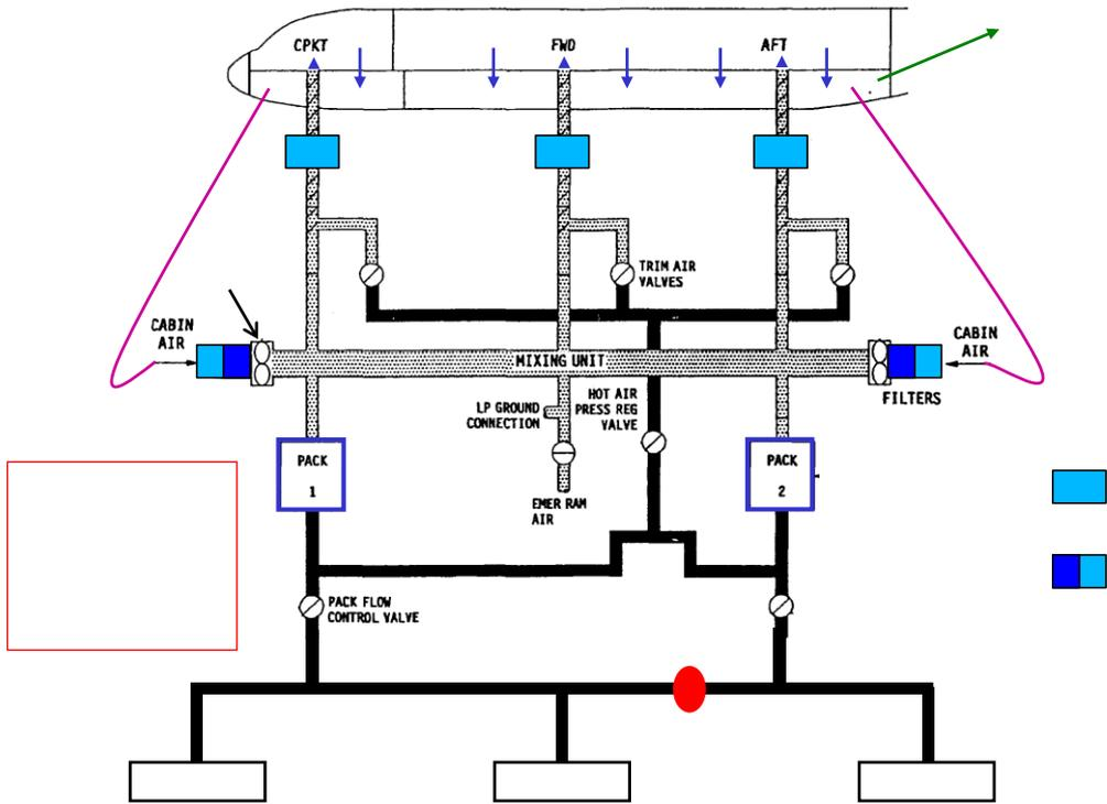
Figure 2.7 Filtration of cabin air option 4, Scholz 2018
