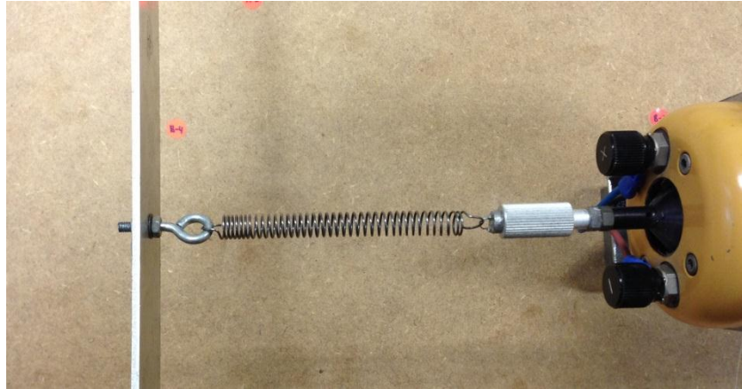
Figure 3-24 Mounting and installation of the minishaker
