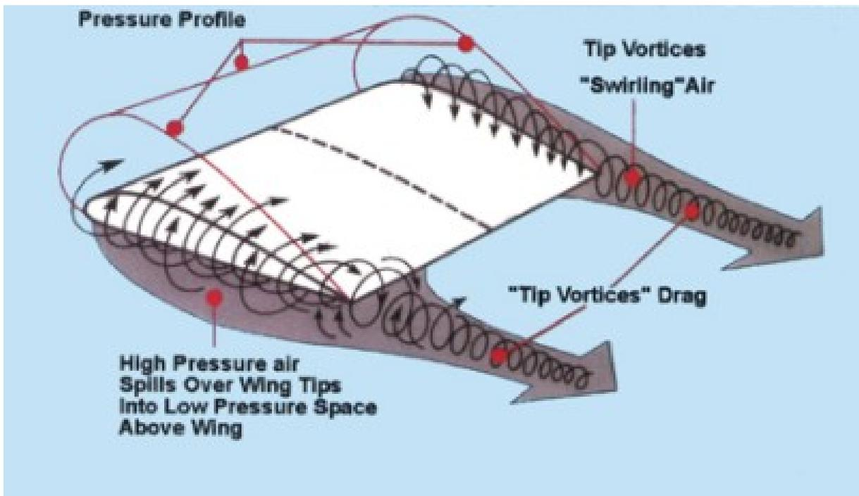
**Figure 8.3** Wingtip vortices generated by the difference of pressure between the two parts of the airfoil. Image taken from **Pilotfriend (2000)**
