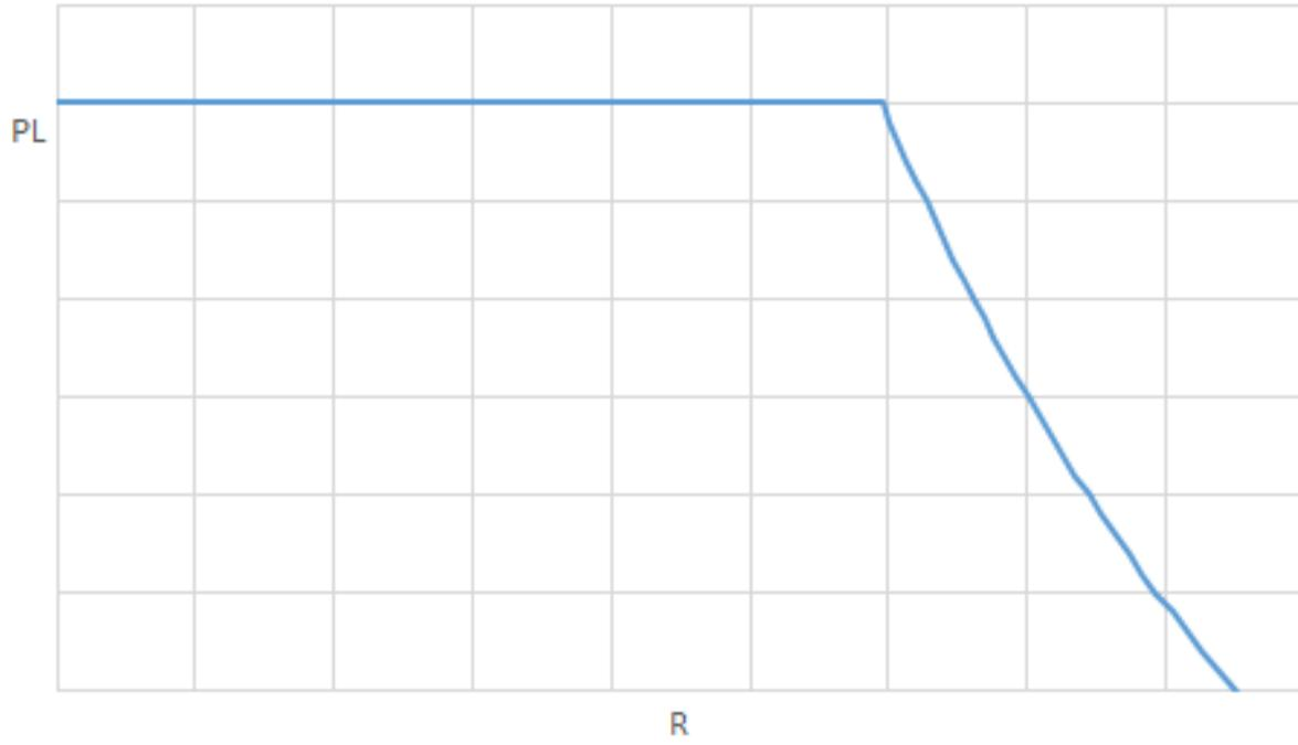
**Figure 3.3** Payload-Range diagram in a battery powered airplane.
