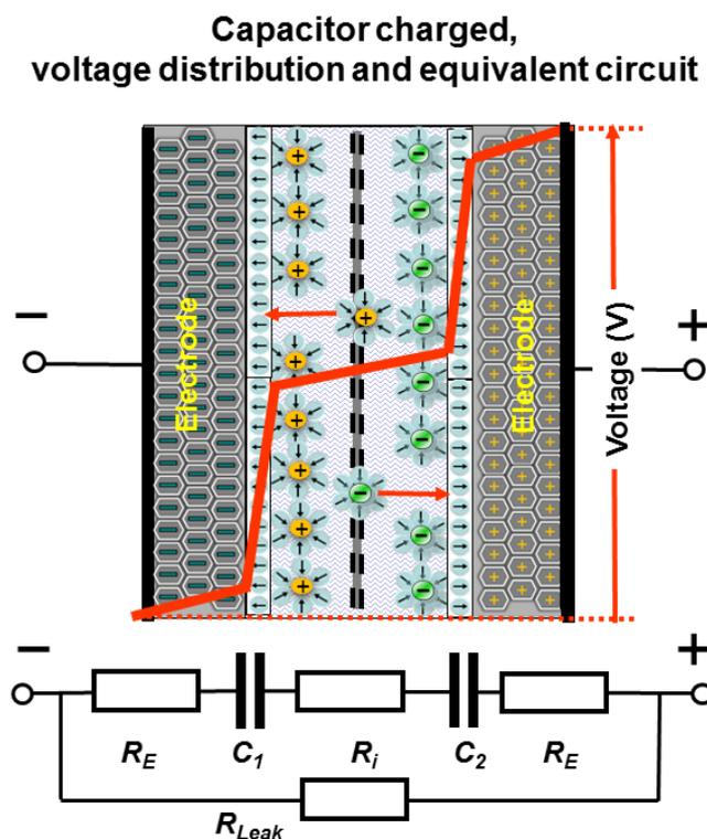
**Figure 2.4** Supercapacitor Scheme taken from **Elcap (2013b)**.
