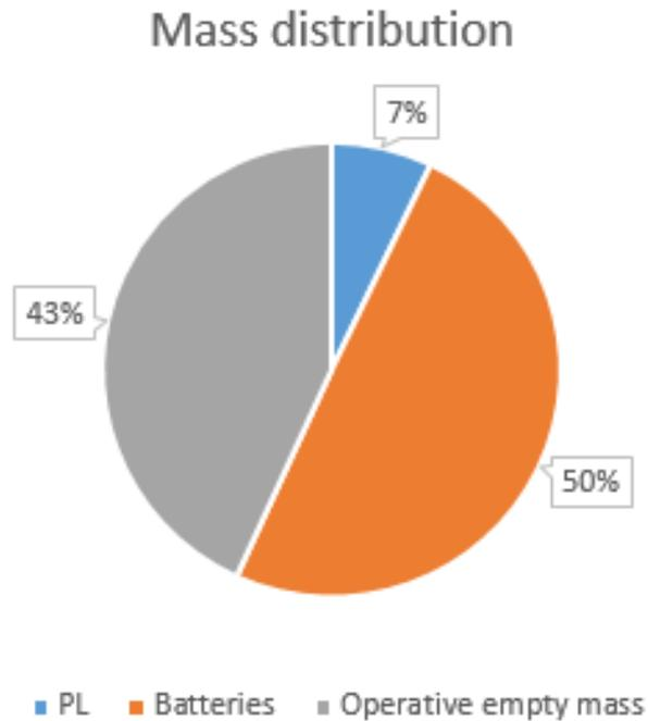
**Figure 6.1** Mass distribution, it is compelling the measly share of payload in the overall weight.
