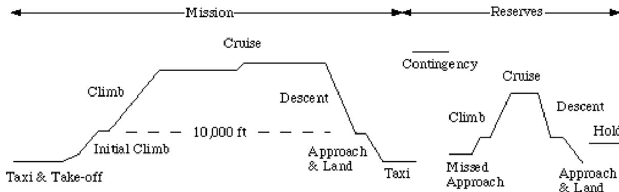
**Figure 4.1** Typical flight profile with its different flight phases.
