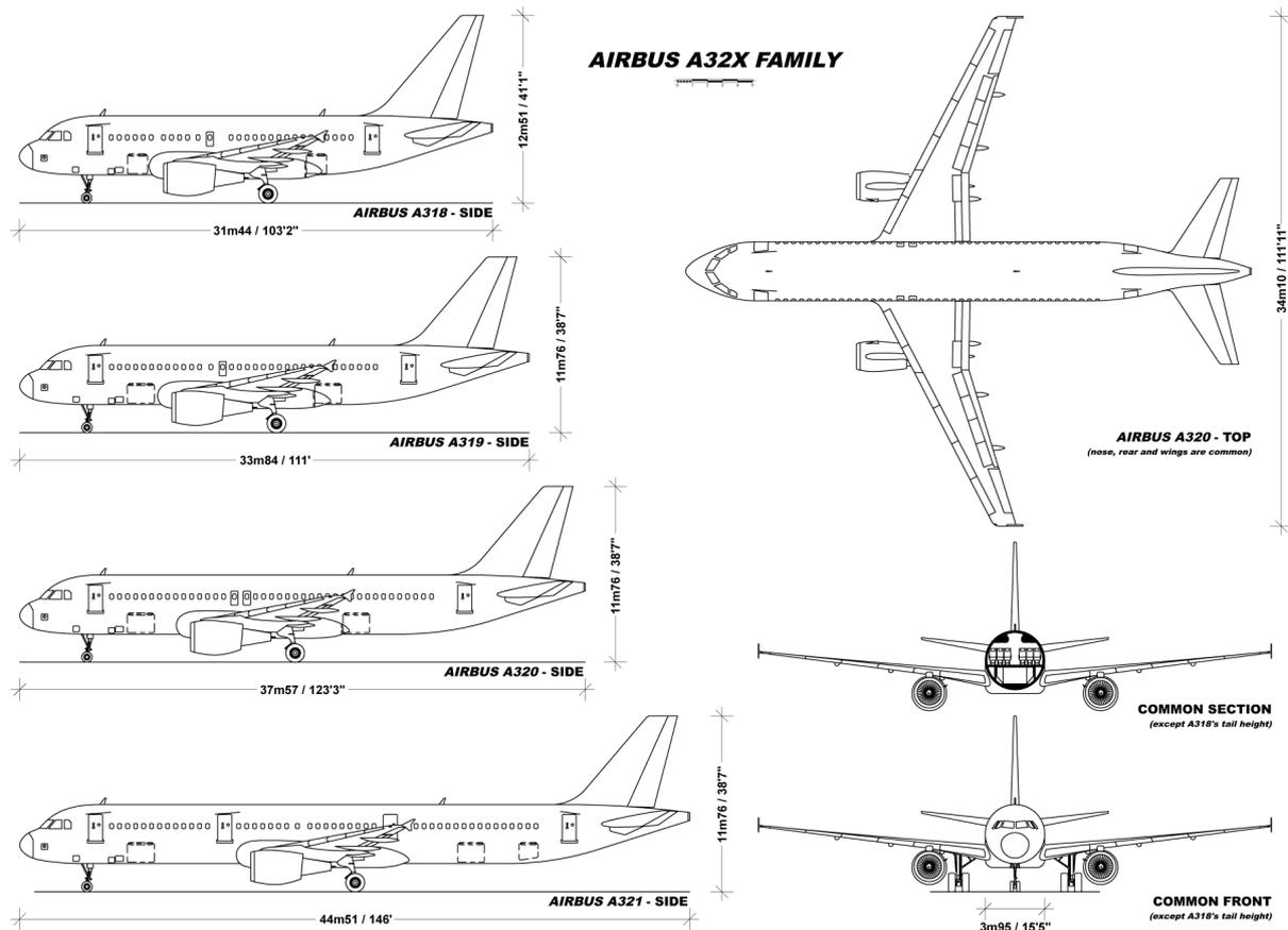
**Figure 5.1** Airplane lengthening in the A320 family. Image taken from (Scavini 2011a).
