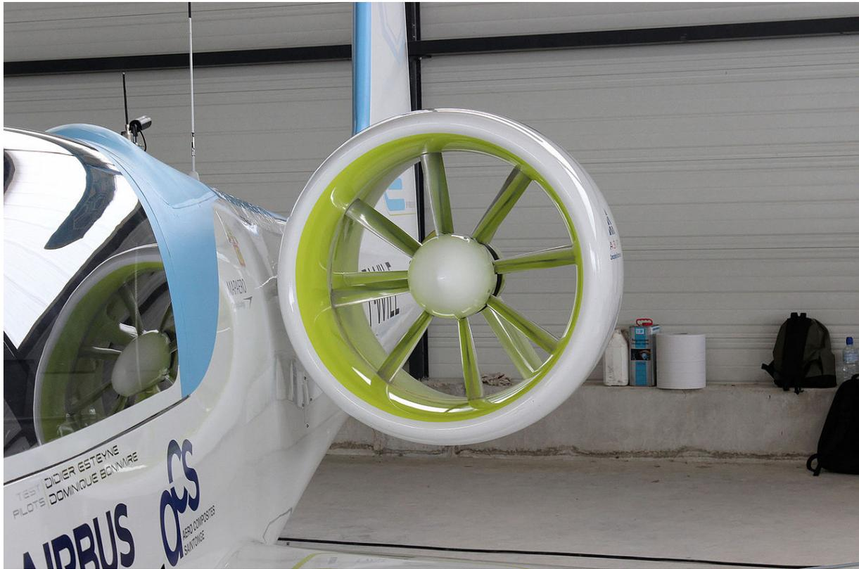
**Figure 2.6** Ducted fans will now be the providers of thrust. Image taken from **Varmin (2014)**.
