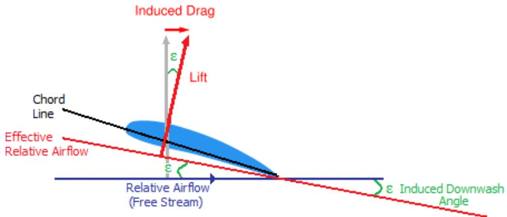
**Figure 8.4** Lift is projected against the airplane velocity, generating induced drag. Image taken from **Walton (2013)**
