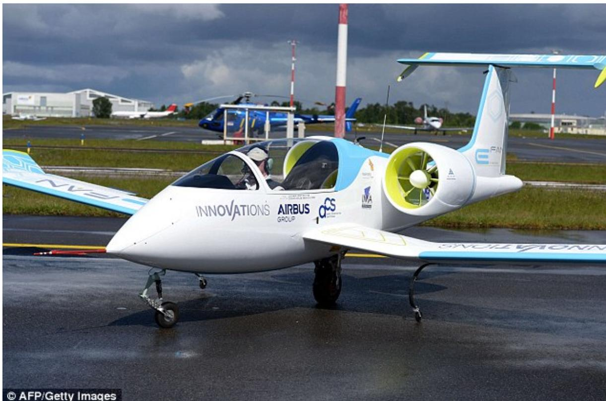
**Figure 1.3** The Airbus E-fan is a modern project of a battery powered airplane. It is only a prototype for now, but it is a first important step in this direction. Image taken from Griffiths (2014)
