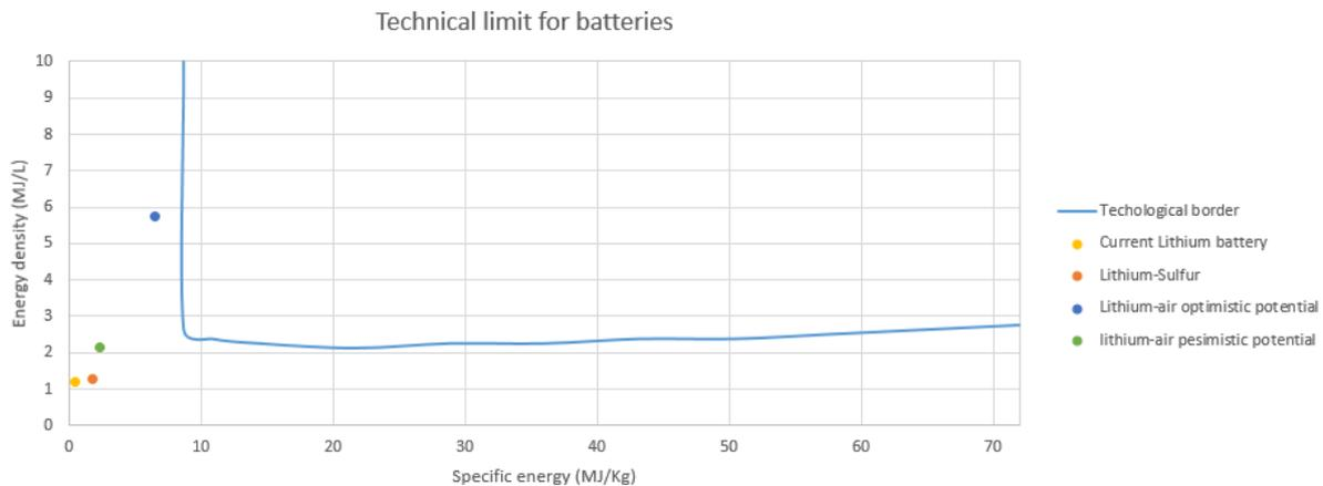
**Figure 6.7** Technological border and technological level of different batteries. All kinds of batteries are out of the possibilities area.
