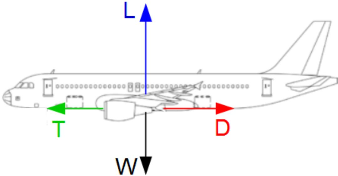
**Figure 3.2** Scheme of forces in an airplane flying in cruise mode, taken from **Scavini (2011b)** and modified.
