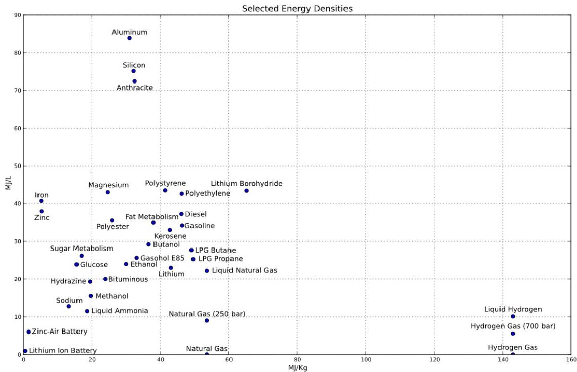
**Figure 2.2** Different energy densities and specific energy for different kinds of Energy storage systems, taken from **Dial (2008)**.
