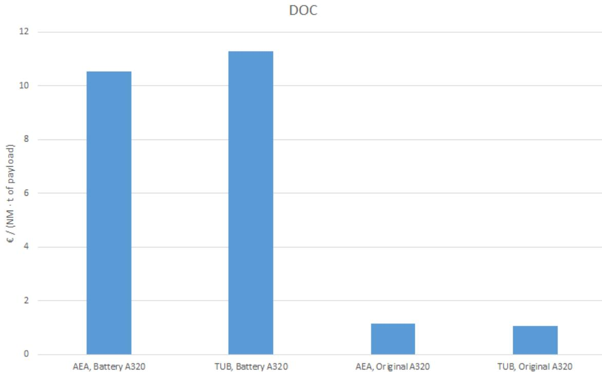
**Figure 6.5** Comparison of costs between the designed battery-powered A320 and the original one, using two different methods.
