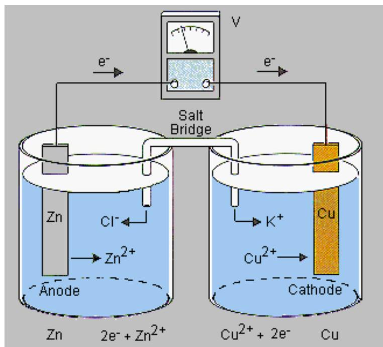
**Figure 8.1** Zn-Cu Battery scheme. Chemical reactions in both sides create a difference of electromagnetic potential, causing electricity to flow. Image taken from **KidsEnergy (2005)**
