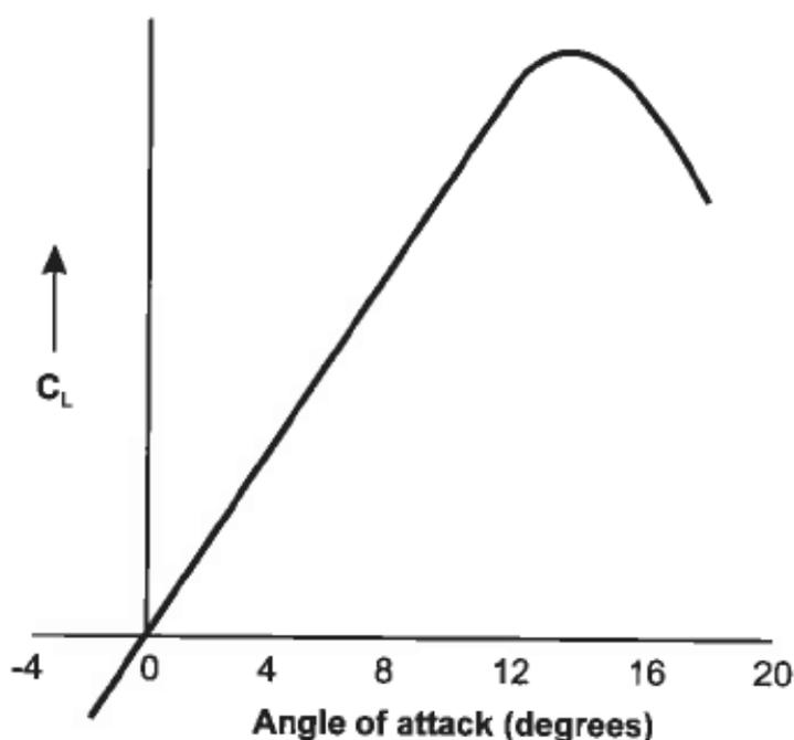
**Figure 8.2** Evolution of the lift coefficient with the angle of attack. Image taken from **Rotorhead8900 (2011)**
