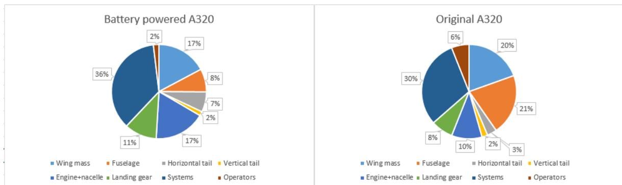
**Figure 6.2** Operative empty mass distribution, comparison between the original A320 and the Battery powered one.
