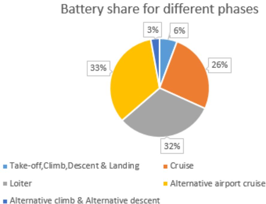
**Figure 6.3** Battery distribution for different flight phases and safety requirements.
