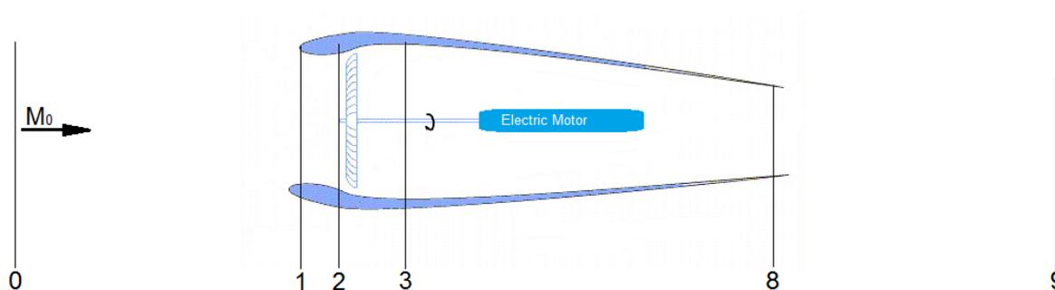
**Figure 3.1** Different sections of a ducted fan, taken from **Thomas (2001)** and modified. The notation is taken from the traditional Engine Design criteria.
