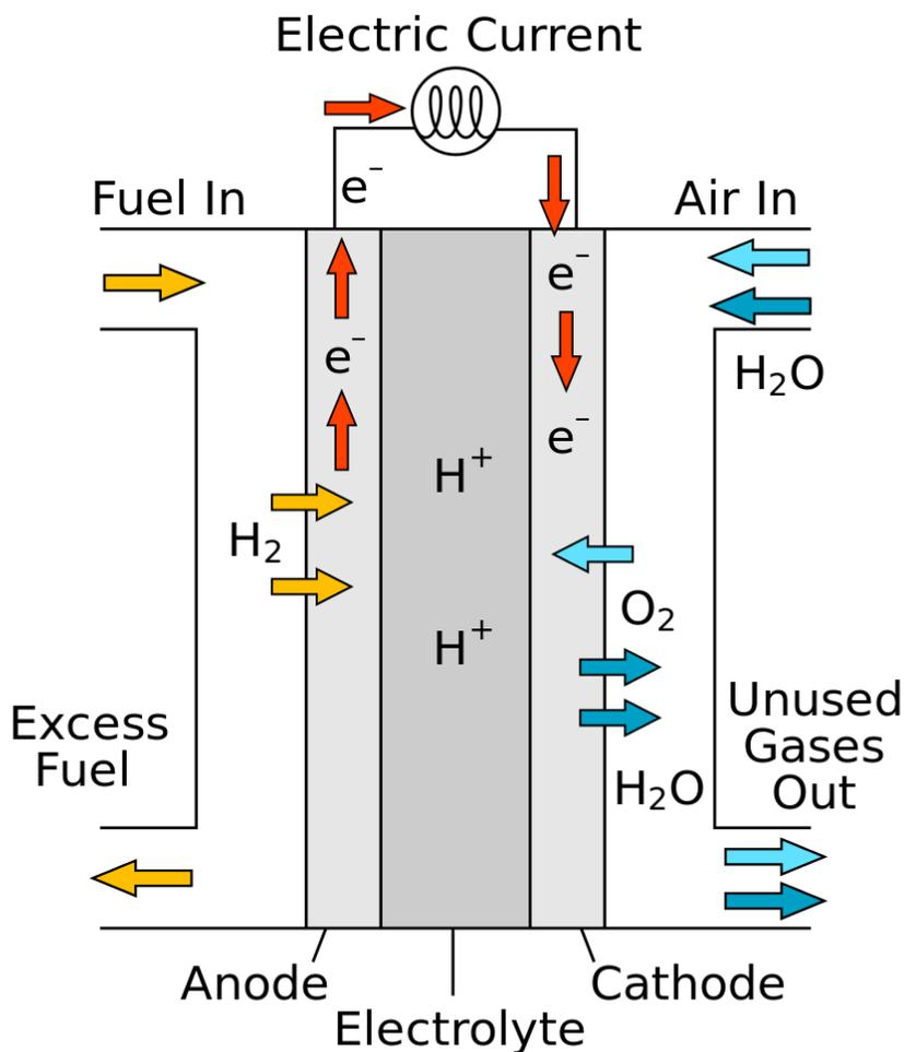
**Figure 2.3** Scheme of a fuel cell taken from **Dervisoglu (2012)**.
