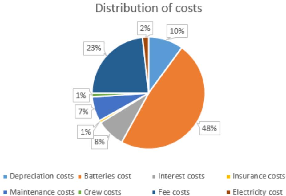
**Figure 6.6** Distribution of costs in the battery powered A320.
