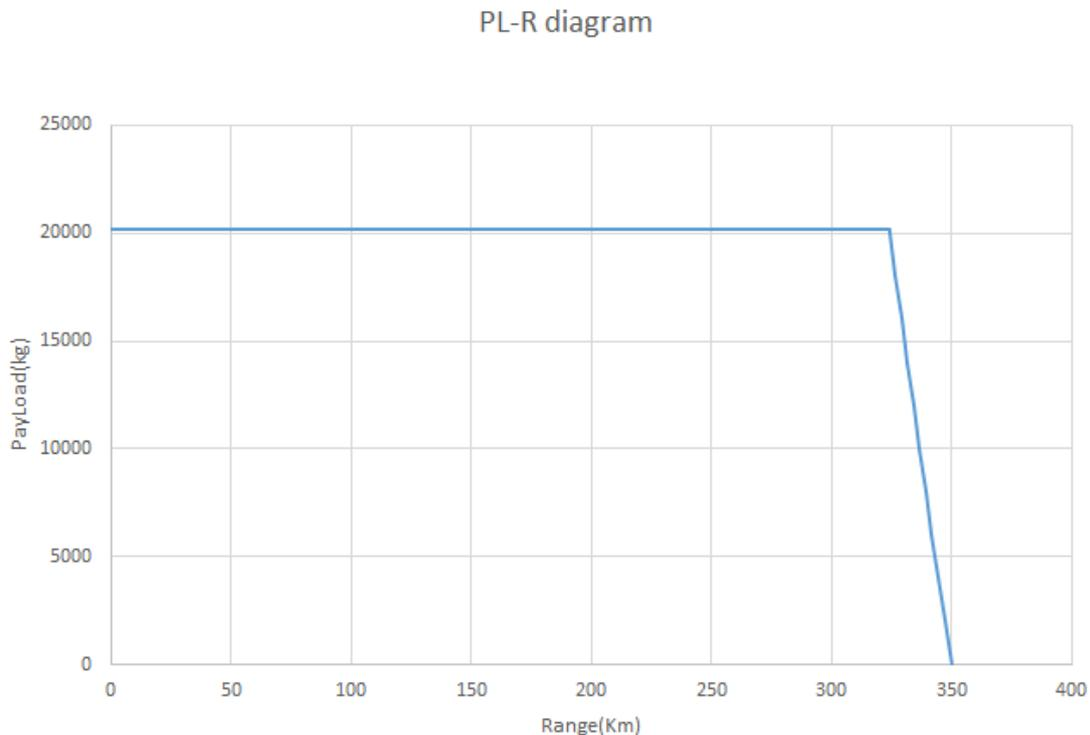
**Figure 6.4** Payload range diagram for the designed battery powered airplane
