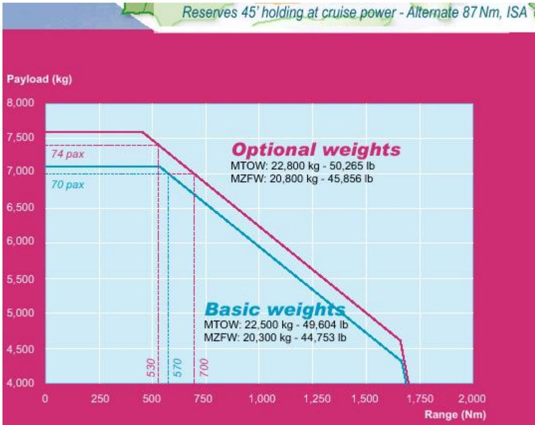
**Fig. 2.2** Payload-range diagram for the ATR 72-500 (ATR 2008)
