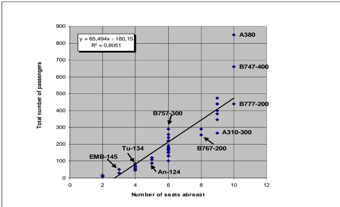
**Figure 3.1** Number of seats abreast versus Total number of passengers
