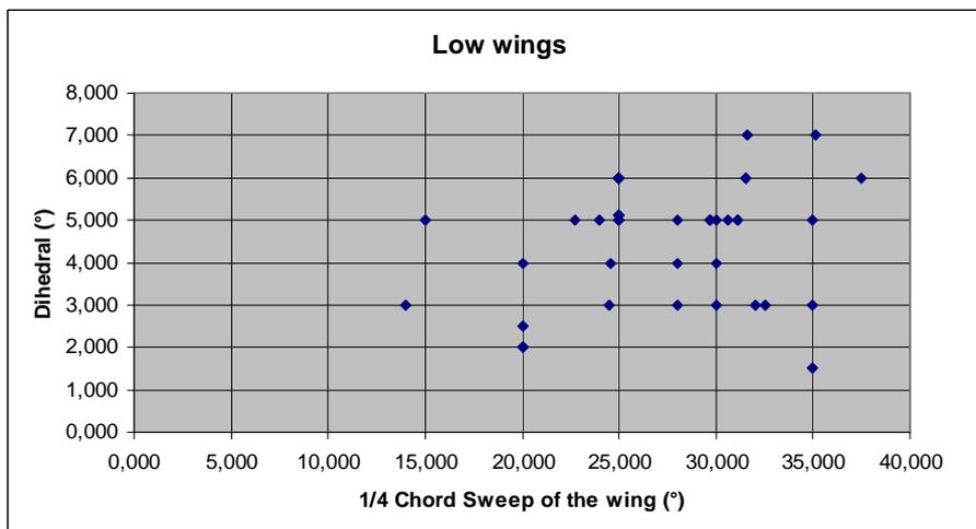
**Figure 3.14** ¼ Chord sweep of the wing versus Dihedral for Low wings
