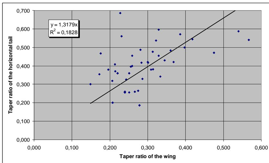
**Figure 3.21** Taper ratio of the wing versus Taper ratio of the horizontal tail
