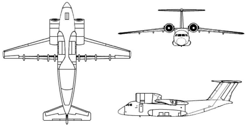
Figure A.51 Three-view drawing: An-72
