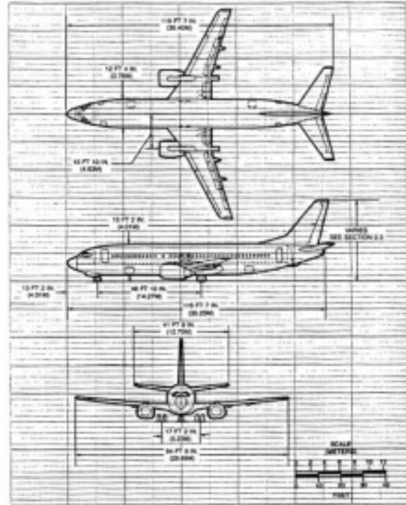
Figure A.16 Three-view drawing: B737-400
