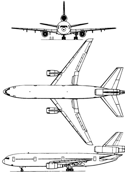
Figure A.28 Three-view drawing: DC10-10
