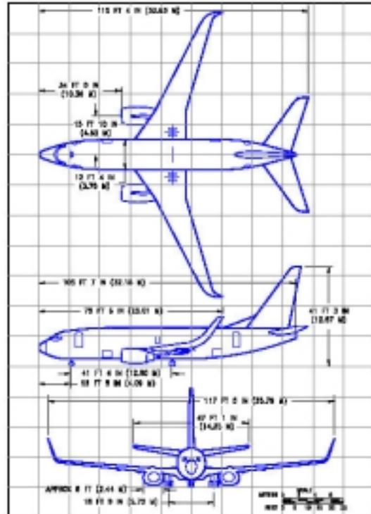
Figure A.18 Three-view drawing: B737-700
