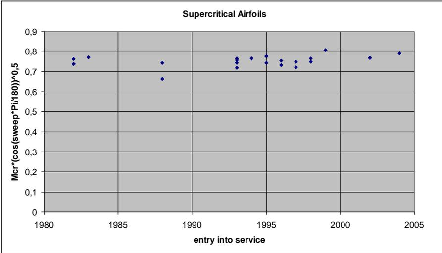
**Figure 3.10** Entry into service versus  $M_{eff}$  for Supercritical Airfoils
