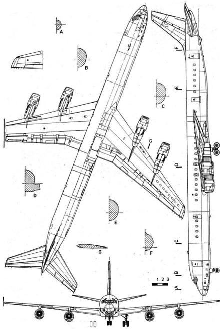
Figure A.27 Three-view drawing: DC8-63
