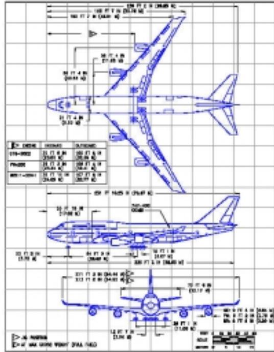
Figure A.20 Three-view drawing: B747-400
