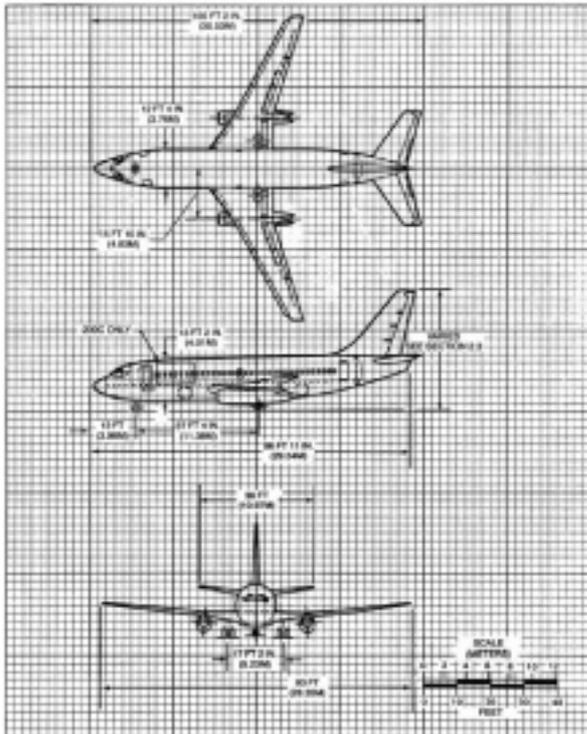
Figure A.15 Three-view drawing: B737-200
