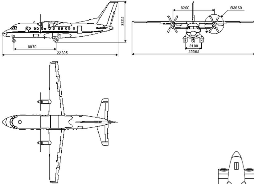
Figure A.50 Three-view drawing: An-140
