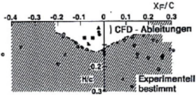
Figure 2.8 Engine locations with CFD Method (Airbus 1991)
