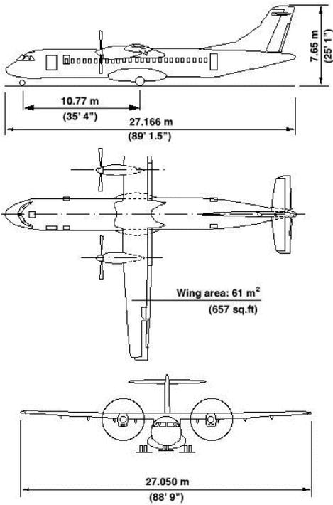
Figure A.52 Three-view drawing: ATR 72
