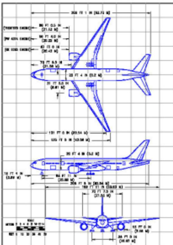
Figure A.25 Three-view drawing: B777-200
