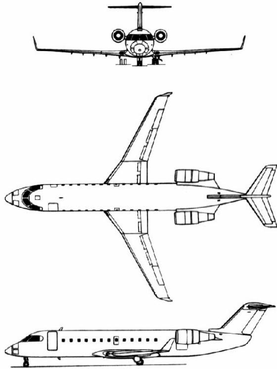
Figure A.47 Three-view drawing: CRJ 200
