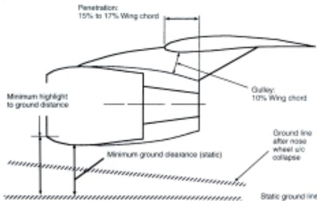
Figure 2.10 Ground clearance considerations for under-wing installation (Jenkinson 1999)
