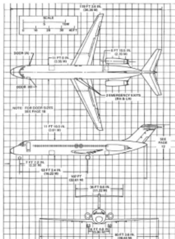
Figure A.26 Three-view drawing: DC9-30
