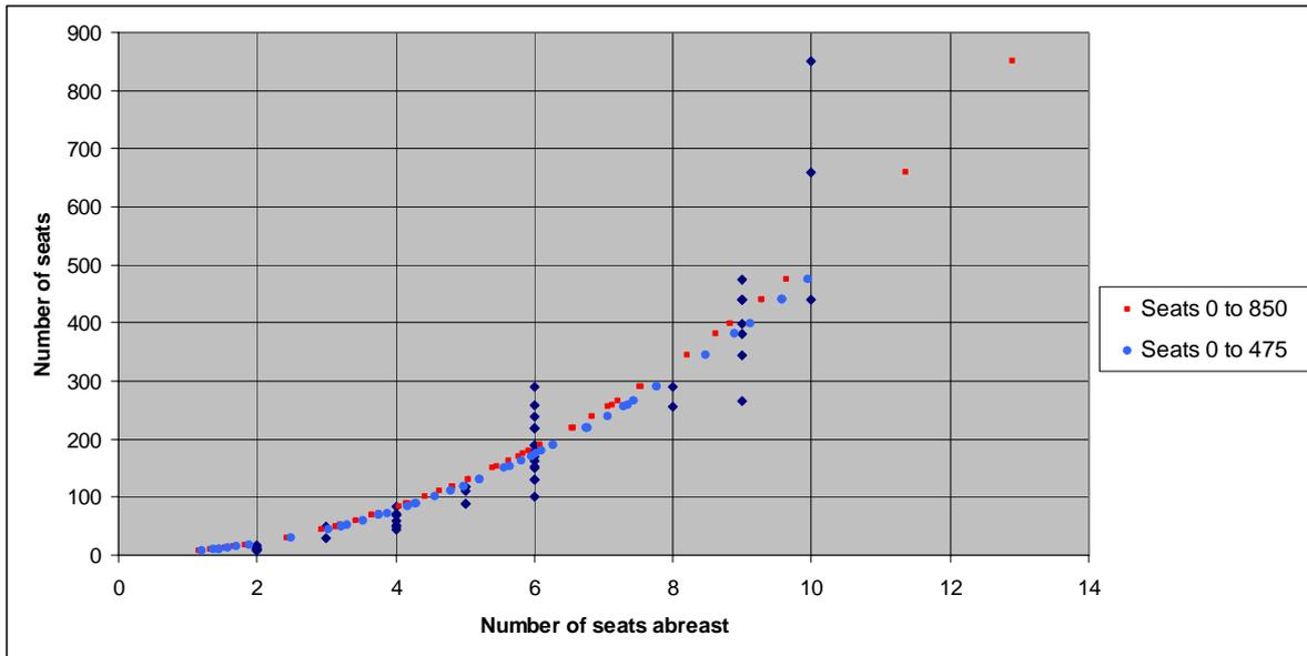
**Figure 3.3** Number of seats abreast versus Total number of seats with optimized series
