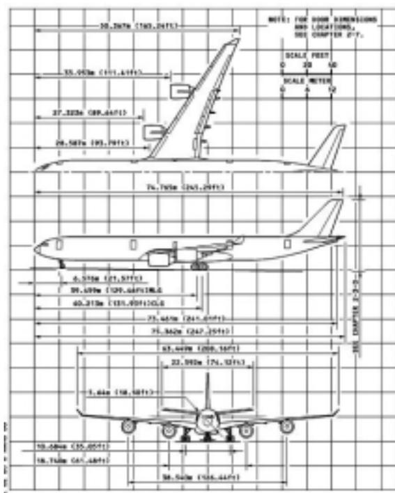
Figure A.10 Three-view drawing: A340-600
