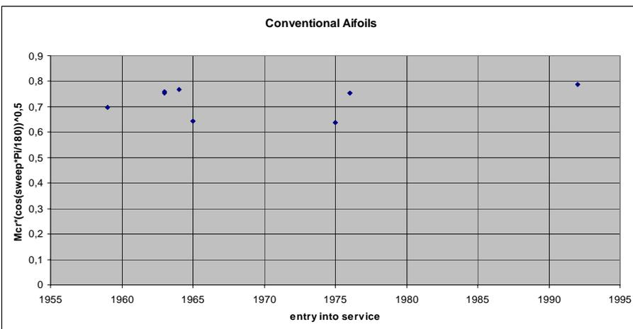
**Figure 3.12** Entry into service versus  $M_{eff}$  for Conventional Airfoils
