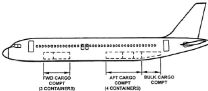
**Figure 2.5** A320, lower deck compartments (**Airbus SAS 2003**)
