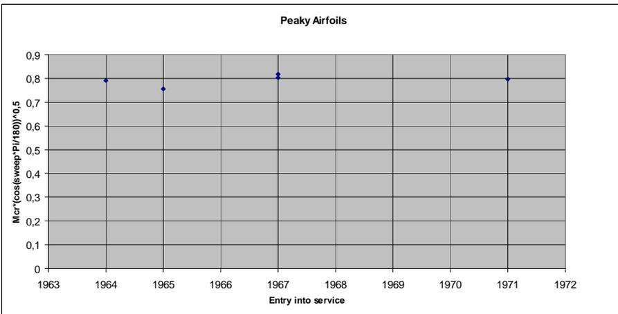
**Figure 3.11** Entry into service versus  $M_{eff}$  for Peaky Airfoils
