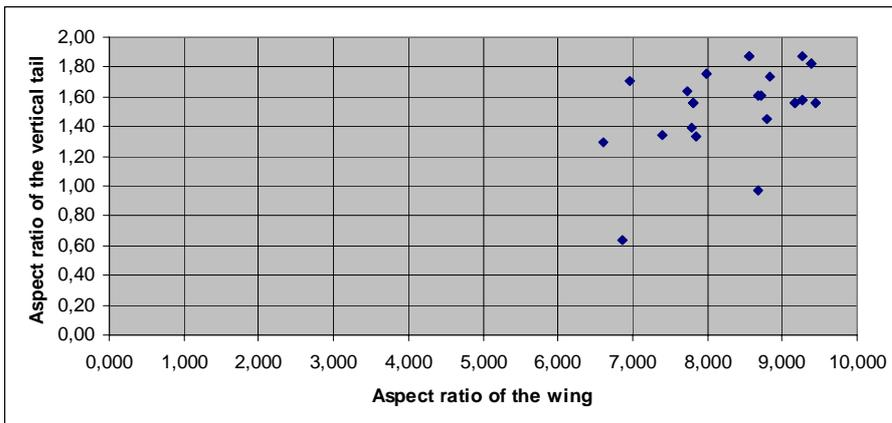
**Figure 3.20** Aspect ratio of the wing versus aspect ratio of the vertical tail
