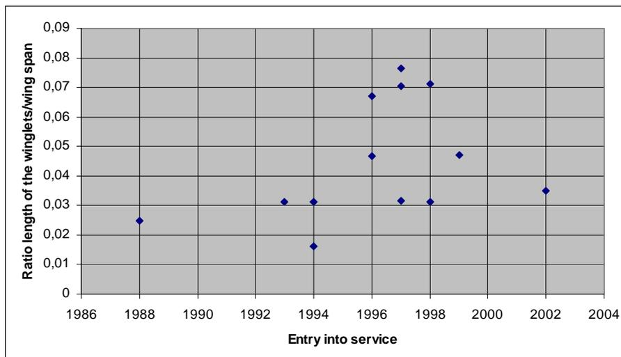
**Figure 3.16** Entry into service versus Ratio length of winglets/wing span for single winglets
