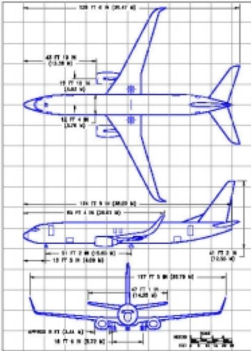
Figure A.19 Three-view drawing: B737-800
