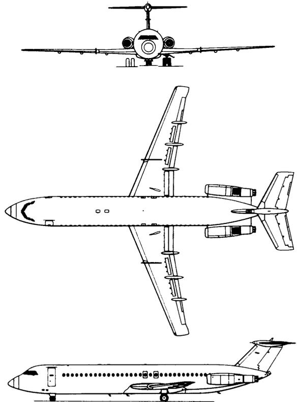
**Figure A.39** Three-view drawing: BAC1-11
