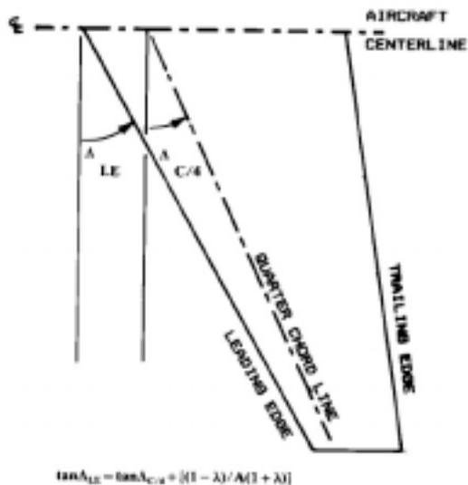
Figure 1.1 Sweep angle of the wing (Raymer 1992, p. 48)
