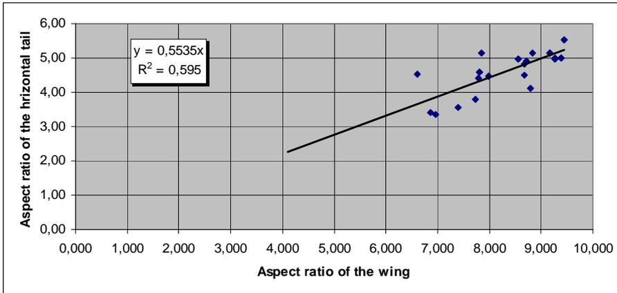
**Figure 3.19** Aspect ratio of the wing versus aspect ratio of the horizontal tail
