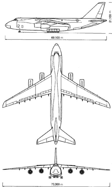
Figure A.49 Three-view drawing: An-124
