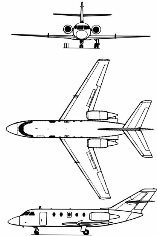
**Figure A.38** Three-view drawing: Falcon 20
