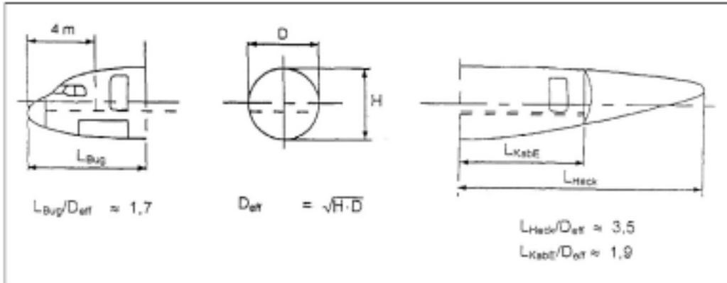
**Figure 2.4** Length of cockpit, nose section, cabin in the tail section and tail section functions of fuselage diameter (**Schmitt 98**)
