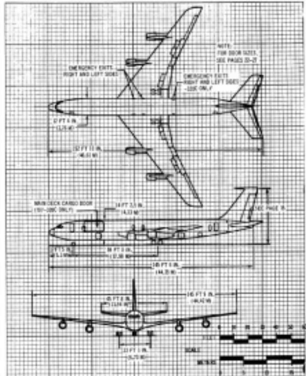
Figure A.12 Three-view drawing: B707-320C
