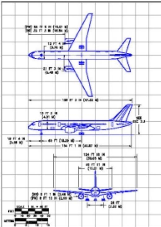
Figure A.21 Three-view drawing: B757-200
