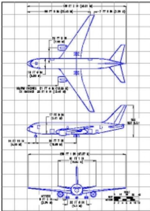
Figure A.23 Three-view drawing: B767-200
