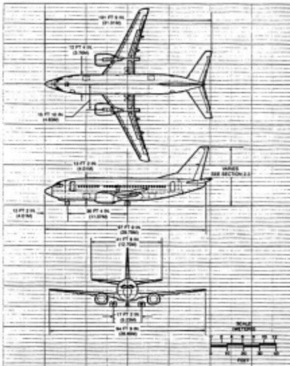
Figure A.17 Three-view drawing: B737-500
