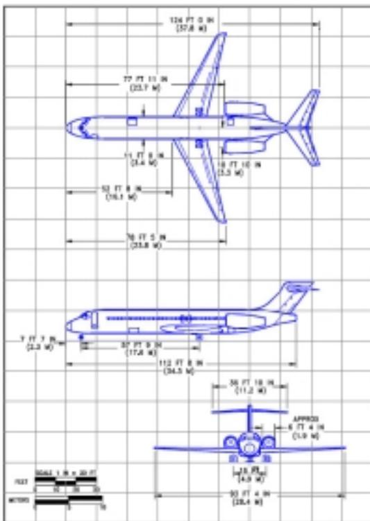
Figure A.13 Three-view drawing: B717-200
