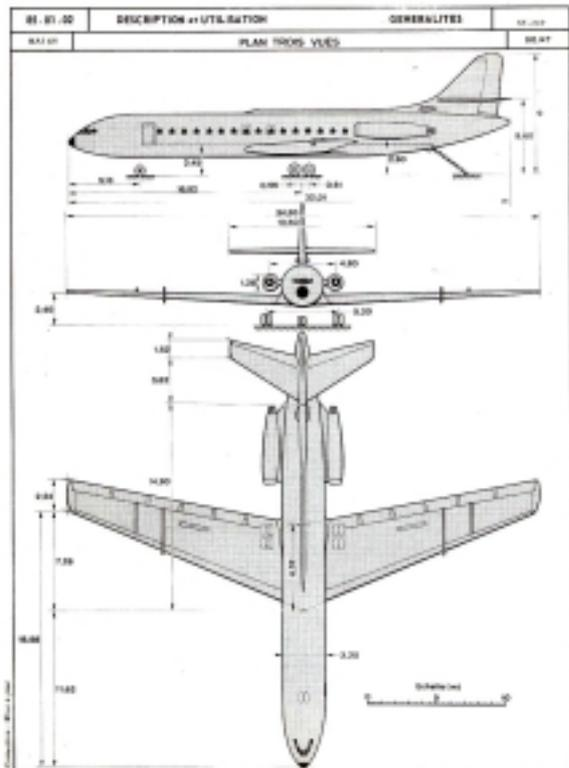
Figure A.33 Three-view drawing: Caravelle
