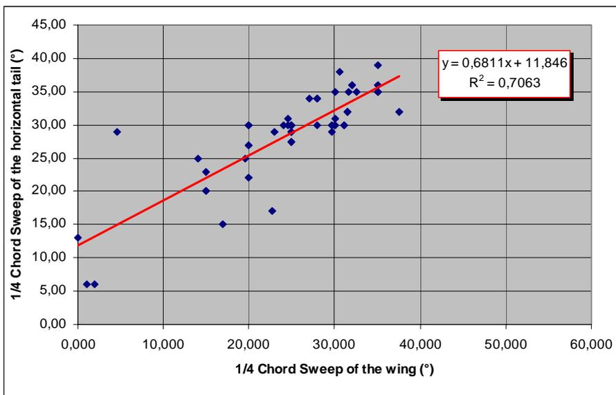
**Figure 3.17** 1/4 Chord sweep of the wing versus 1/4 Chord sweep of the horizontal tail
