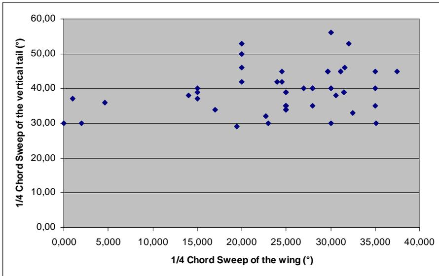
**Figure 3.18** 1/4 Chord sweep of the wing versus 1/4 Chord sweep of the vertical tail
