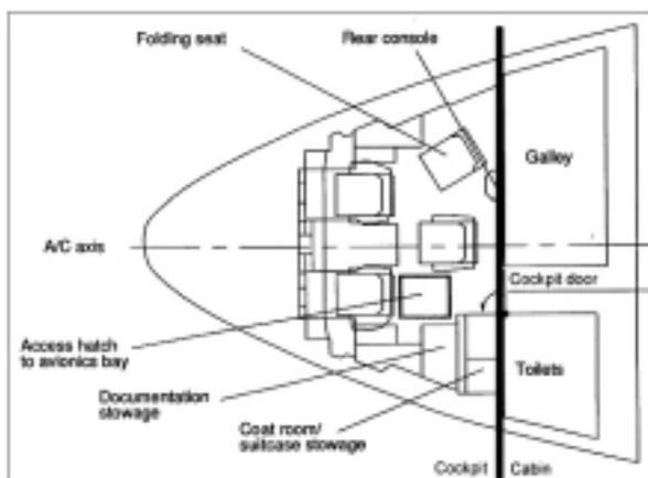
**Figure 2.3** Cockpit of Airbus A340 (Airbus Industries)
