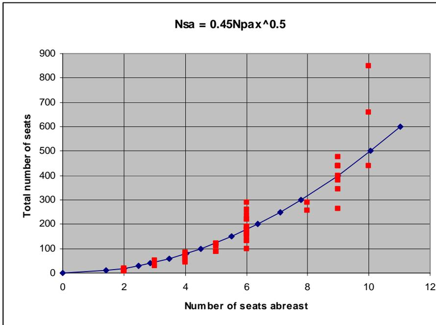
**Figure 3.2** Superposition of figure 2.2 and gathered data
