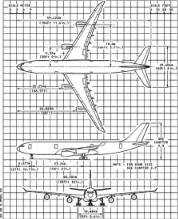
Figure A.8 Three-view drawing: A340-200
