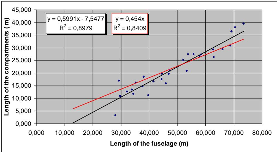
**Figure 3.5** Length of the fuselage versus length of the cargo compartments
