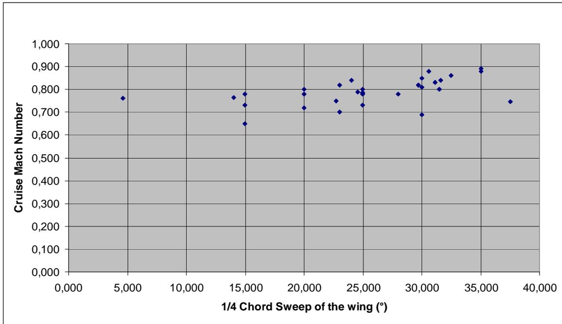
**Figure 3.9** ¼ Chord sweep of the wing versus Cruise Mach number
