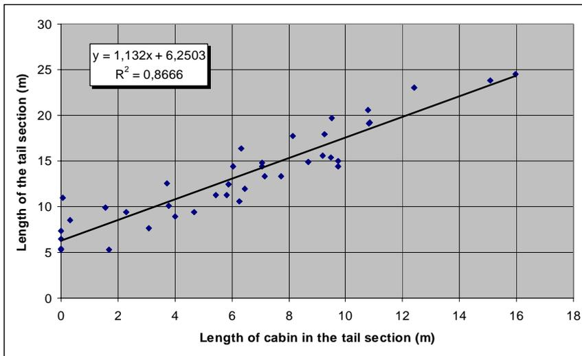
**Figure 3.4** Length of cabin in the tail section versus length of the tail section
