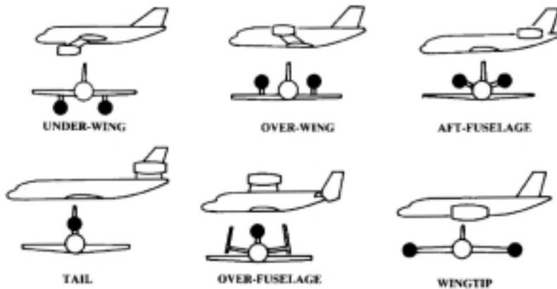
**Figure 2.6** Inlet locations-podded engines (Raymer 1992)
