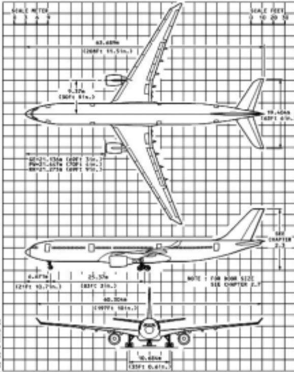
Figure A.7 Three-view drawing: A330-300
