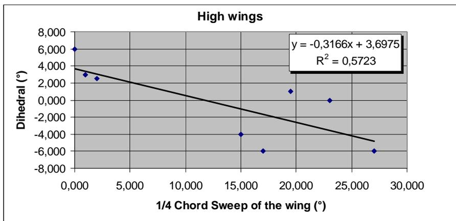
**Figure 3.13** ¼ Chord sweep of the wing versus Dihedral for High wings
