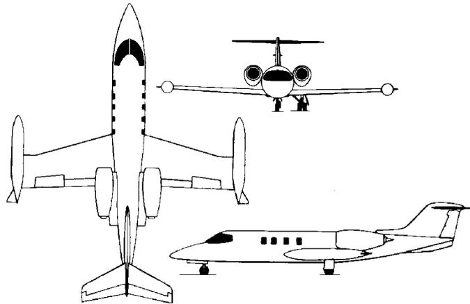
Figure A.36 Three-view drawing: Jetstar II
