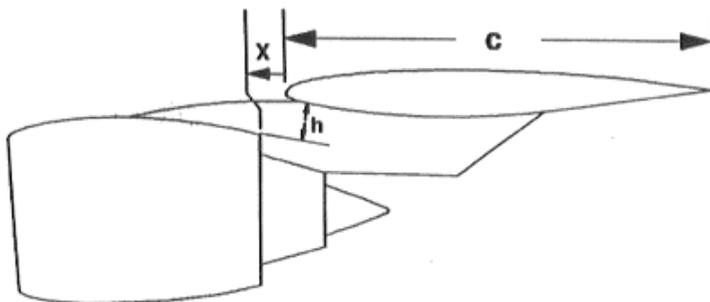
**Figure 2.7** Location of the nacelle compared to the wing (Kroo 2005)
