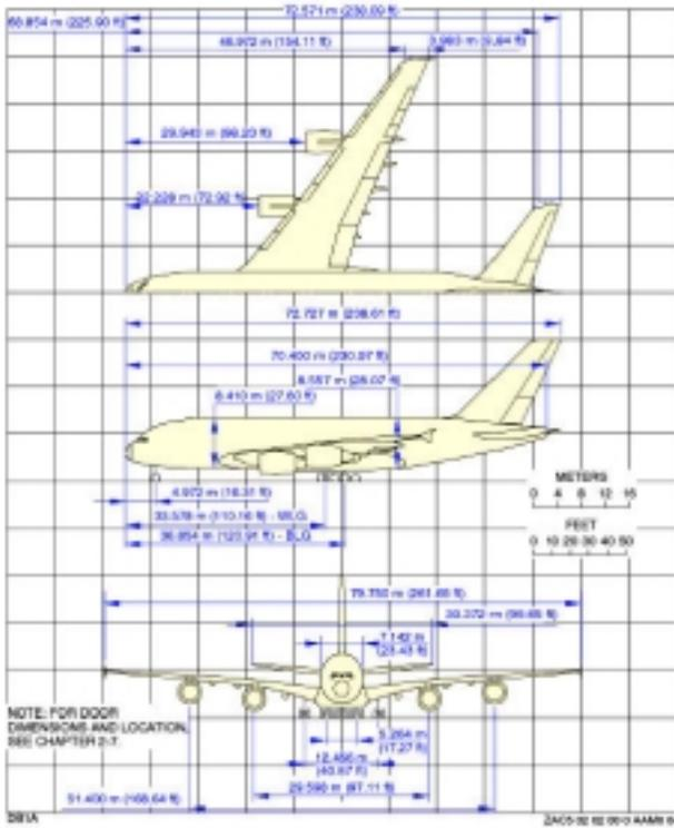
Figure A.11 Three-view drawing: A380-800
