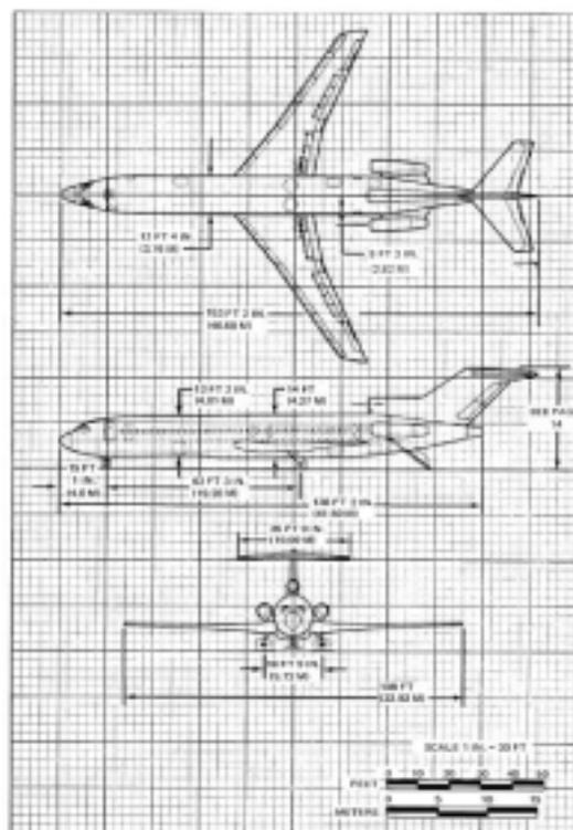
Figure A.14 Three-view drawing: B727-200
