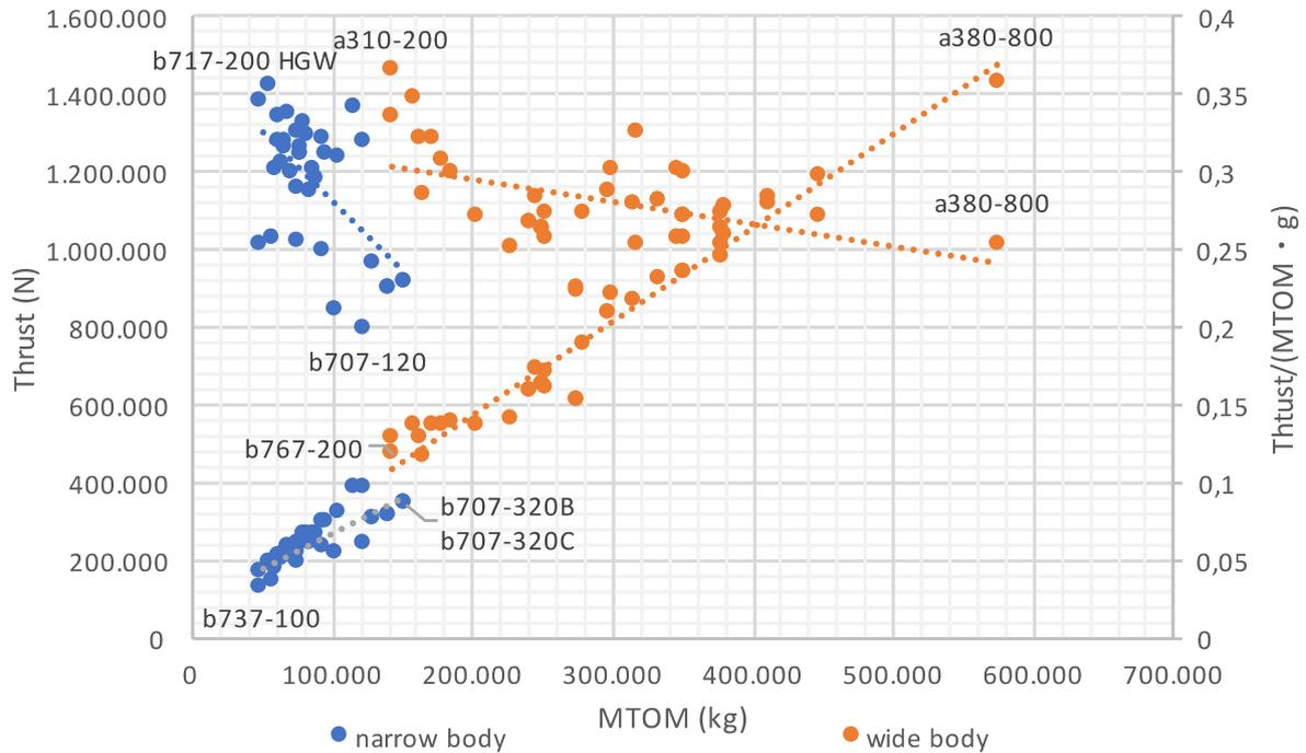
**Figure 6.9** T versus  $m_{MTO}$  (MTOM) and  $T/(m_{MTO} \cdot g) = T/W$  ( $T/(MTOM \cdot g)$ ) lines.
