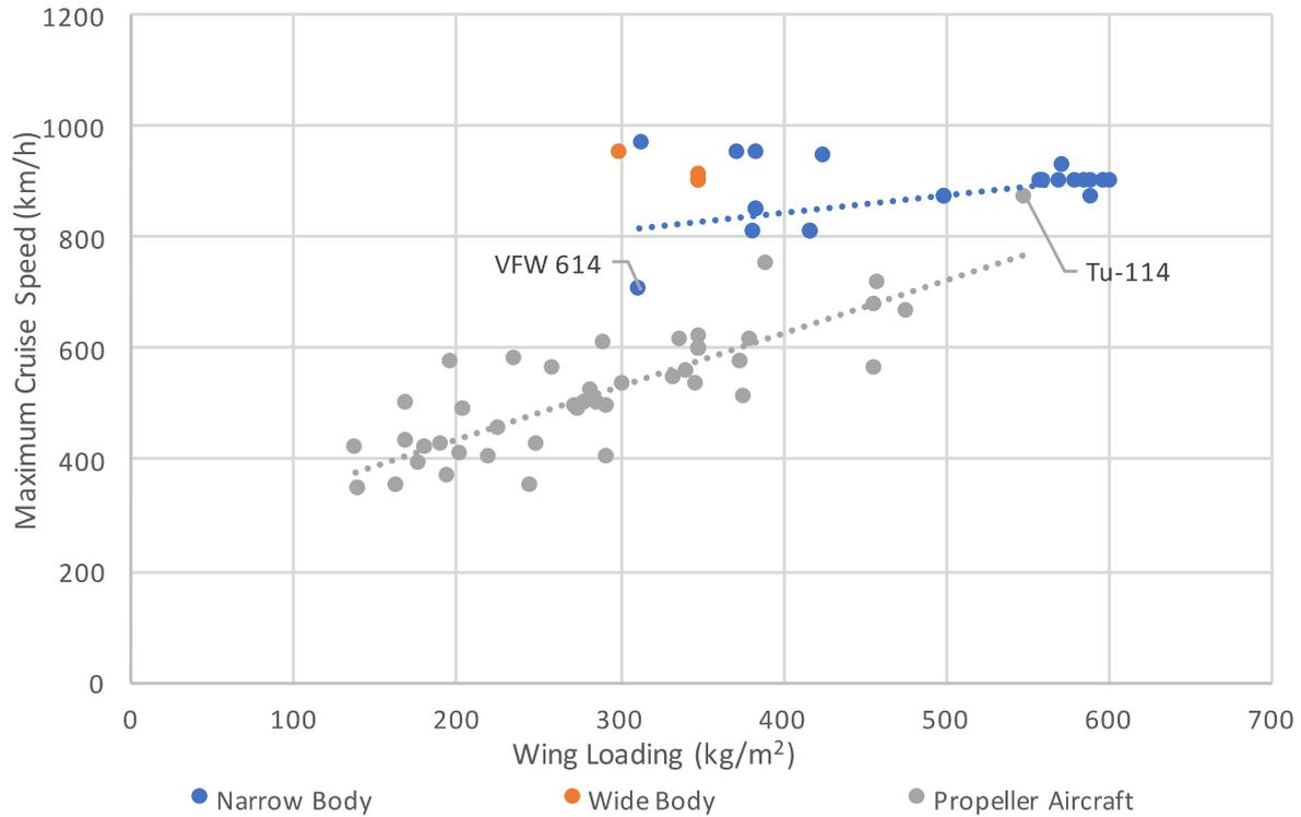
**Figure 5.10** Maximum Cruise Speed and Wing Loading.
