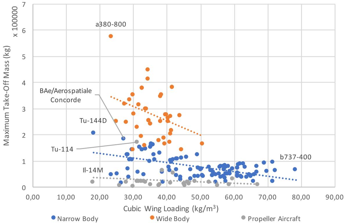
**Figure 5.1** Maximum Take-Off Mass and Cubic Wing Loading.
