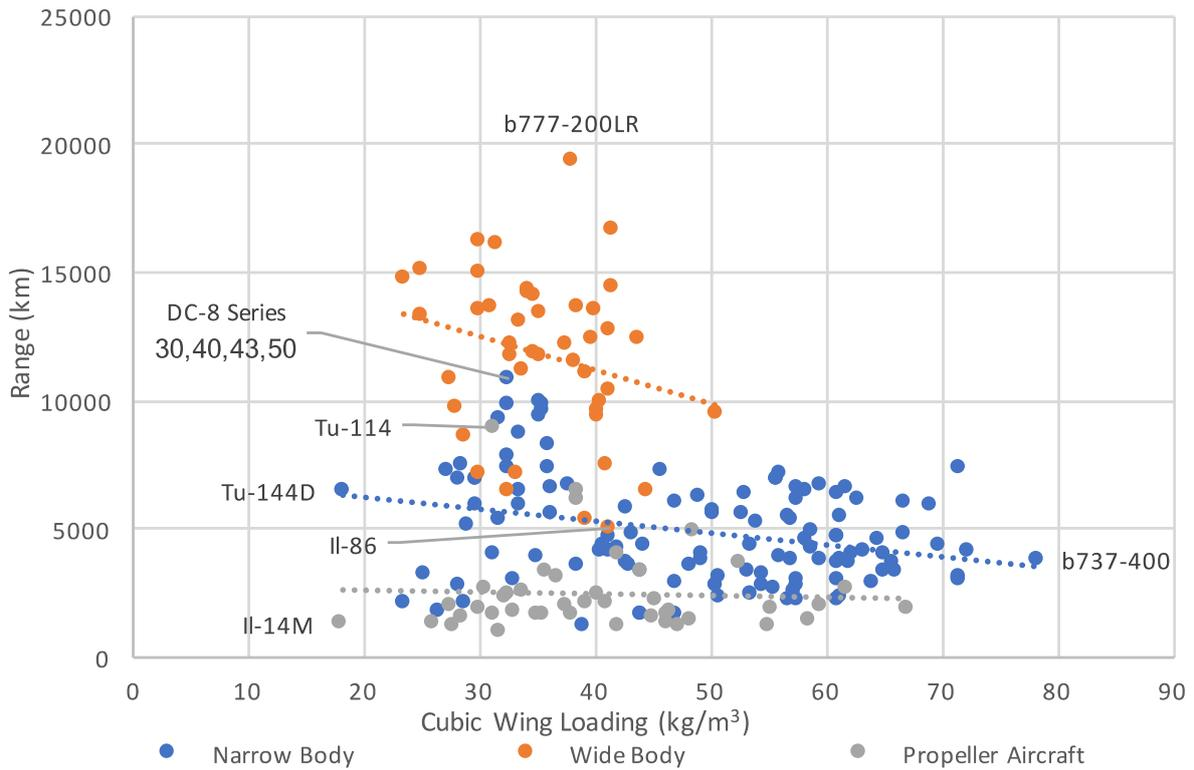
**Figure 5.11** Range and Cubic Wing Loading.
