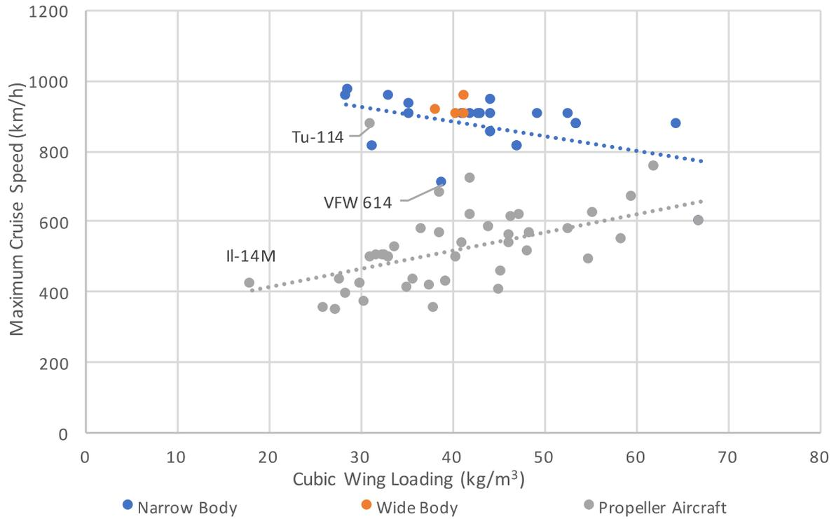
**Figure 5.9** Maximum Cruise Speed and Cubic Wing Loading.
