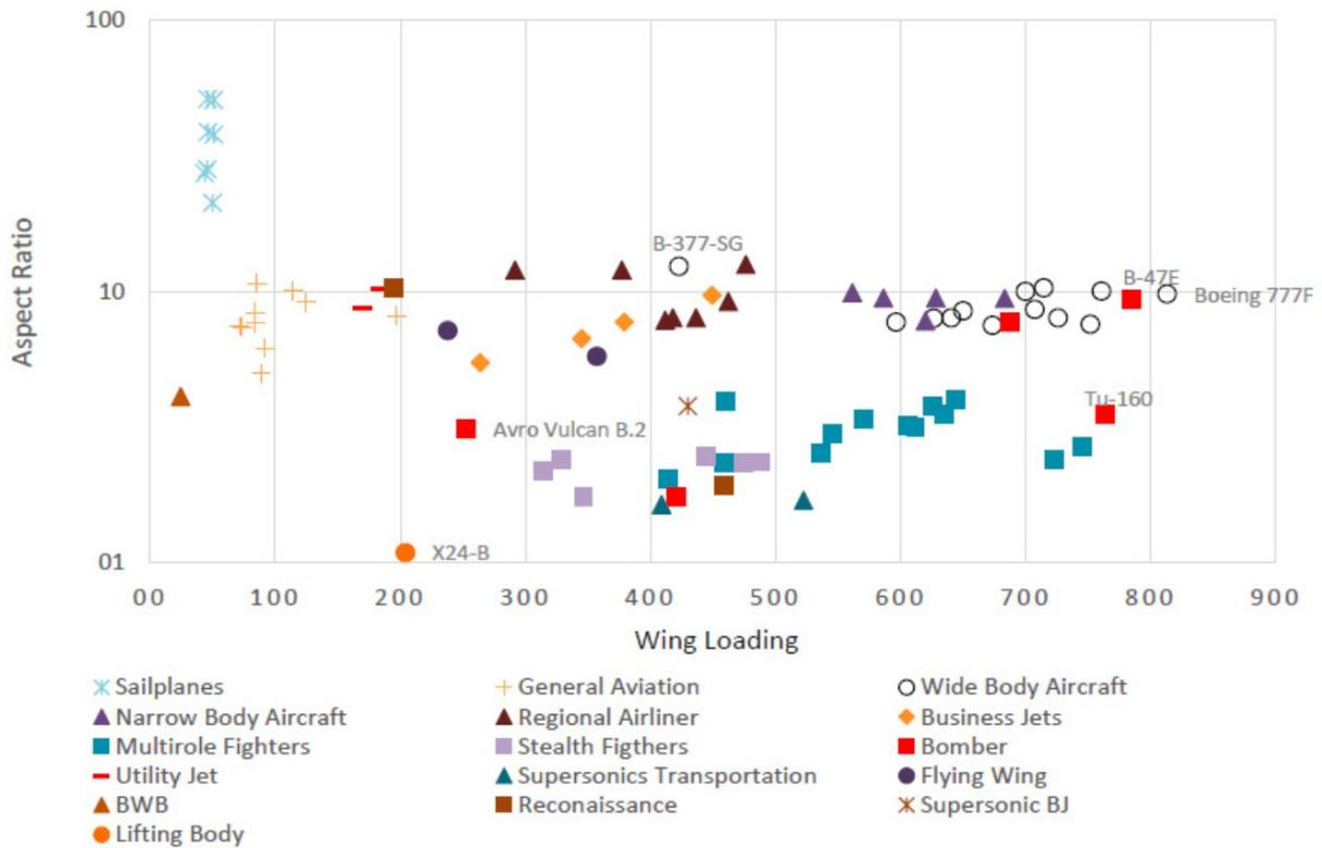
**Figure 2.7** Aspect ratio and wing loading chart of 81 aircraft. A base 10 log. Scale for AR was used for the readability of the scatter plot. (Durmus 2020)
