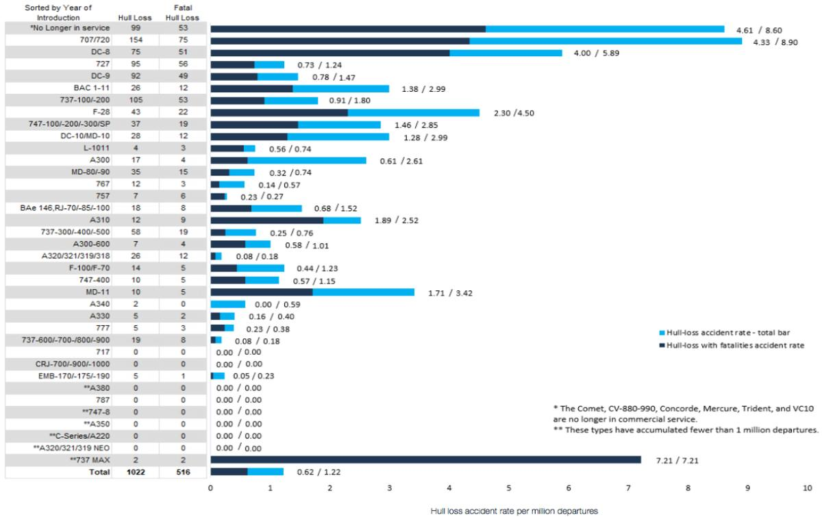
Figure 6.4 Hull-loss accident rates by airplane type (Boeing 2020).
