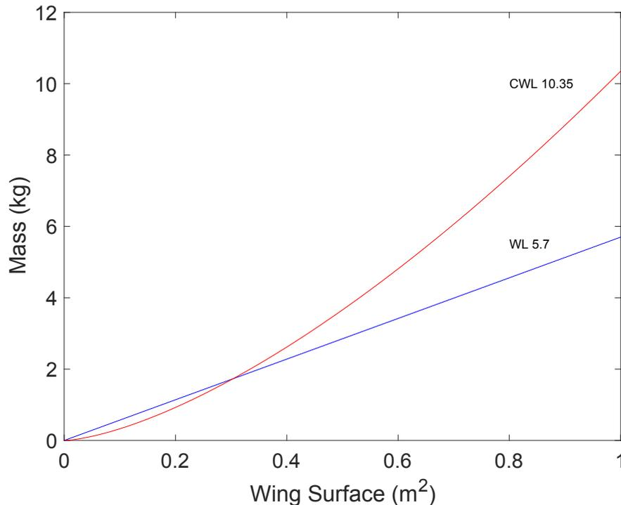
**Figure 2.2** CWL and WL lines for basic model.
