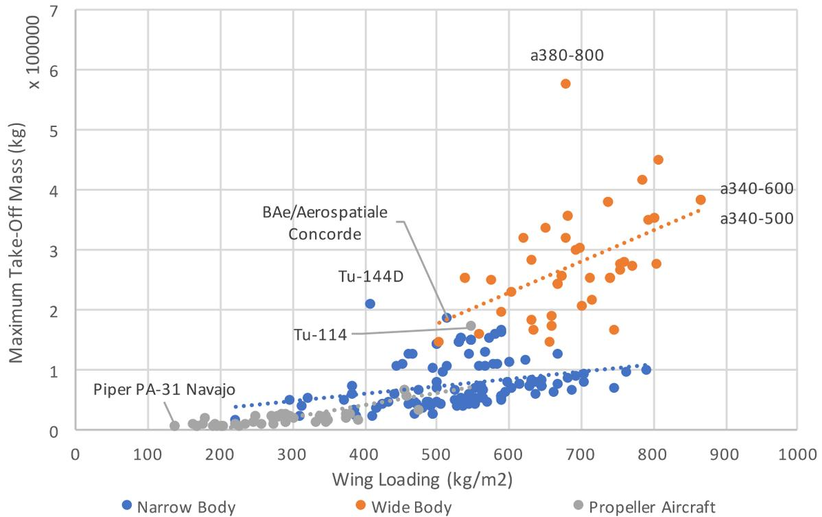
**Figure 5.2** Maximum Take-Off Mass and Wing Loading.
