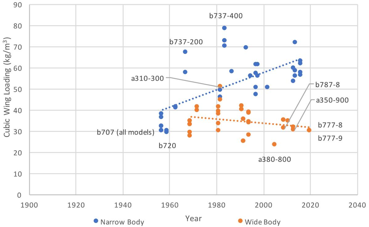
**Figure 5.13** Cubic Wing Loading through Years.
