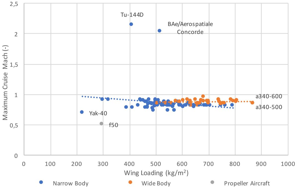
**Figure 5.8** Maximum Cruise Mach and Wing Loading.
