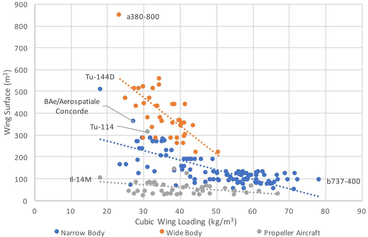
**Figure 5.3** Wing Surface and Cubic Wing Loading.
