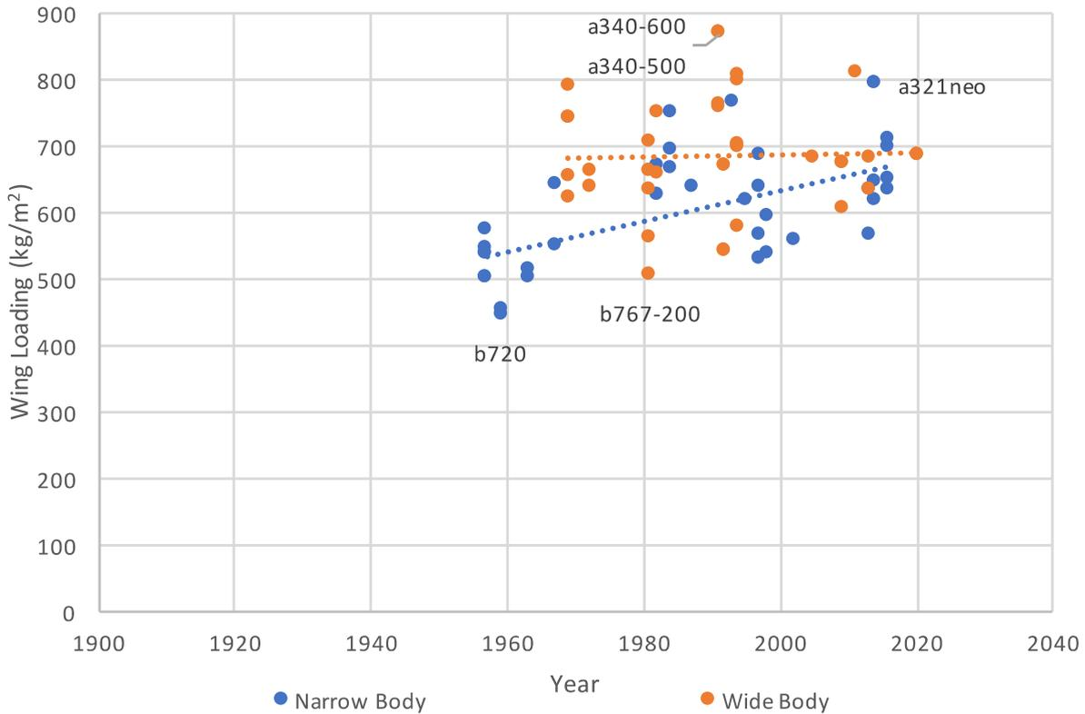
**Figure 5.14** Wing Loading through Years.
