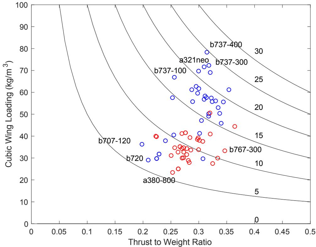
**Figure 6.3** Performance Factor for Airbus and Boeing's models.
