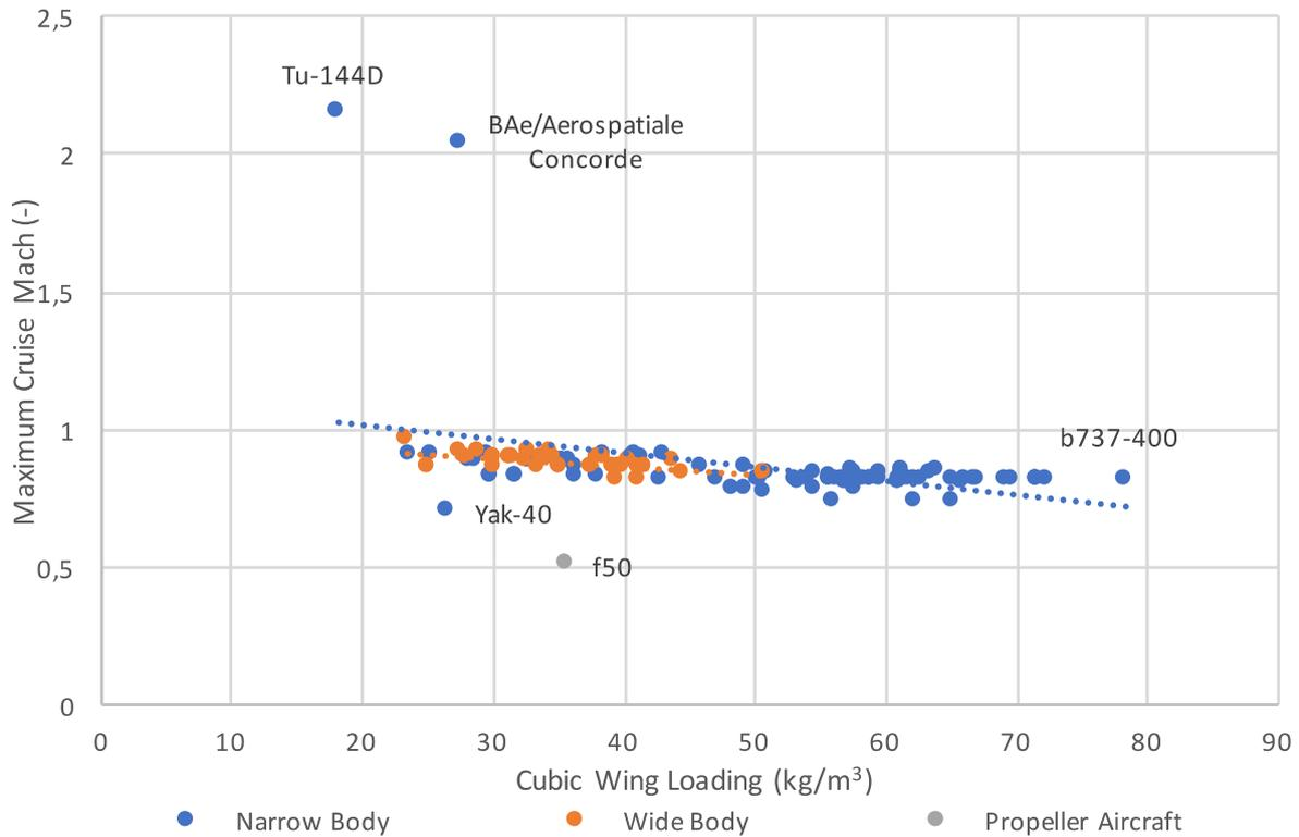
**Figure 5.7** Maximum Cruise Mach and Cubic Wing Loading.
