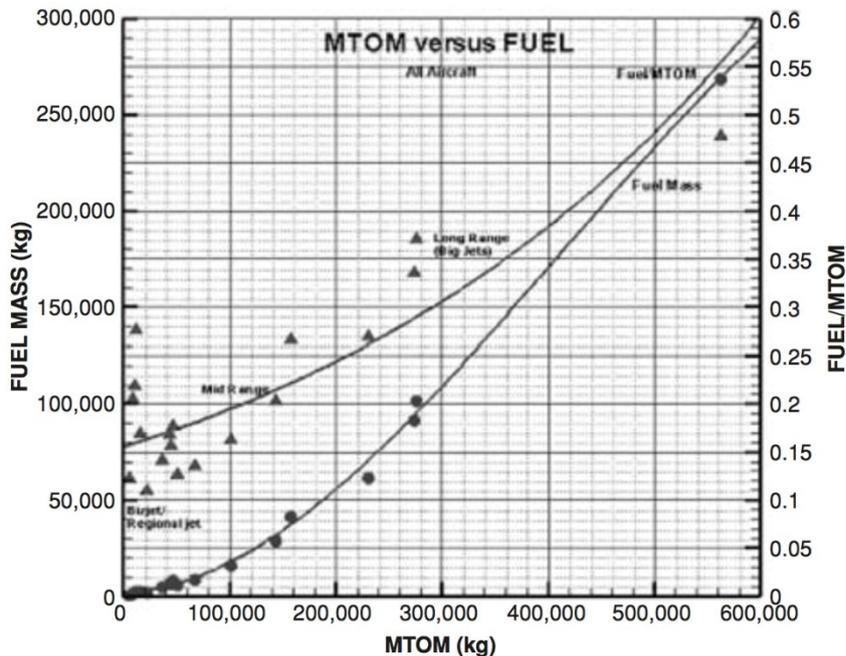
**Figure 6.8** Fuel load versus  $m_{MTO}$  (MTOM) and  $m_F/m_{MTO}$  ( $M_F/MTOM$ ) lines (Kundu 2010).
