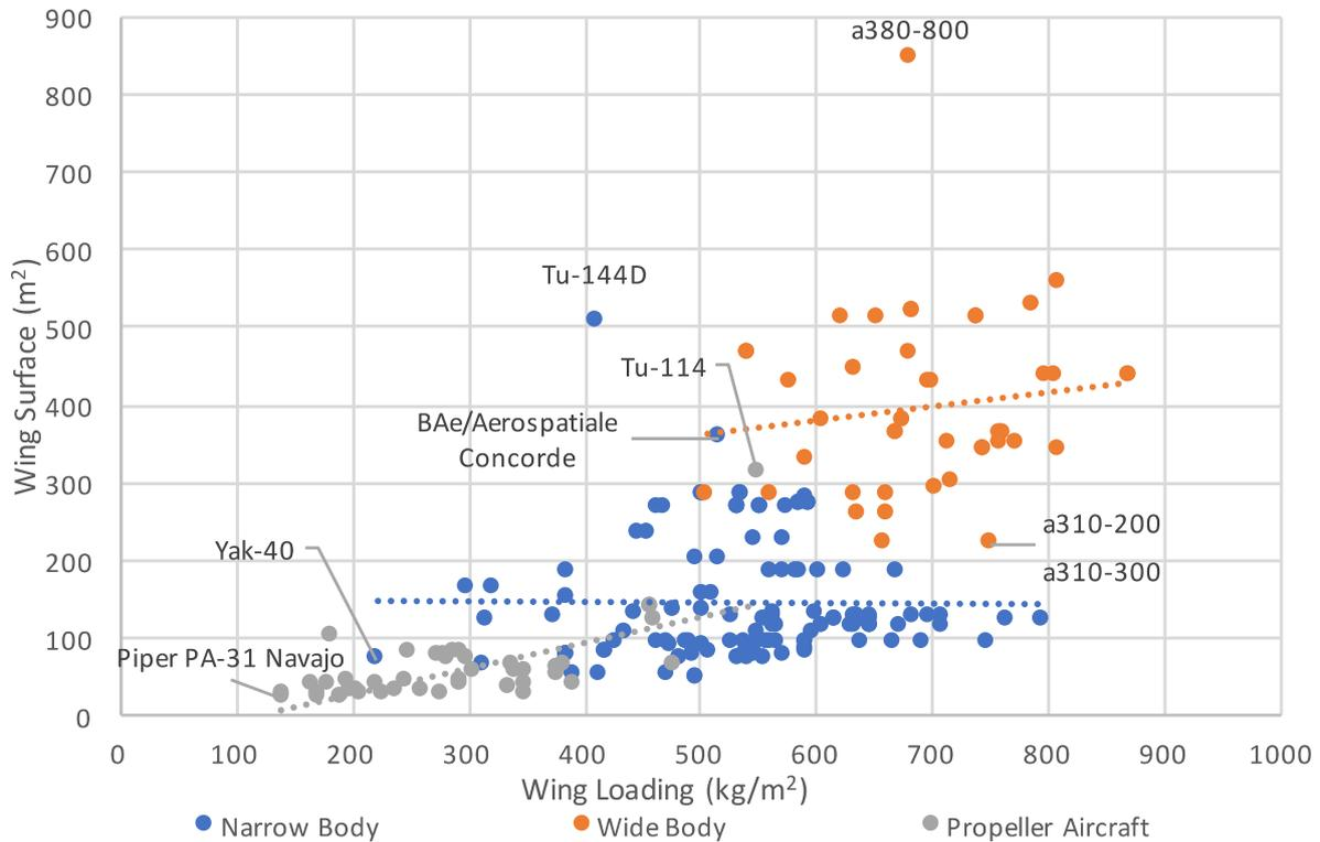
**Figure 5.4** Wing Surface and Wing Loading.
