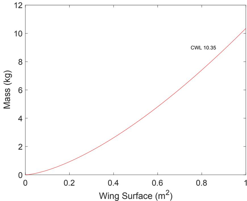
**Figure 2.3** CWL line for basic model.
