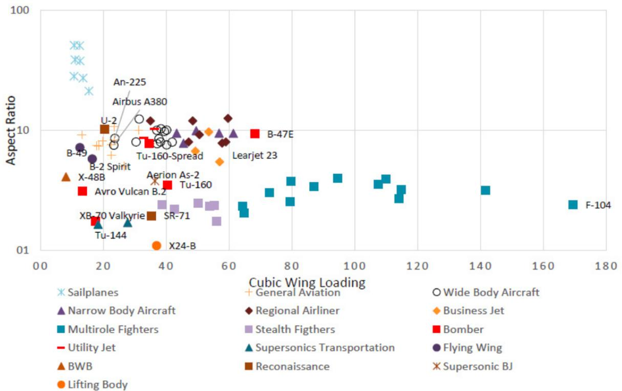
**Figure 2.6** Aspect ratio and cubic wing loading chart of 81 aircraft. A base 10 log. Scale for AR was used for the readability of the scatter plot. (Durmus 2020)
