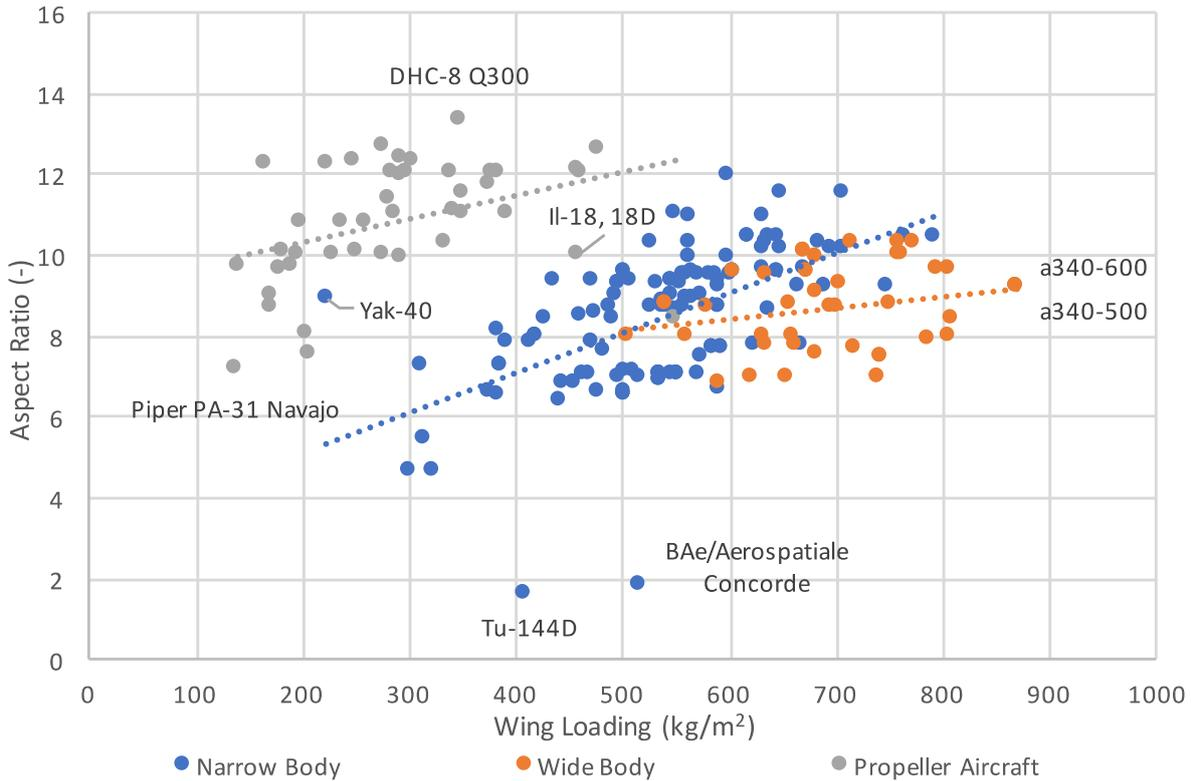
**Figure 5.6** Aspect Ratio and Wing Loading.
