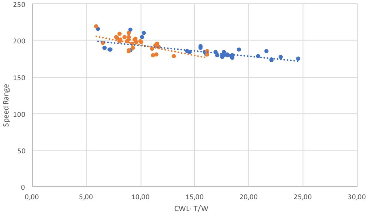
**Figure 6.2** Speed Range and Performance Factor for 72 Airbus and Boeing's models (CWL·T/W).
