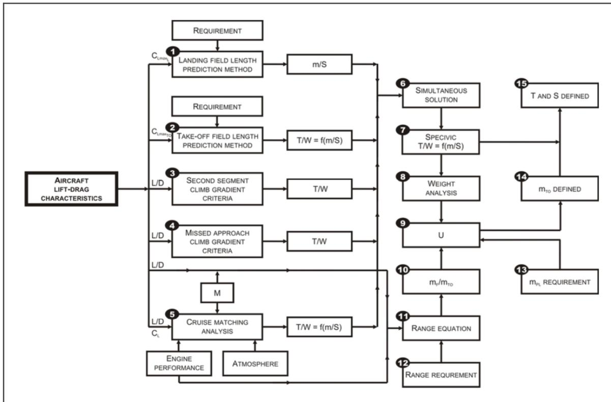
**Figure 4.1** Flow chart of the aircraft preliminary sizing for jets (Scholz 2015). Based on (Loftin 1980).
