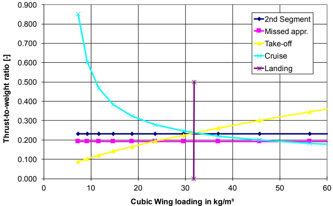
**Figure 4.2** Matching chart. Lines mark restrictions as imposed by equations.
