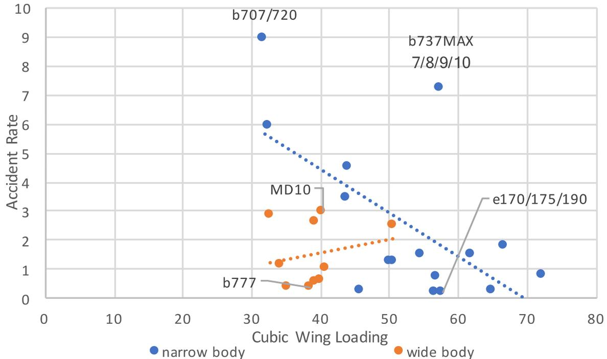
**Figure 6.6** Accident Rate over Cubic Wing Loading for narrow-body and wide-body aircraft.**Table 6.4** Trend-line's data for Figure 6.6.
