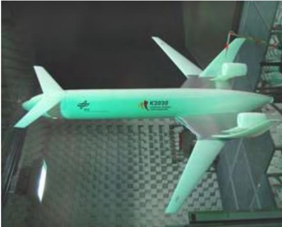
**Figure A.3** Model of the LNA configuration in the acoustic wind tunnel Braunschweig (from **DLR Report 2008**)
