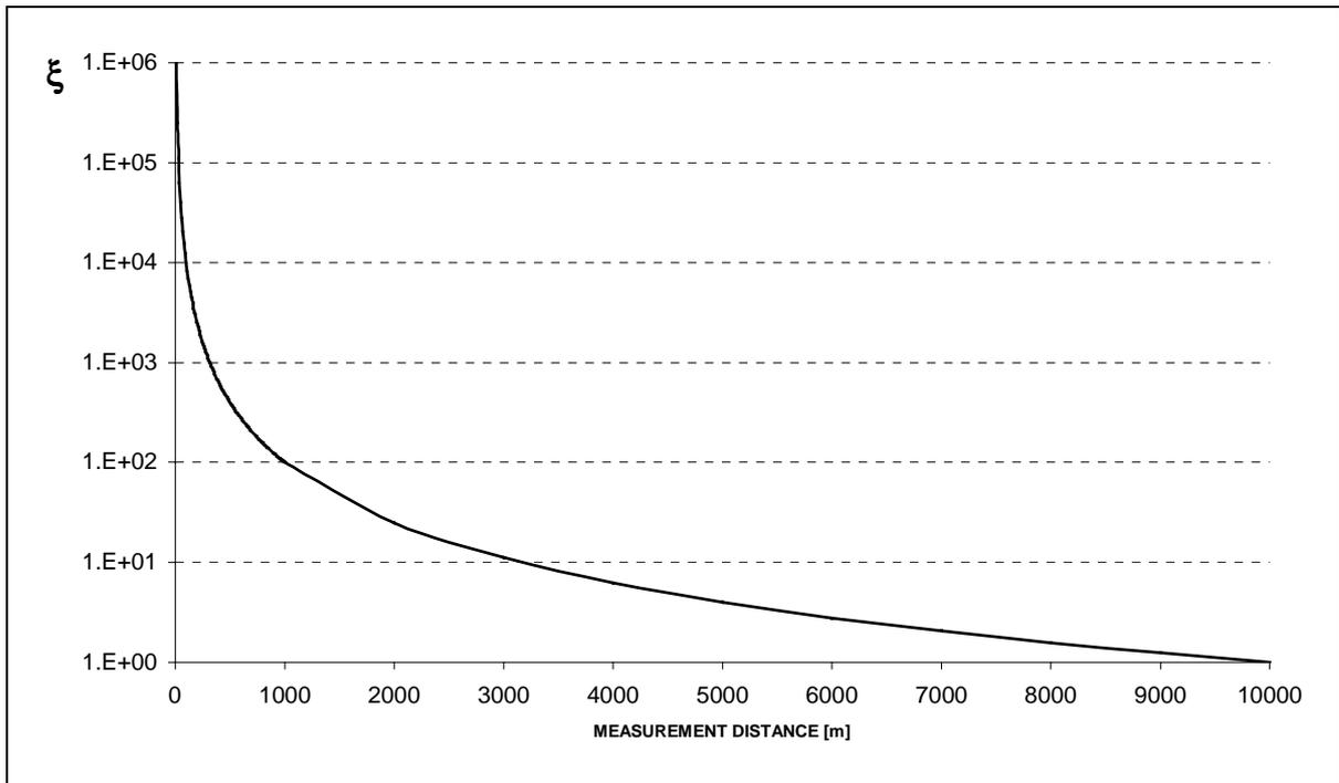
Fig.: 17-7 The distance-ratio over the measurement distance for ODIN-3
