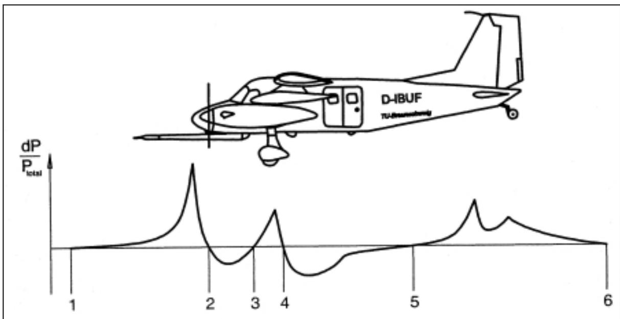
Fig.: 8-1 The computed position error on the DO 128 (Delft 1999)
