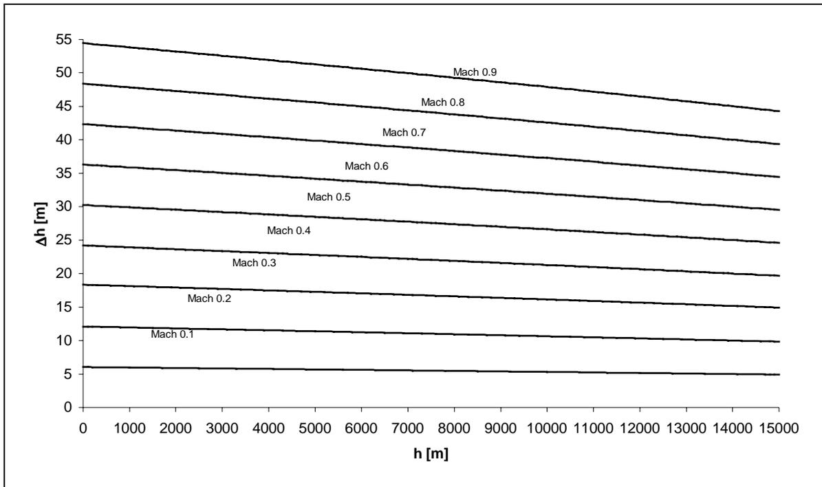
Fig.: 7-1 The altitude error of the FAR, over the height and Mach number
