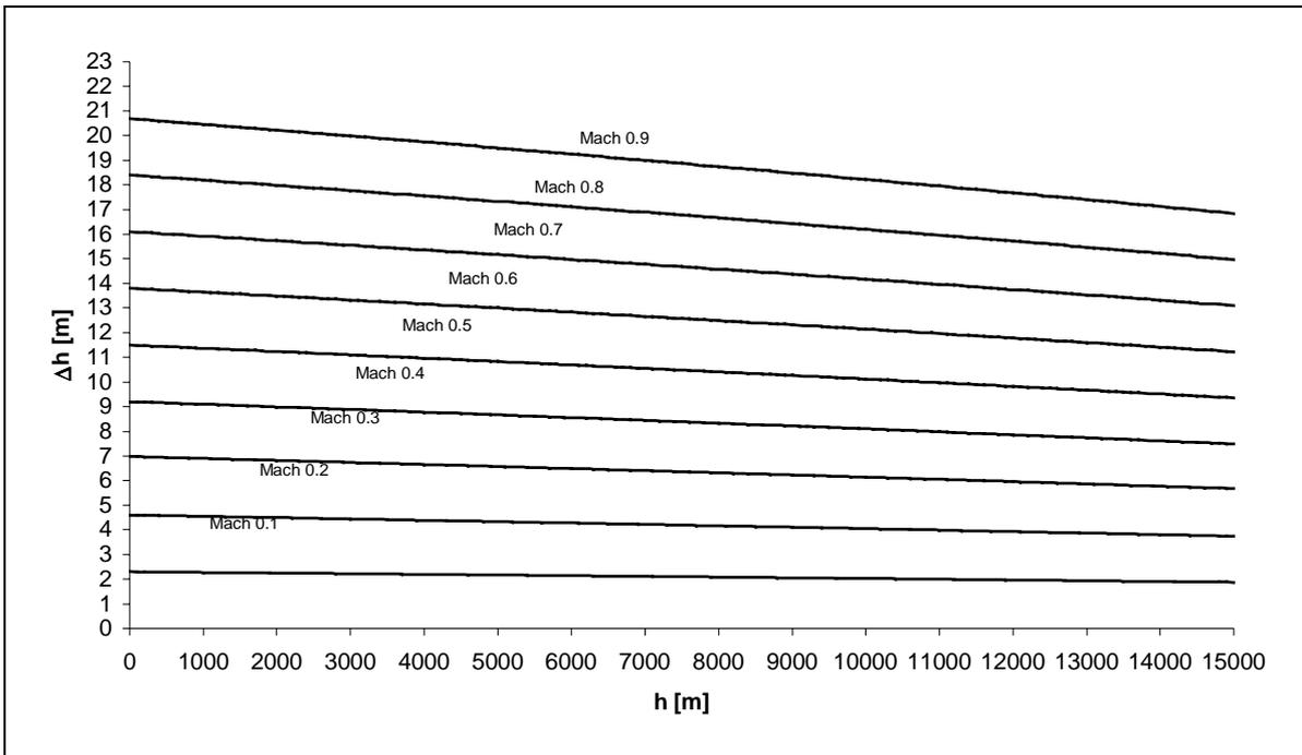
Fig.: 7-2 The altitude error of the I.C.A.O. over the height and Mach number
