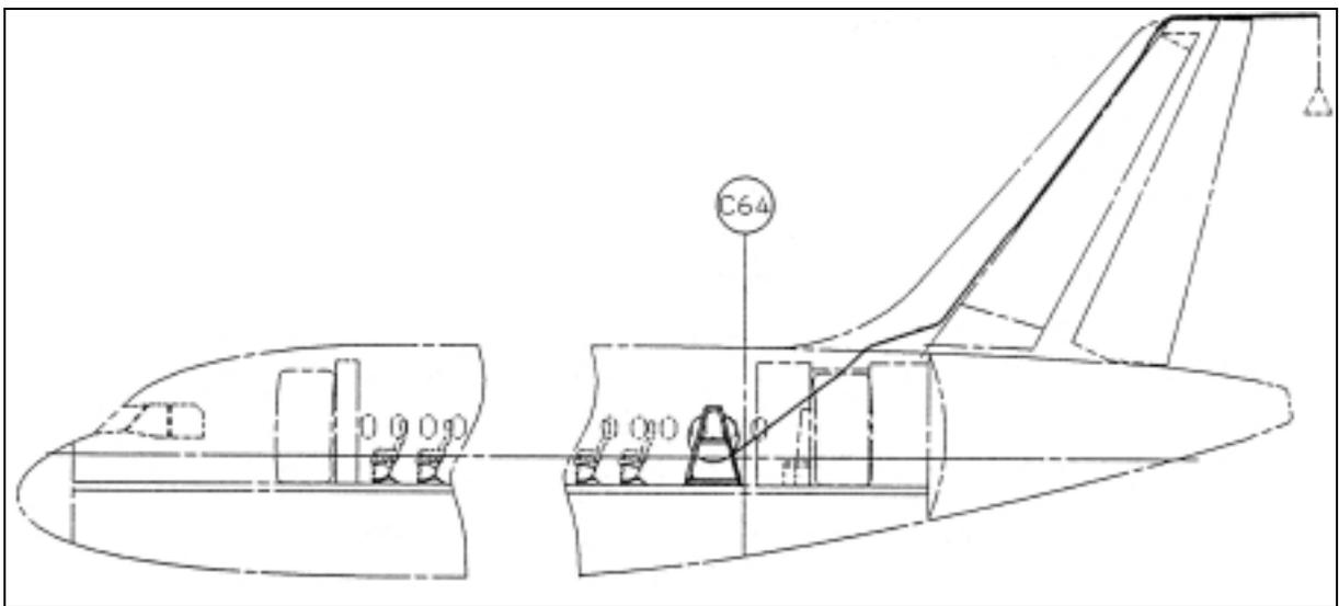
Fig.: 9-1 The trailing cone on Airbus (ETF)
