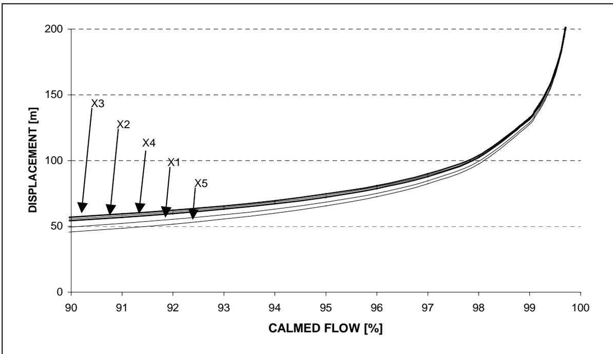
Fig.: 3-8 The calmed flow over the fuselage due to the displacement in x-steps
