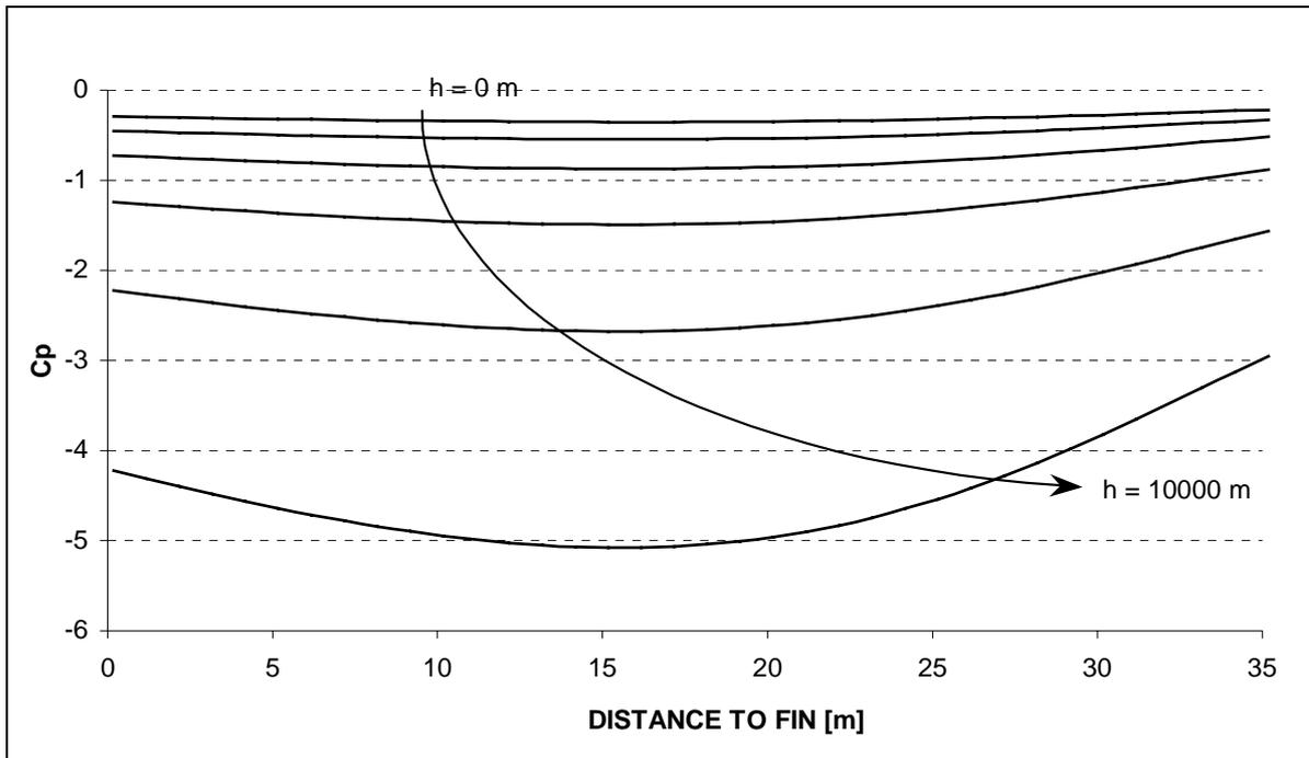
Fig.: 13-2 The pressure coefficient  $c_p$  over distance to fin in variable height (Mach 0,3)
