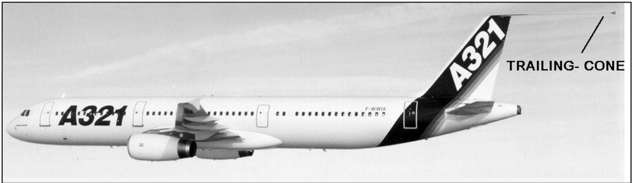
Fig.: 8-4 The trailing cone calibration method on the A321 (Airbus)
