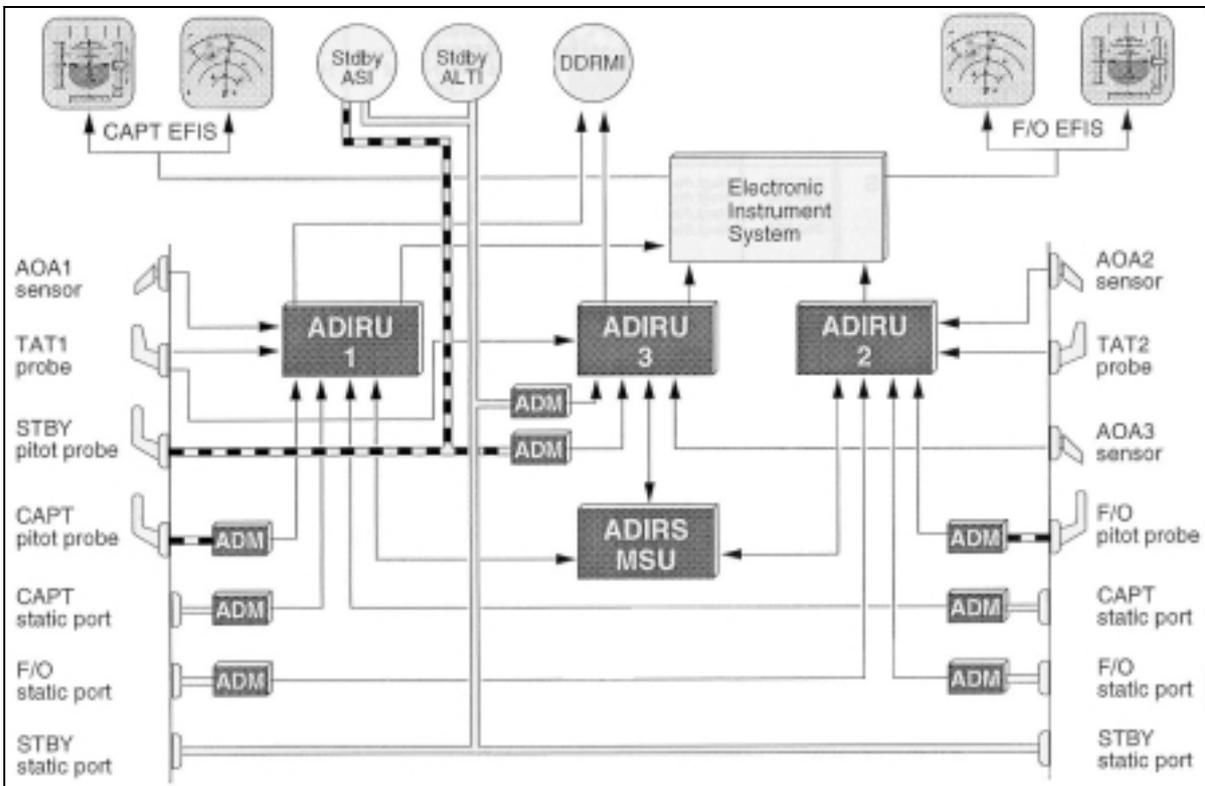
Fig.: 4-3 The pressure measurement system on Airbus A330/A340 (SCG 1997)
