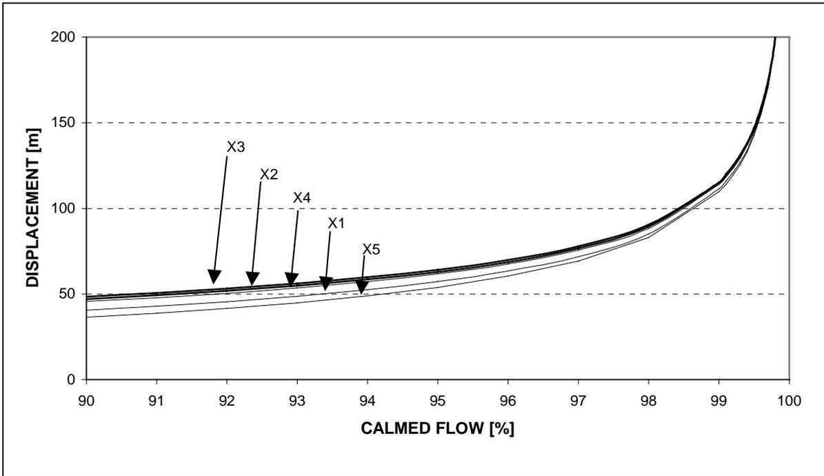
Fig.: 3-7 The calmed flow besides the fuselage over the displacement in x-steps
