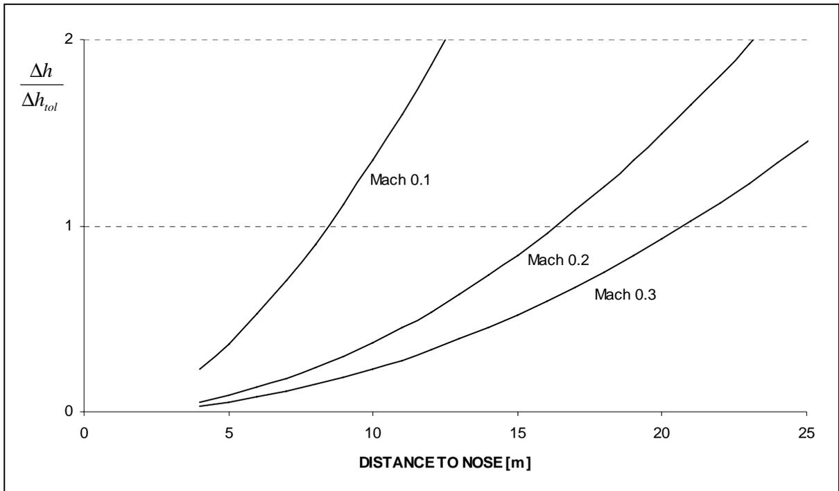
Fig.: 13-6 The height error relation over distance to fin (Mach 0,1–0,3)
