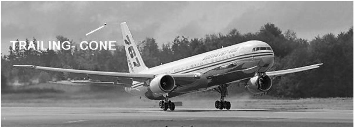
Fig.: 10-3 The Boeing 767-400 with trailing-cone
