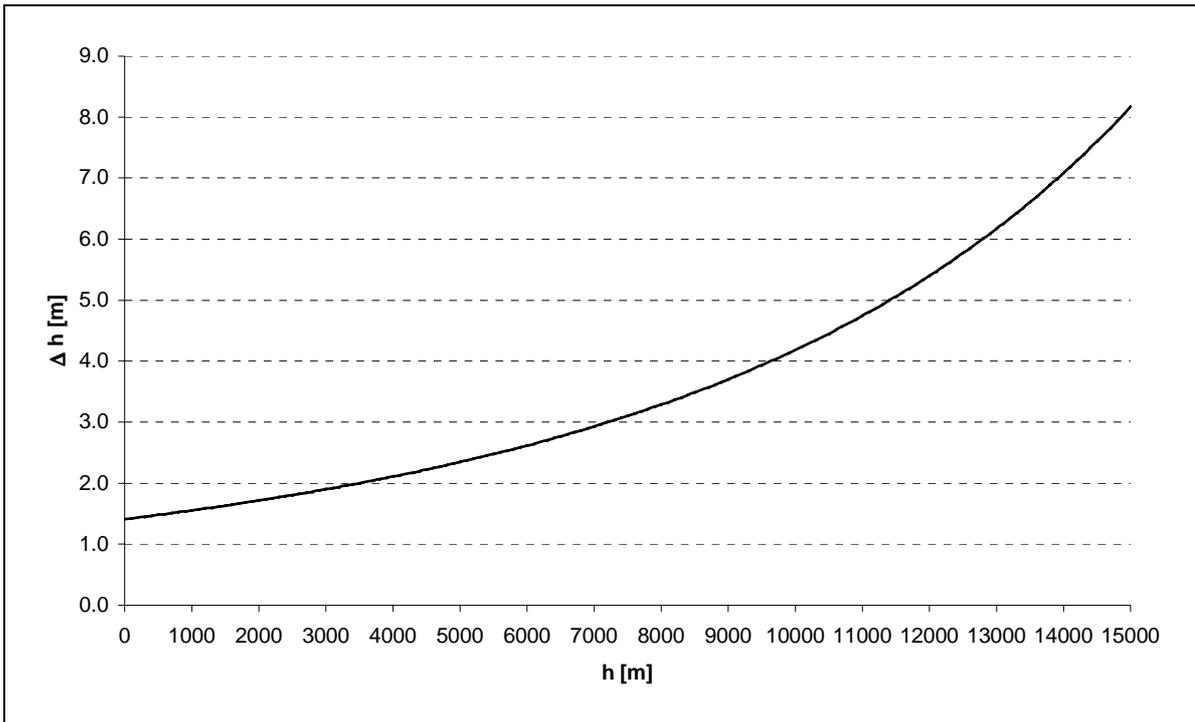
Fig.: 7-4 The altitude error of the calibration equipment
