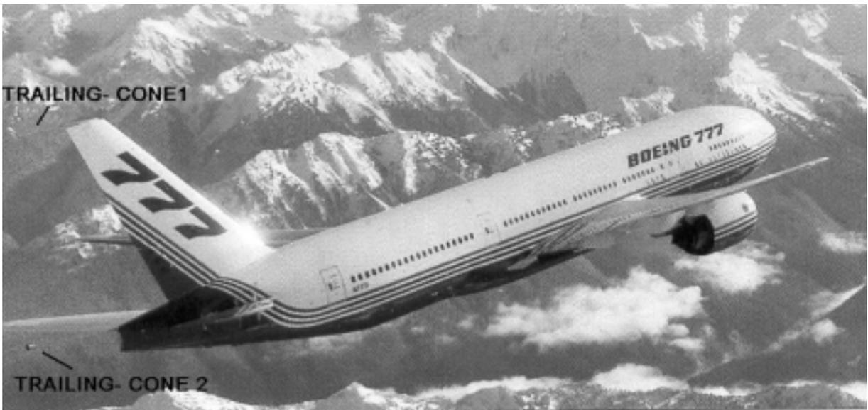
Fig.: 10-4 The Boeing 777 with two different trailing-cones
