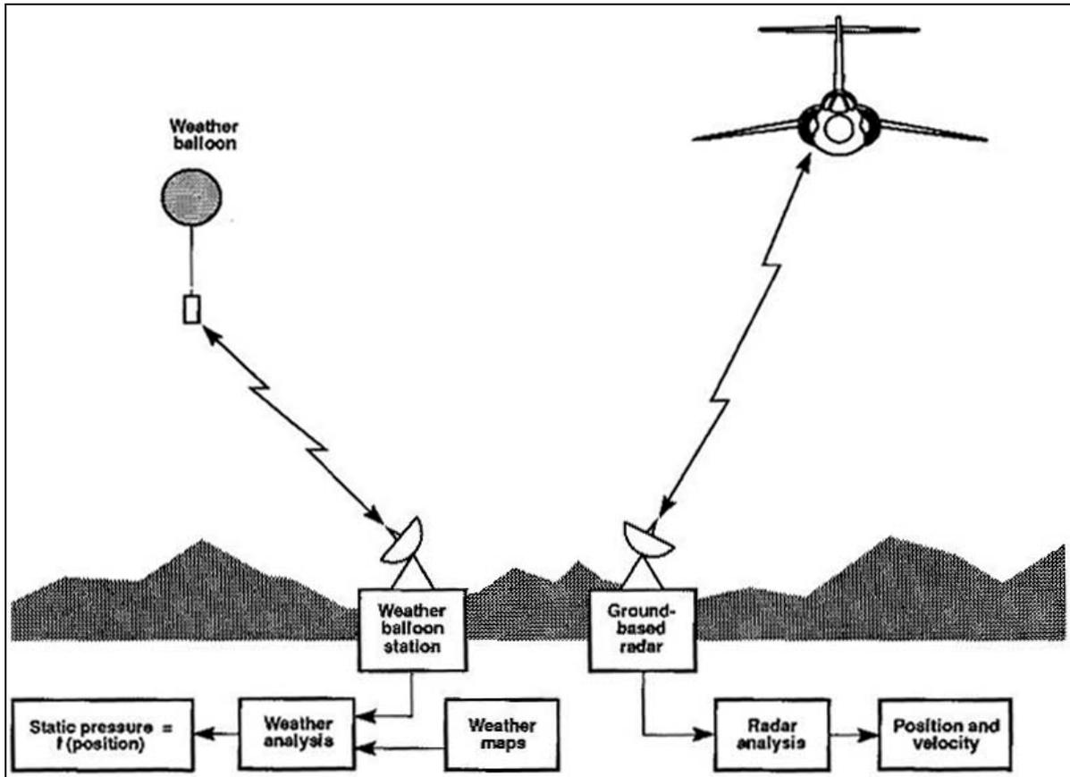
Fig.: 8-3 The radar tracking method
