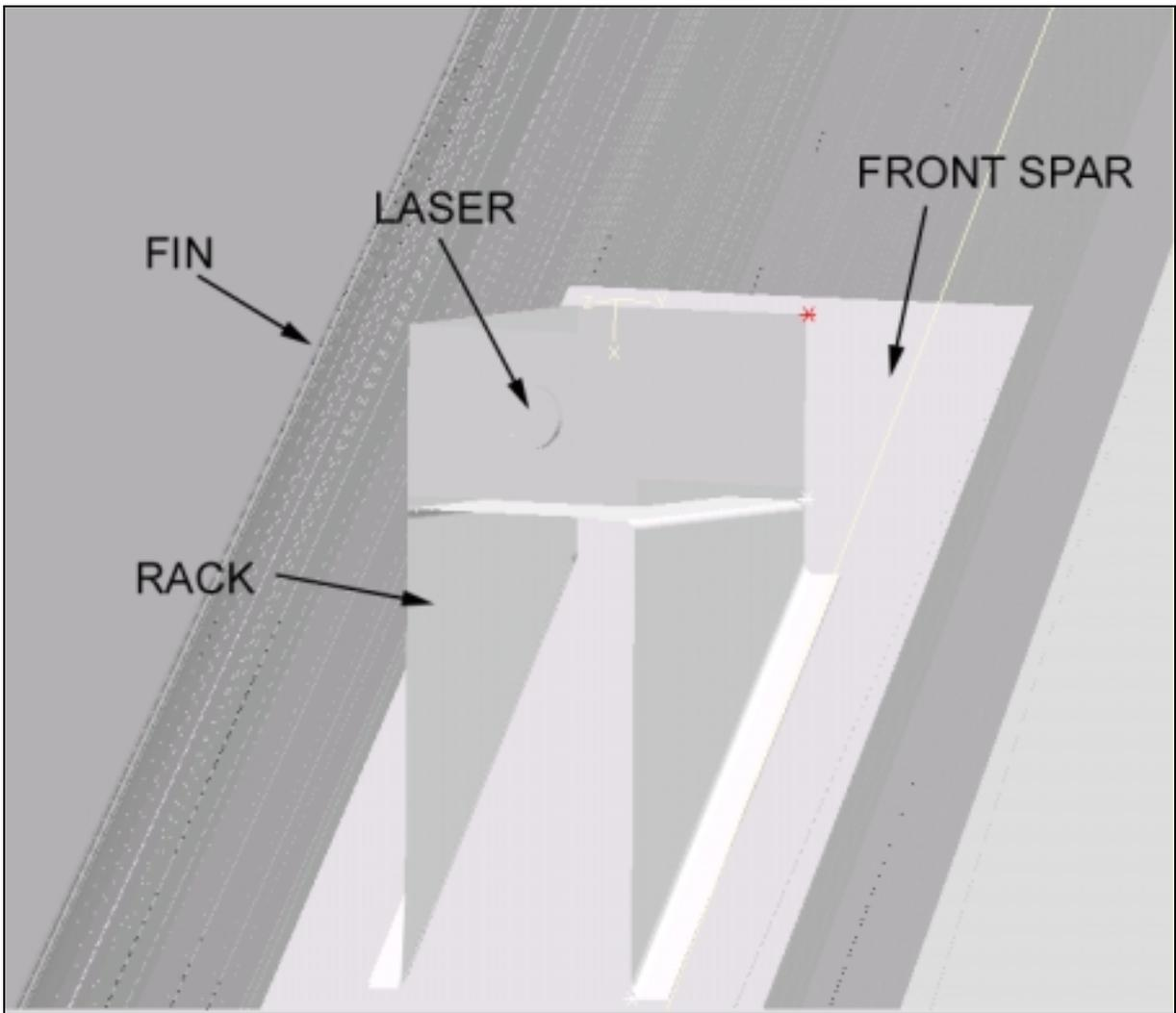
Fig.: 17-12 The laser attached on the front spar of the fin
