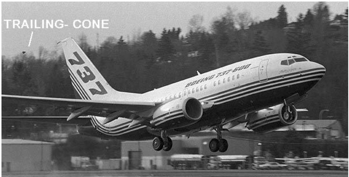
Fig.: 10-1 The Boeing 737-600 with trailing-cone
