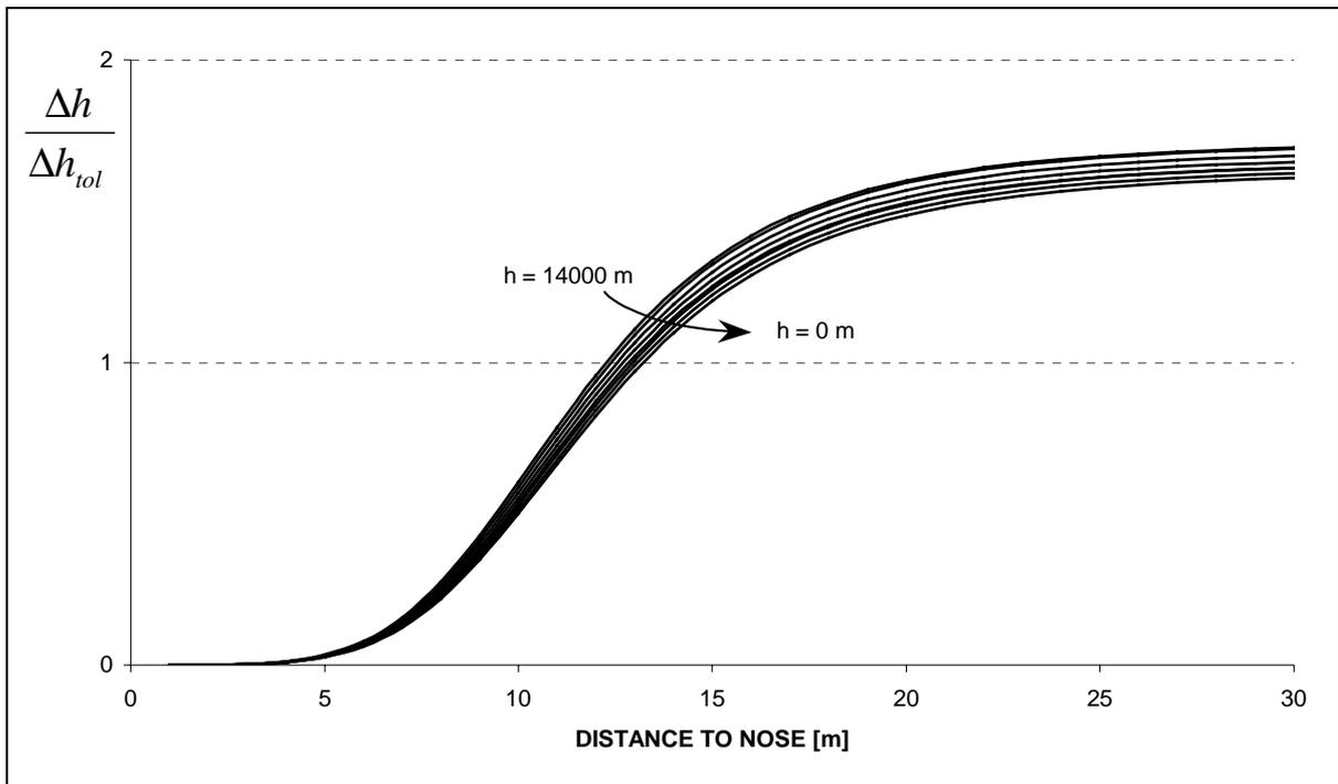
Fig.: 17-5 The height error relation over distance to nose in steps of 2000 m (Ma 0,9)
