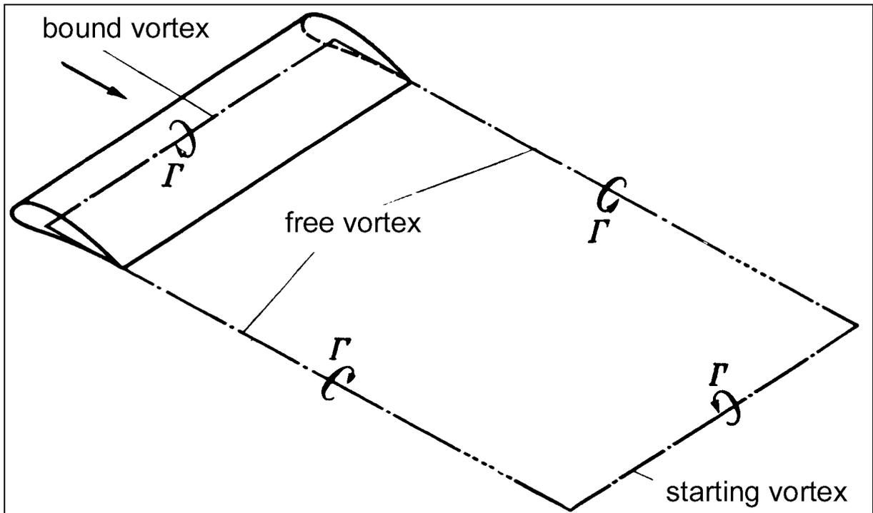
Fig.: 3-11 The circulation of the wing with finite span
