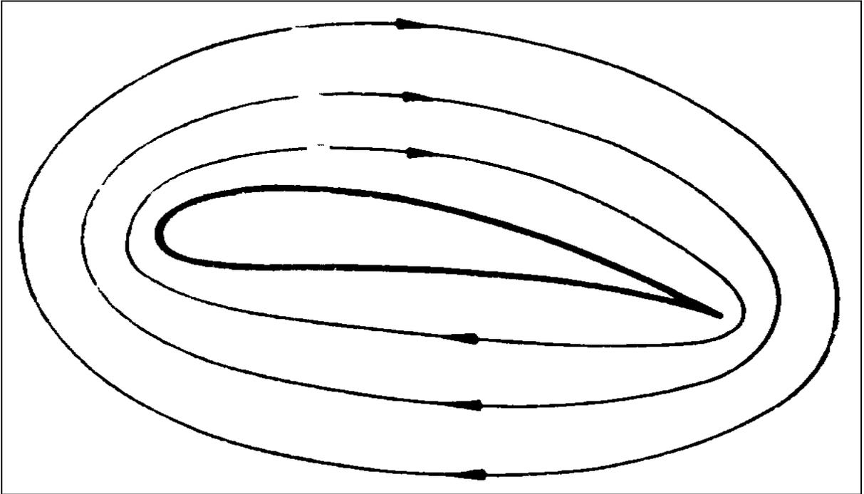
Fig.: 3-10 The circulation of the wing shape
