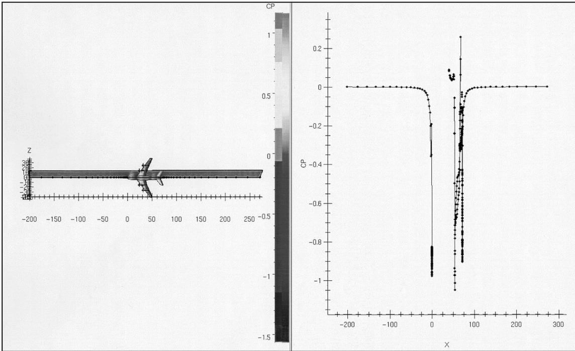
Fig.: 13-7 The pressure coefficient  $c_p$  for the A3XX (EFD)
