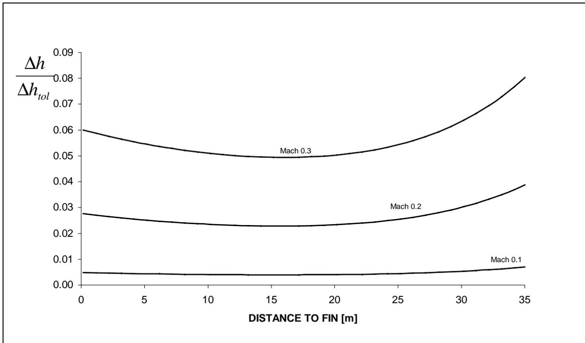
Fig.: 13-3 The height error relation over distance to fin (Mach 0,1–0,3)
