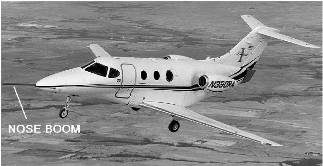
Fig.: 10-11 The Raytheon Aircraft's Premier with nose boom
