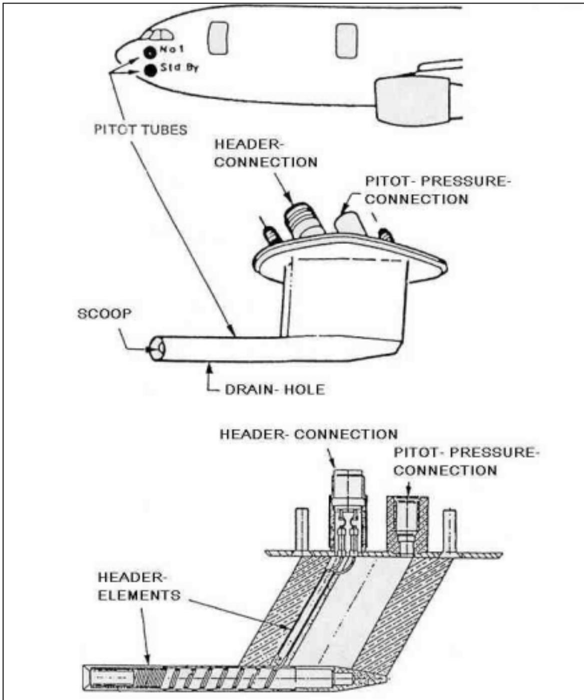
Fig.: 4-1 The pitot tube on aircraft
