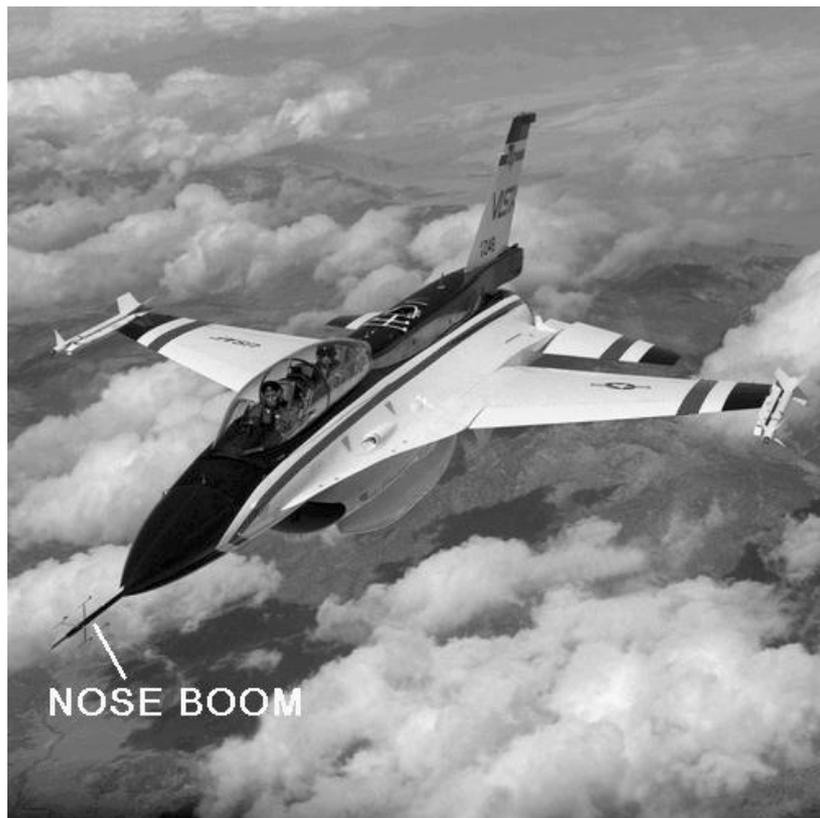
Fig.: 8-5 The nose boom calibration method on the F16 (NASA)
