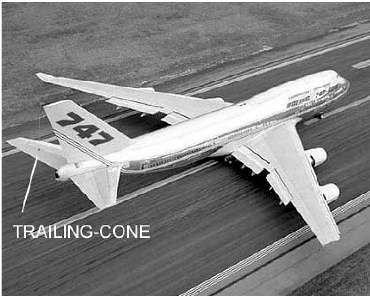
Fig.: 10-2 The Boeing 747-400 with trailing-cone
