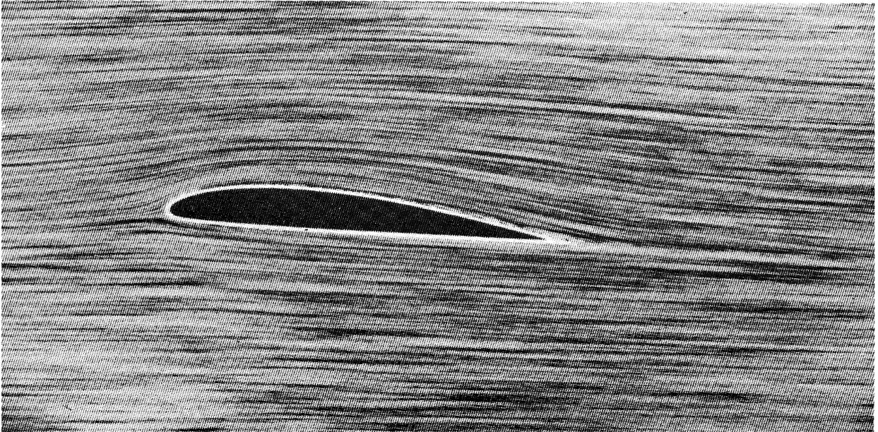
Fig.: 3-3 The displacement on a wing shape
