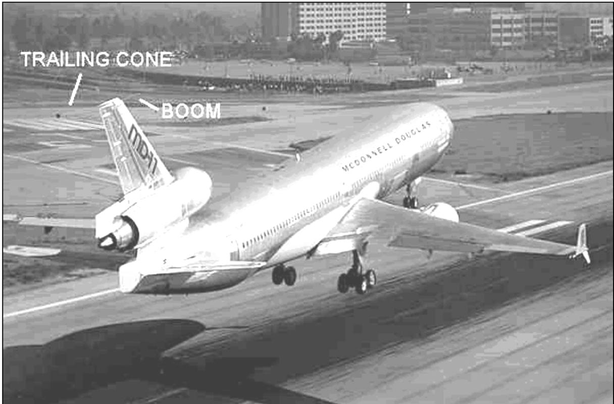
Fig.: 10-10 The Mc Donnell Douglas MD 11 with trailing-cone and boom
