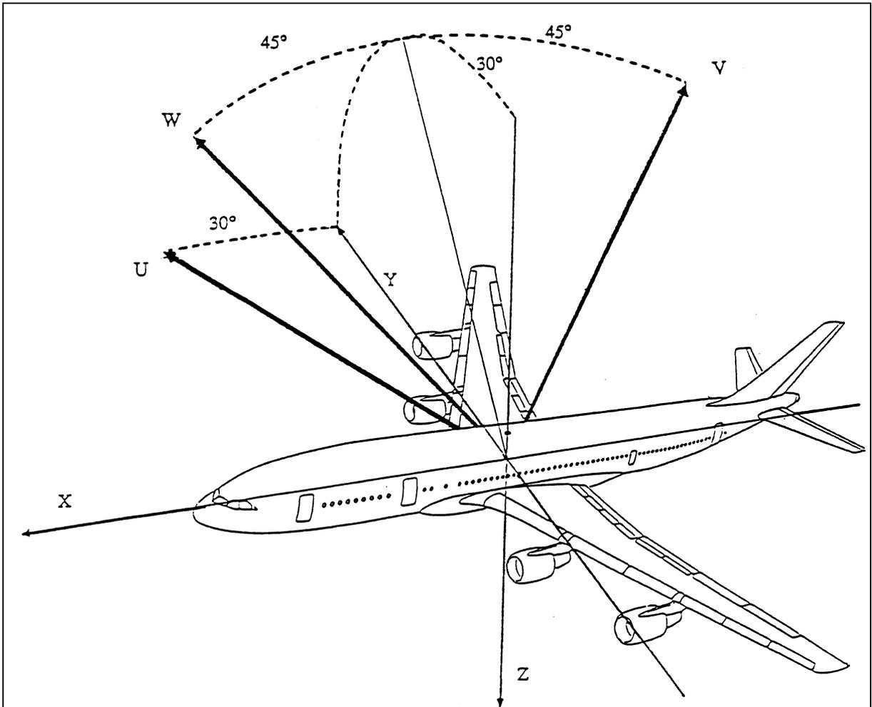
Fig.: 9-2 The 3D laserbeam overview of ALEV3
