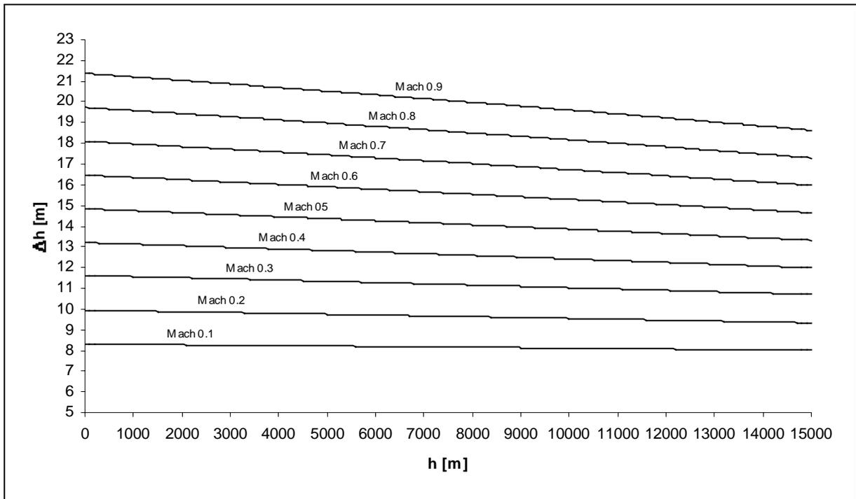
Fig.: 7-4 The altitude error of FAR and I.C.A.O. over the height and Mach number
