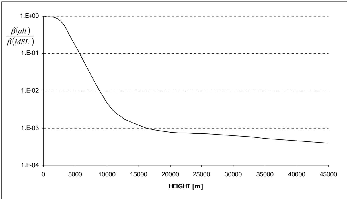
Fig.: 17-6 The aerosol backscatter ratio over the height
