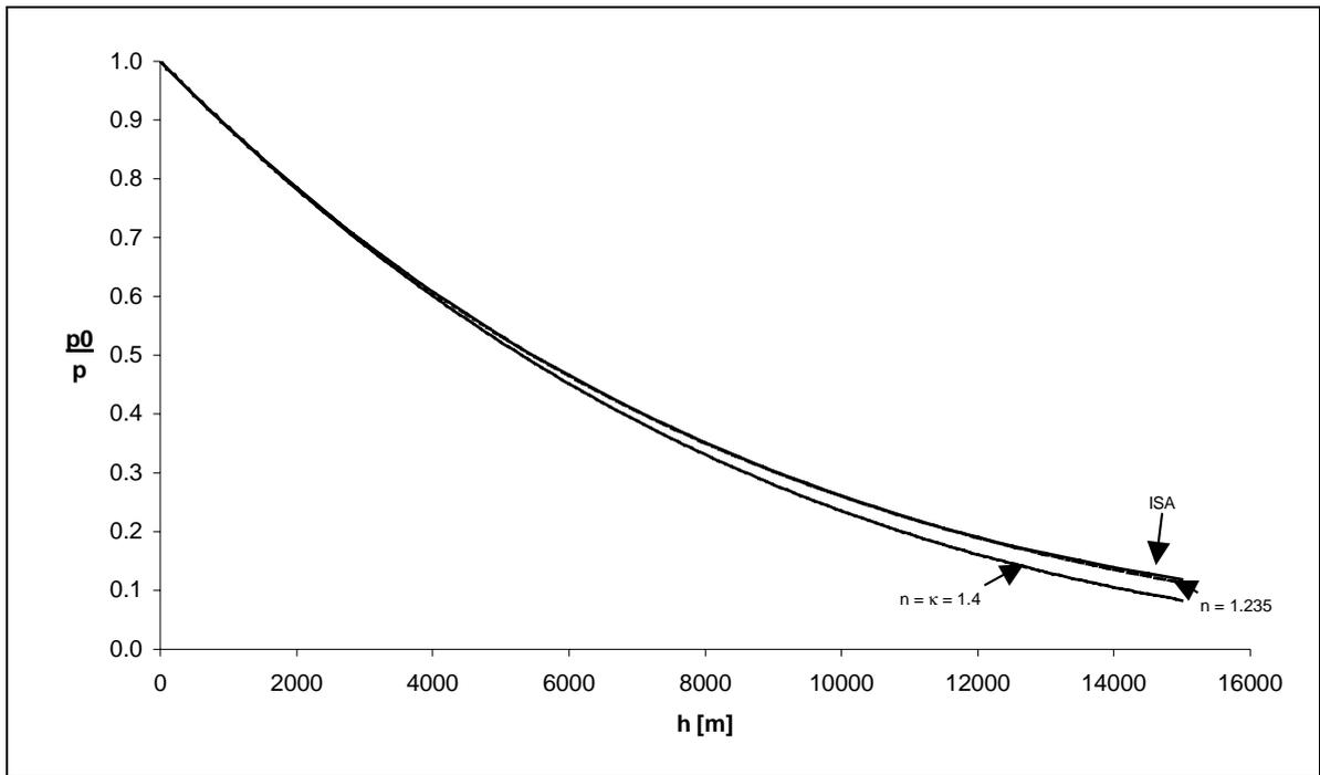
Fig.: 3-2 The different exponents of the atmosphere ( $p/p_0$  over the height)
