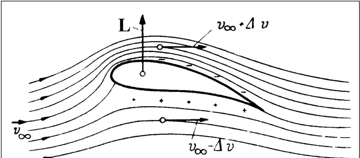
Fig.: 3-9 The lift of the wing shape
