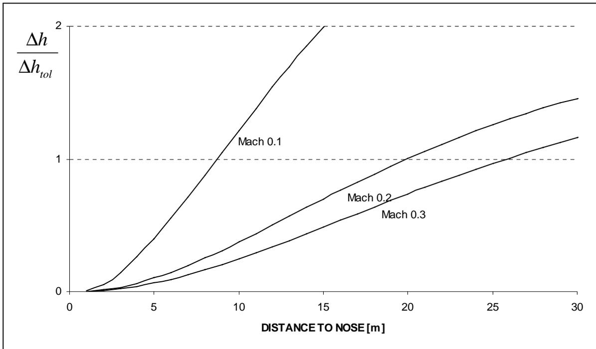
Fig.: 17-3 The height error relation over distance to nose (Mach 0,1-0,3) at MSL
