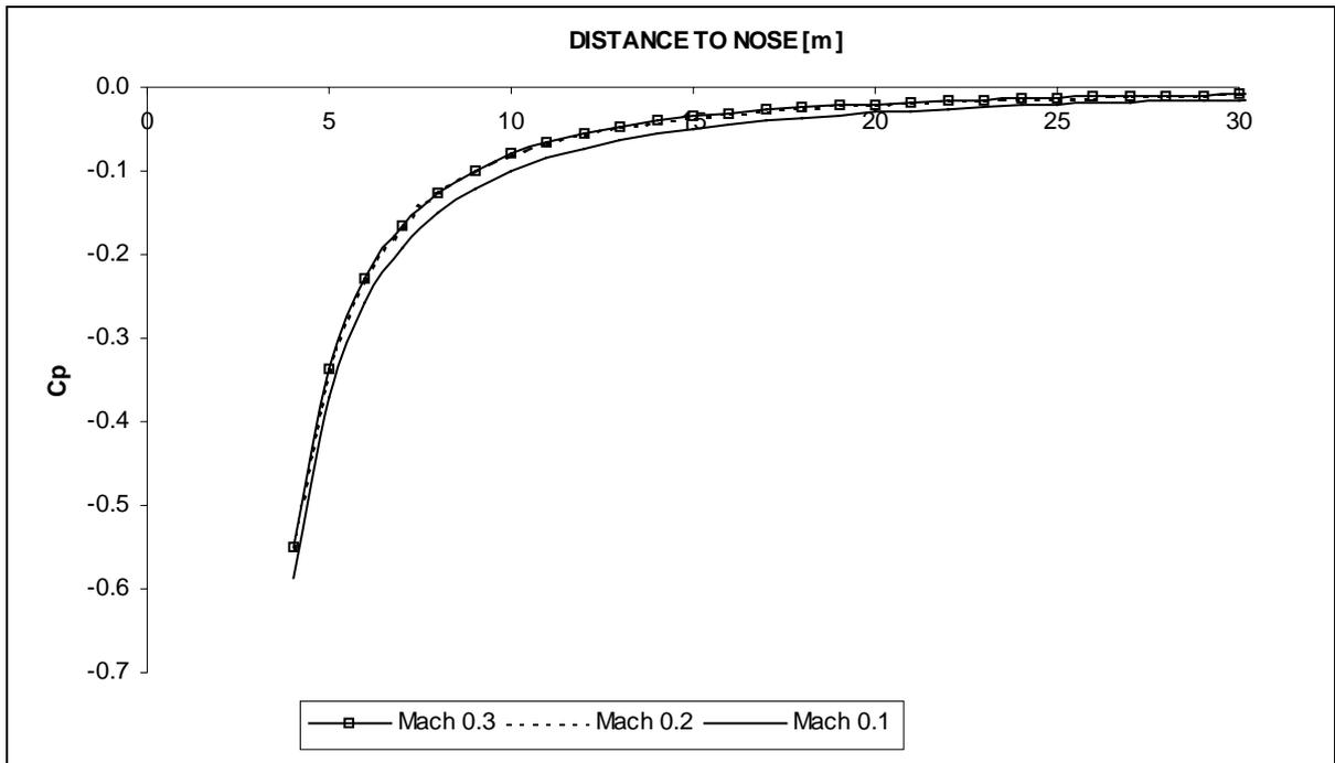
Fig.: 13-5 The pressure coefficient  $c_p$  over distance to nose (Mach 0,1-0,3)
