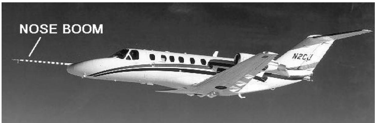
Fig.: 10-7 The Cessna Citation CJ2 with nose boom
