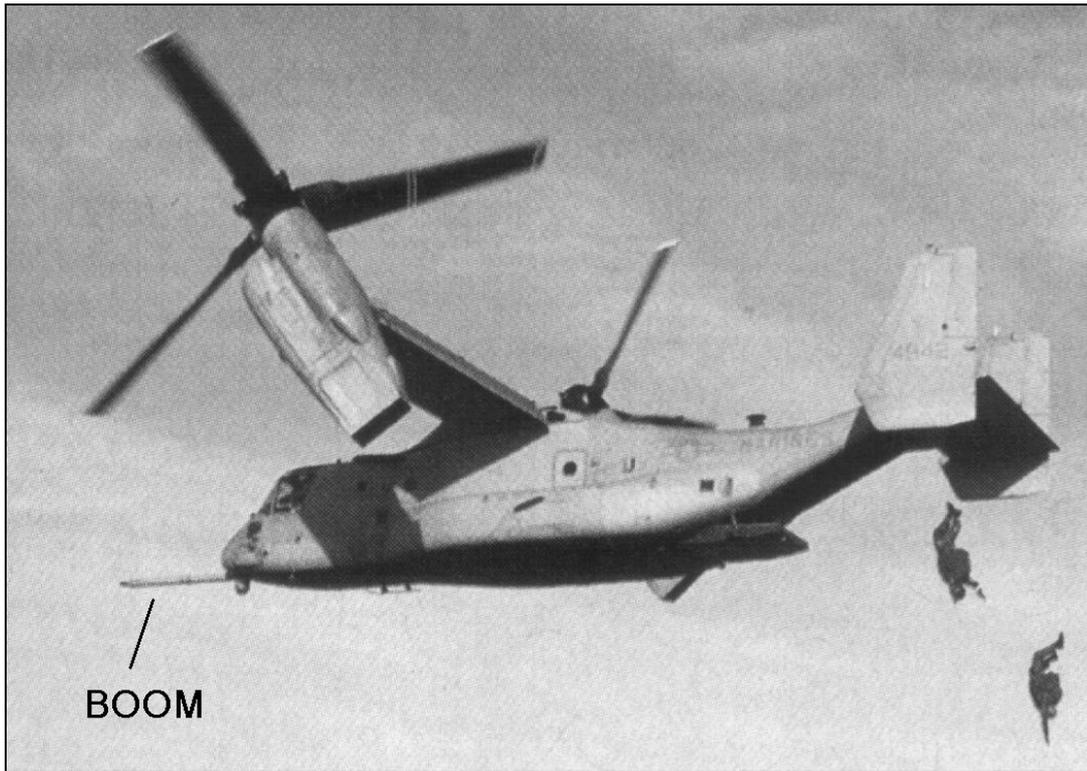
Fig.: 10-5 The Boeing Osprey with nose boom
