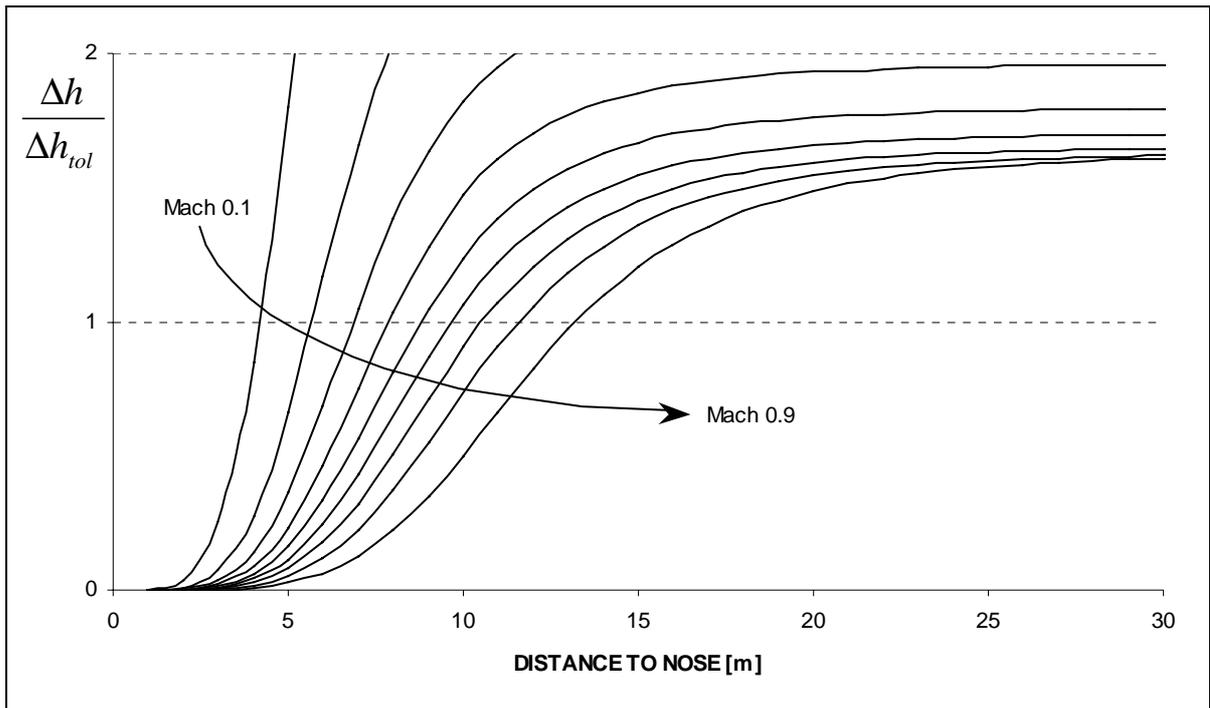
Fig.: 17-4 The height error relation over distance to nose (Mach 0,1-0,9) at MSL
