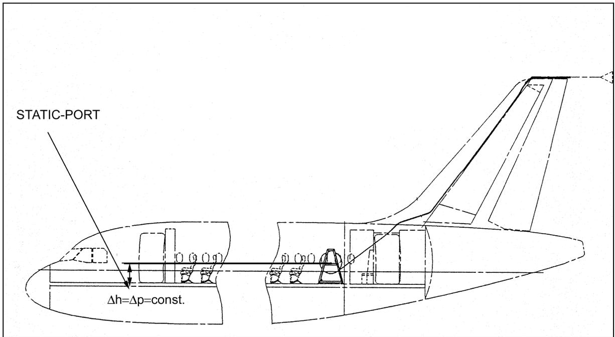
Fig.: 12-2 The trailing cone indirect measurement (ETF)
