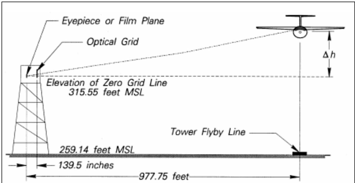
Fig.: 8-2 The tower fly-by calibration method
