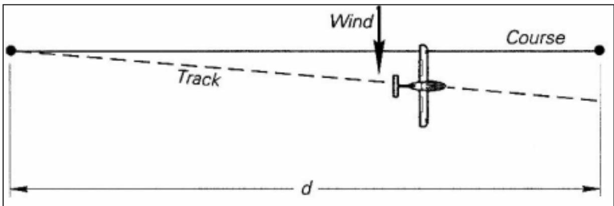
Fig.: 8-6 The speed-course calibration method
