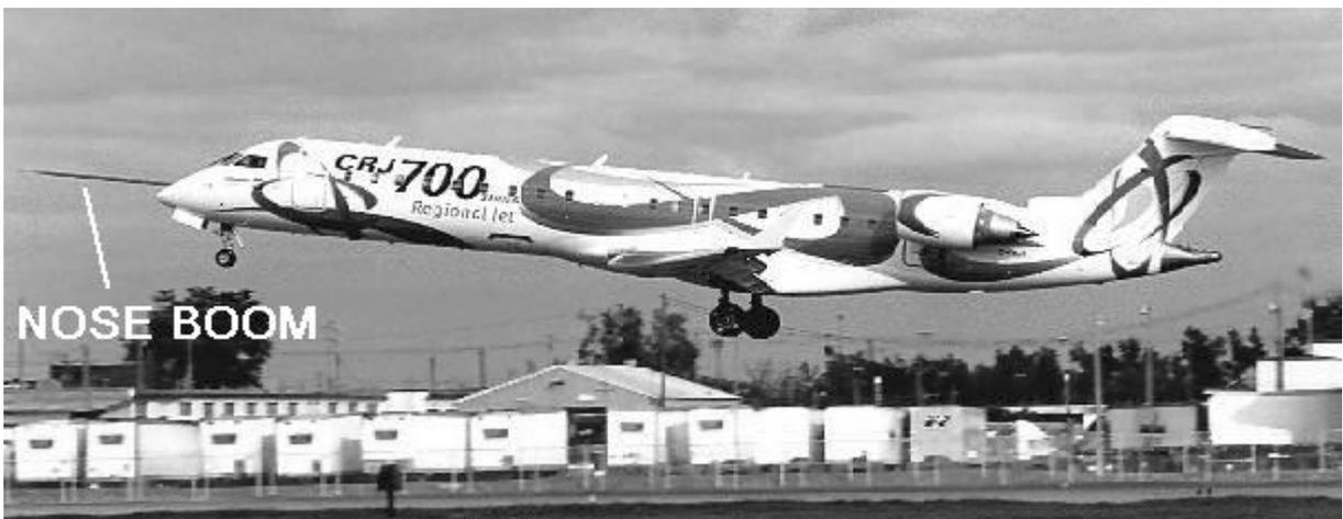
Fig.: 10-6 The Bombardier CRJ700 with nose boom
