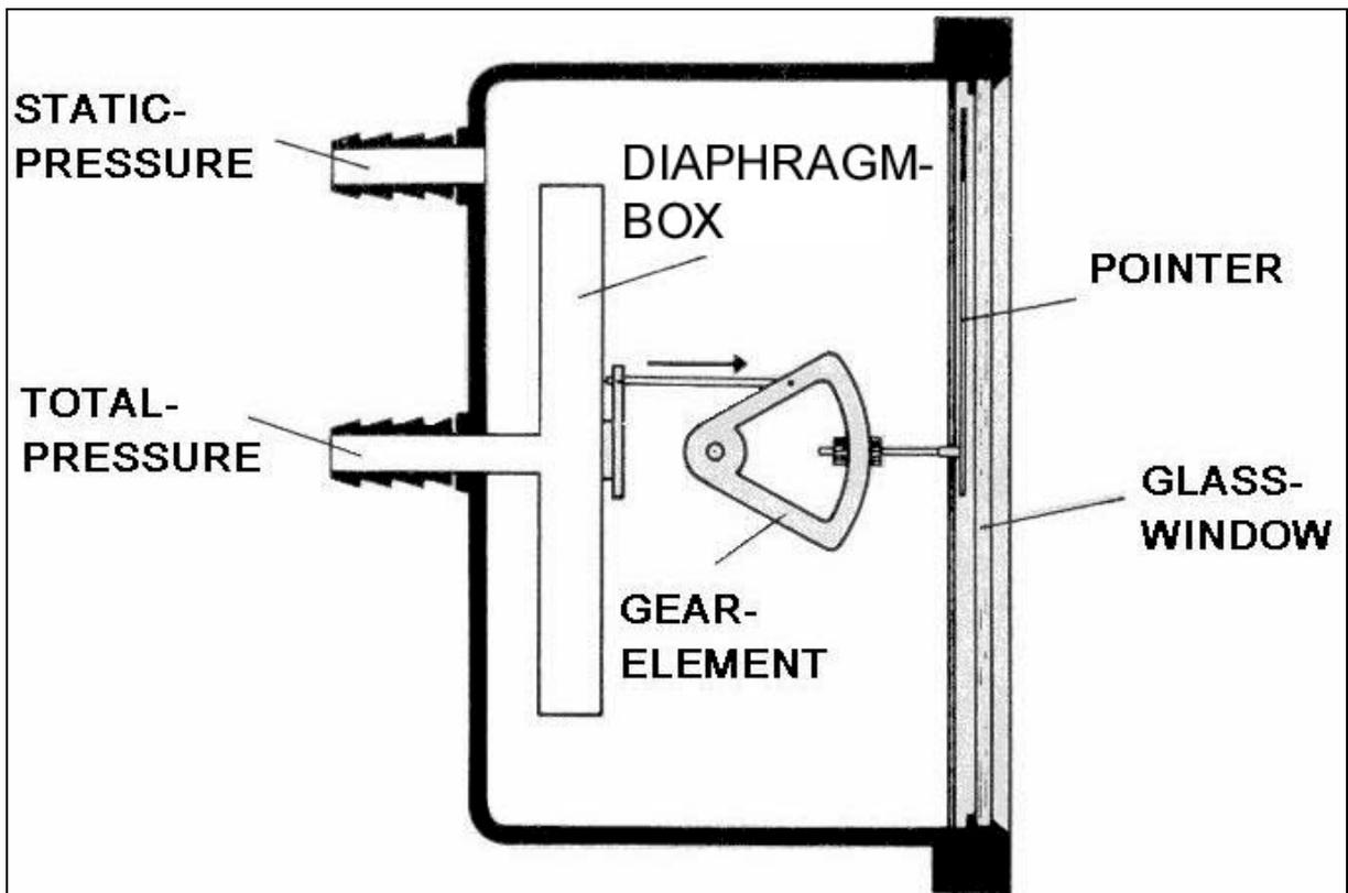
Fig.: 5-5 The analog airspeed indicator
