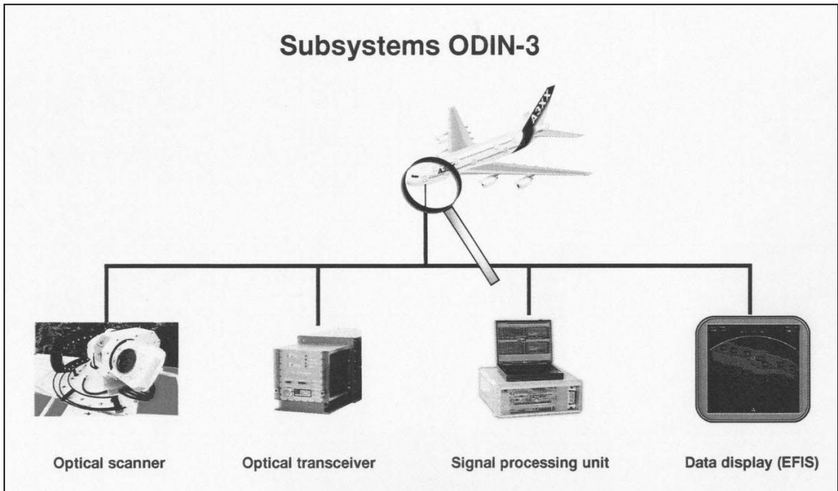
Fig.: 17-2 The subsystems of ODIN-3
