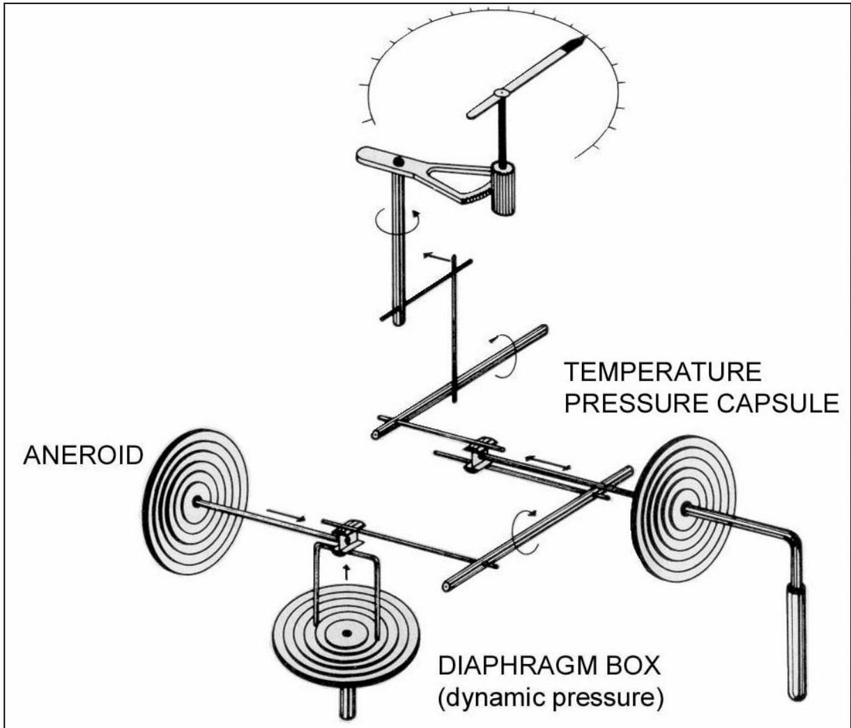
Fig.: 5-6 The analog compensating airspeed indicator
