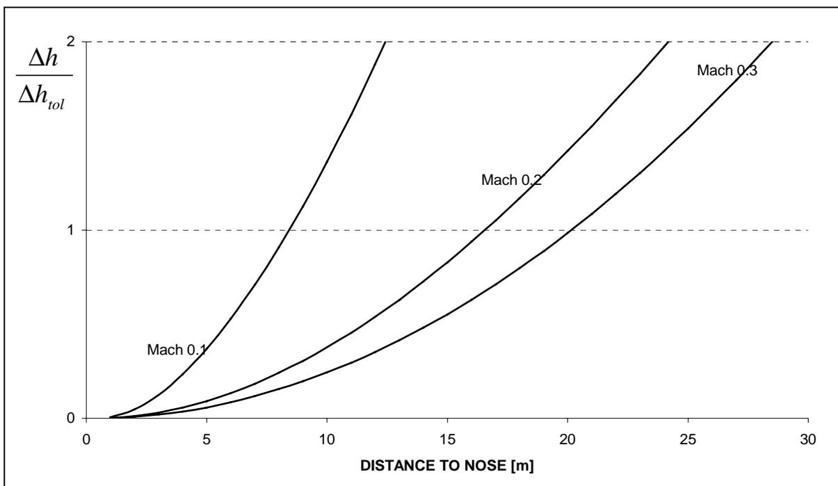
Fig.: 14-2 The height error relation over distance to nose (Mach 0,1-0,3)
