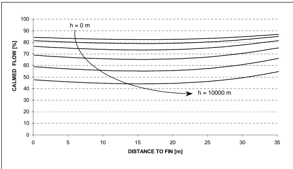
Fig.: 13-1 The calmed flow over distance to fin in variable height (Mach 0,3)
