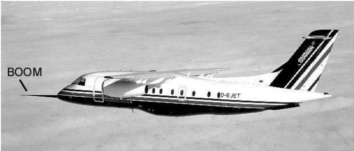
Fig.: 10-8 The Dornier Fairchild 328 Jet with nose boom
