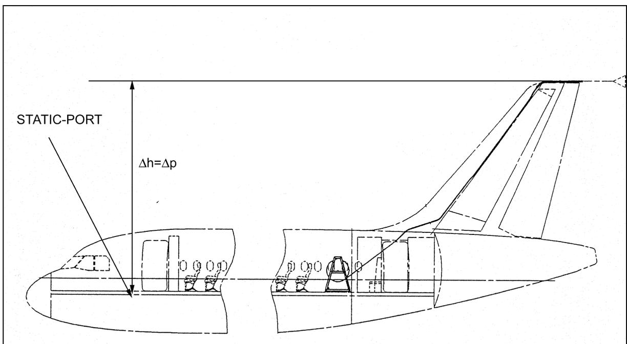
Fig.: 12-1 The trailing cone direct measurement (ETF)
