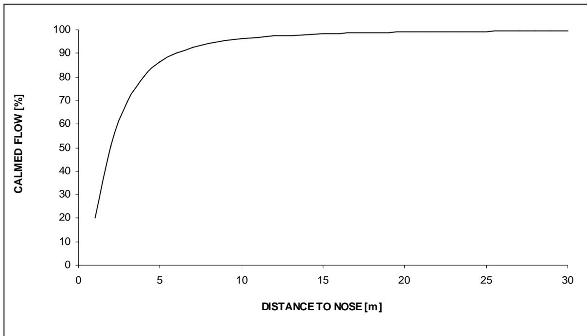
Fig.: 14-1 The calmed flow over distance to nose
