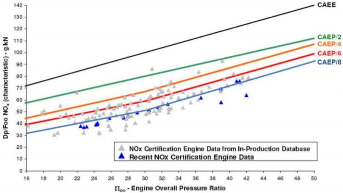
**Figure 5.14** Normalized NO<sub>x</sub> emission (g/kN) as a function of the overall pressure ratio (ICAO 2014)
