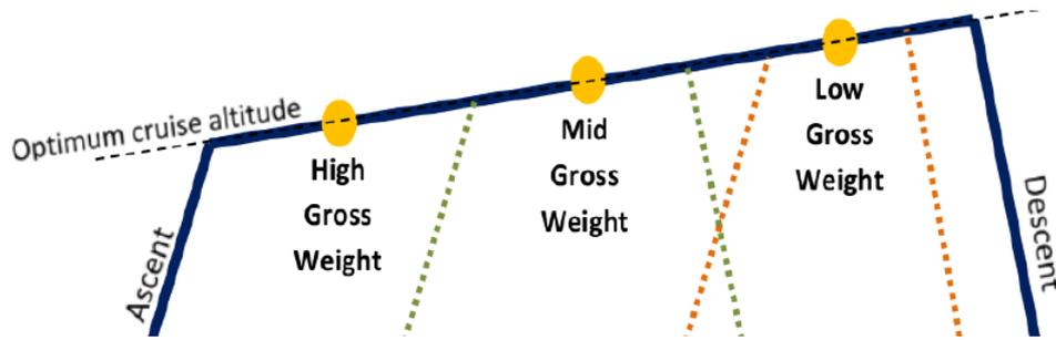
**Figure 5.19** Reference points for the determination of SAR (ICAO 2012)
