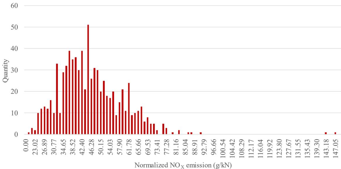
**Figure 5.15** Normalized emitted NO<sub>x</sub> for the LTO cycle (g NO<sub>x</sub>/kN thrust)
