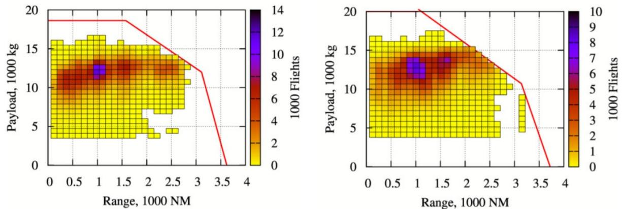
**Figure 5.9** Annual number of flights and payload-range diagram of an Airbus A320-200 (left) and a Boeing 737-800 (right) (Linke 2020)
