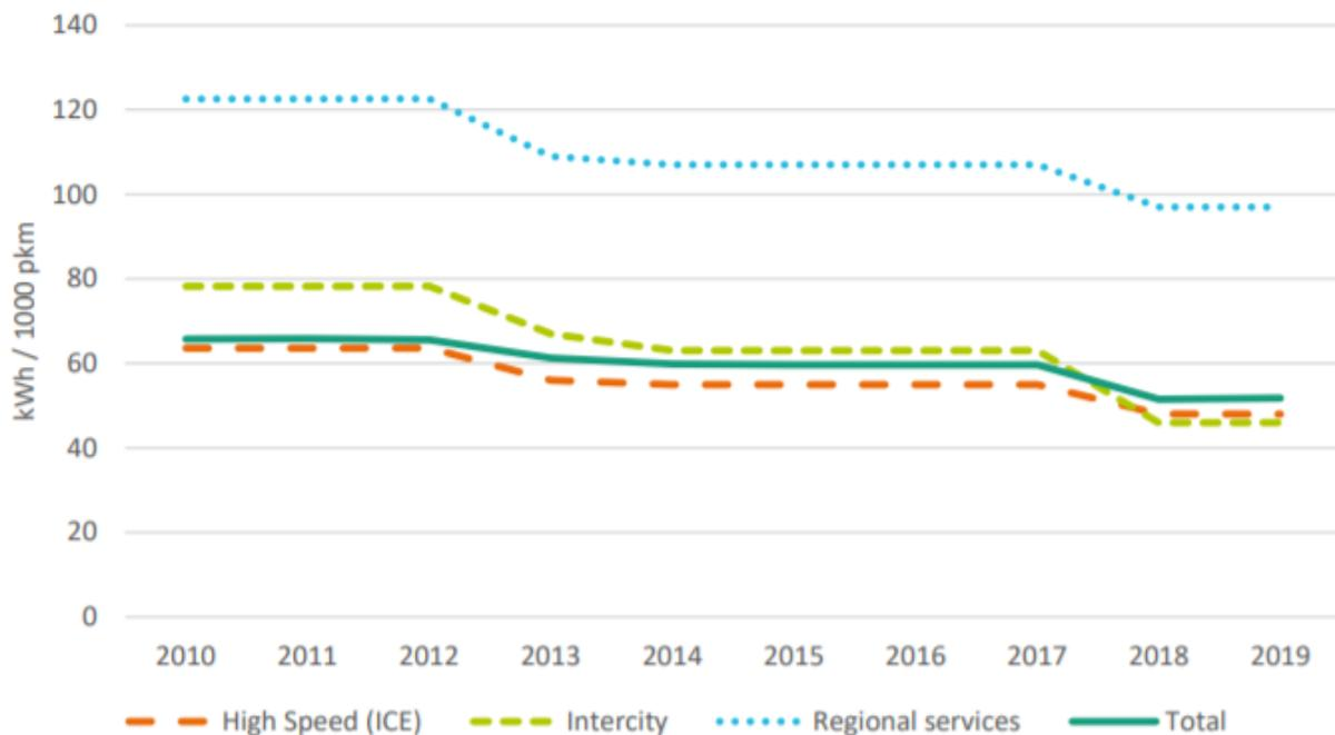
**Figure 7.11** Energy consumption of a train per passenger kilometer over time (Fraunhofer ISI 2020)
