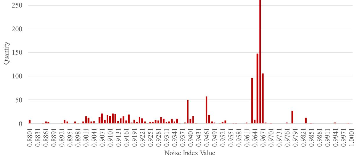
**Figure 5.27** Distribution of the noise index values for turboprop aircraft (EPNdB/EPNdB)
