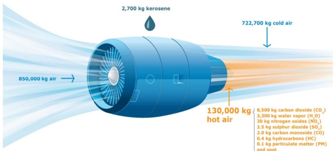
**Figure 5.12** Emissions from a 2-engine jet aircraft during 1-hour flight with 150 pax (EASA 2019a)
