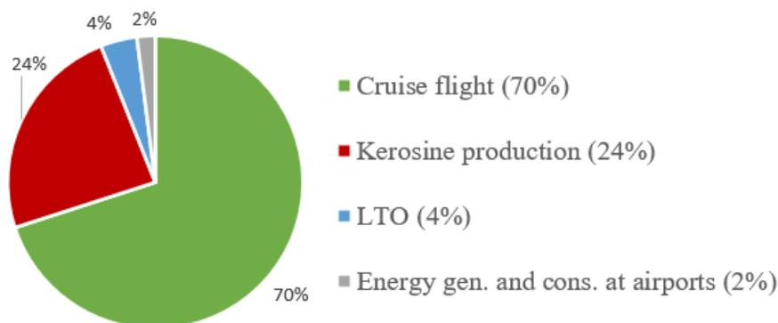
**Figure 5.3** Percentage of different processes on the environmental impact of an Airbus A320-200 adapted from (Johanning 2014)
