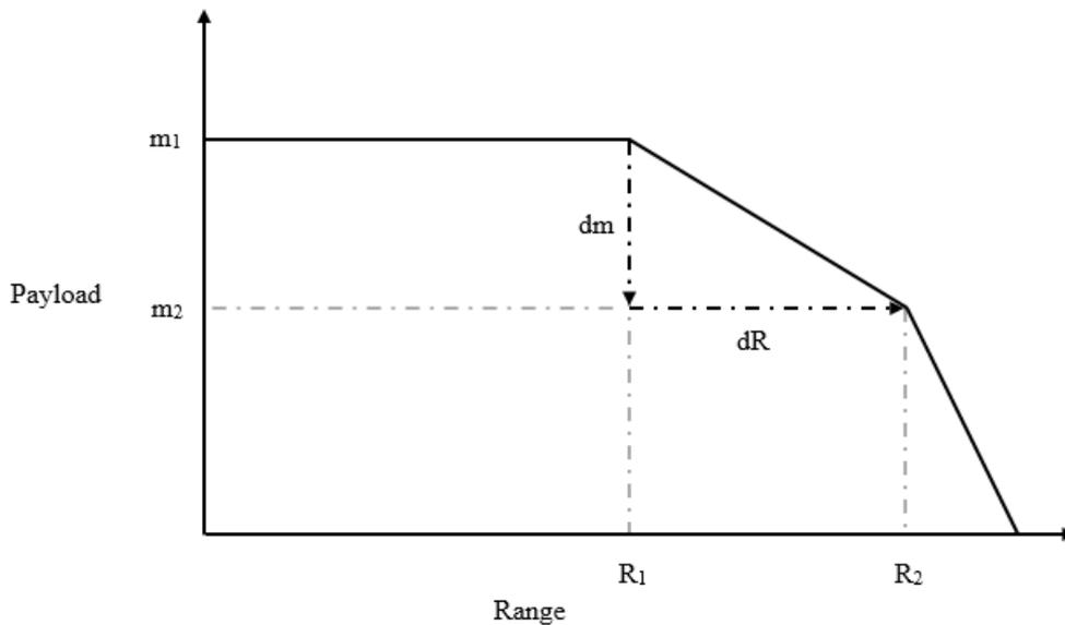
**Figure 5.5** Example of a payload-range diagram (Van Endert 2017)
