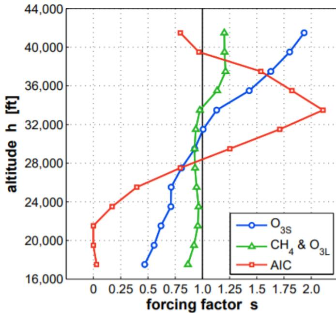
**Figure 5.20** Forcing factor  $s$  as a function of altitude (Schwartz 2011)
