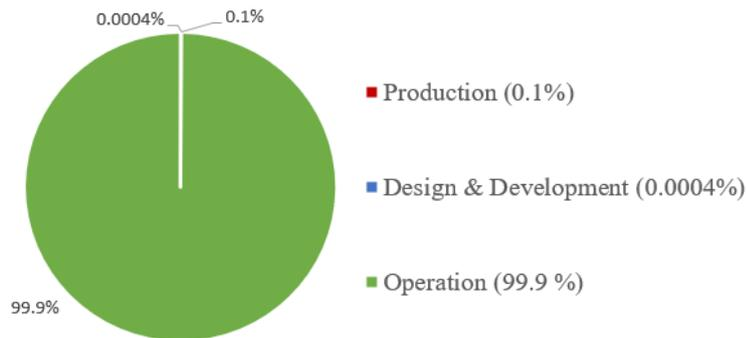
**Figure 5.2** Environmental impact of life cycle phases of an Airbus A320-200 adapted from (Johanning 2014)
