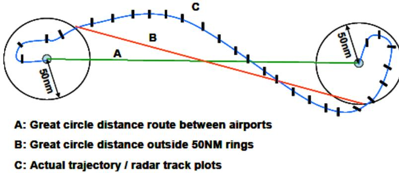
**Figure 7.6** Representation of flight inefficiency (Kettunen 2005)
