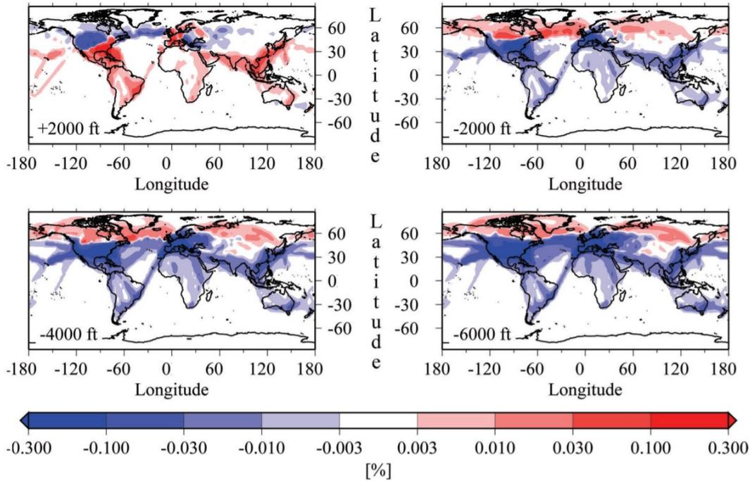
**Figure 5.18** Contrail coverage in function of altitude changes (% relative to base case) (Fichter 2005)
