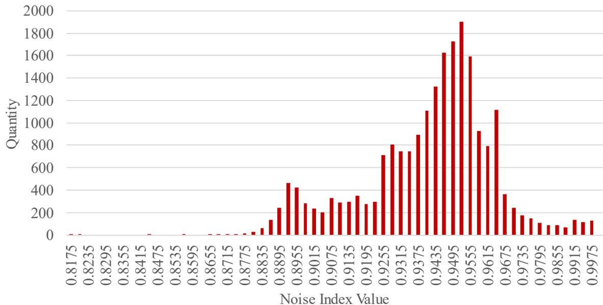
**Figure 5.28** Distribution of the noise index values for jet aircraft and turboprop aircraft (EPNdB/EPNdB)
