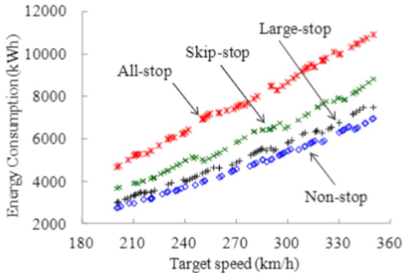
**Figure 7.10** Energy consumption of trains as a function of the target speed and the number of stops (Feng 2014)
