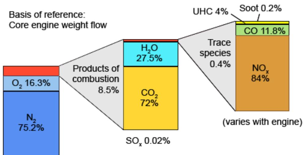
**Figure 3.5** Distribution of combustion products (adapted from Norman et al. 2003)
