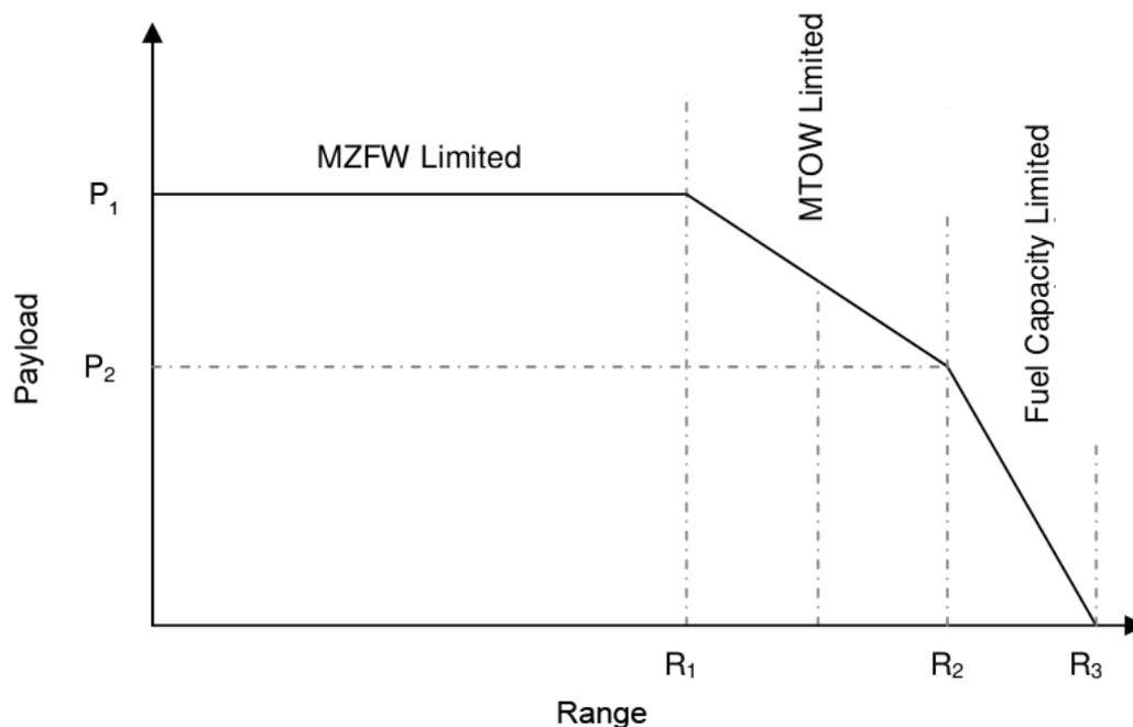
**Figure 4.2** Schematic payload/range diagram
