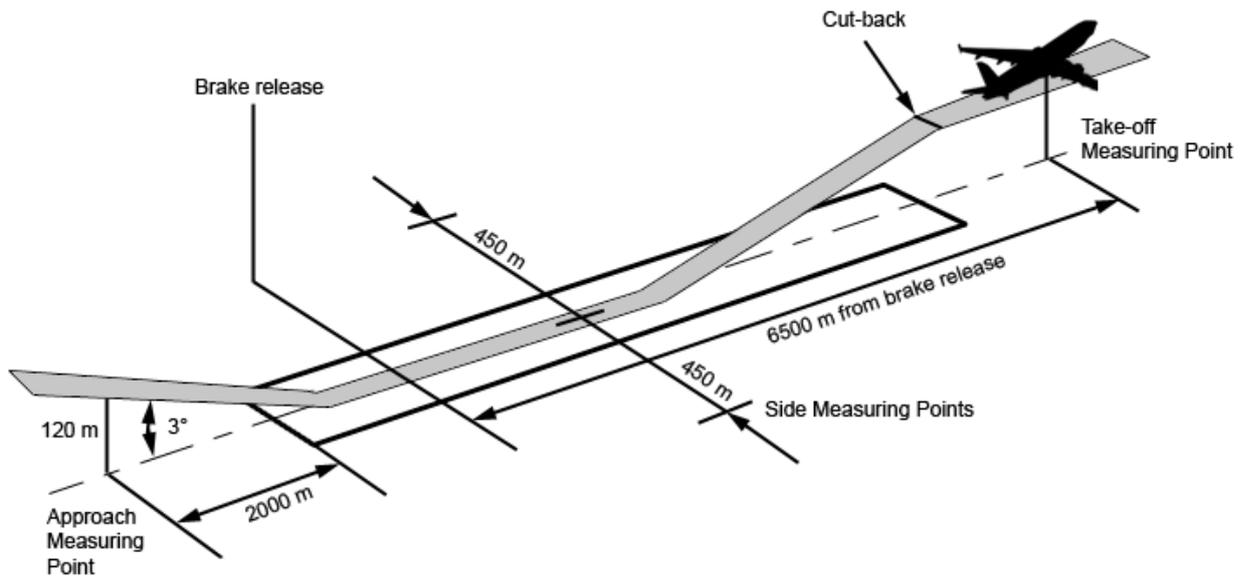
**Figure A.1** Reference points for noise measurement (based on specifications by ICAO Annex 16, Vol I)
