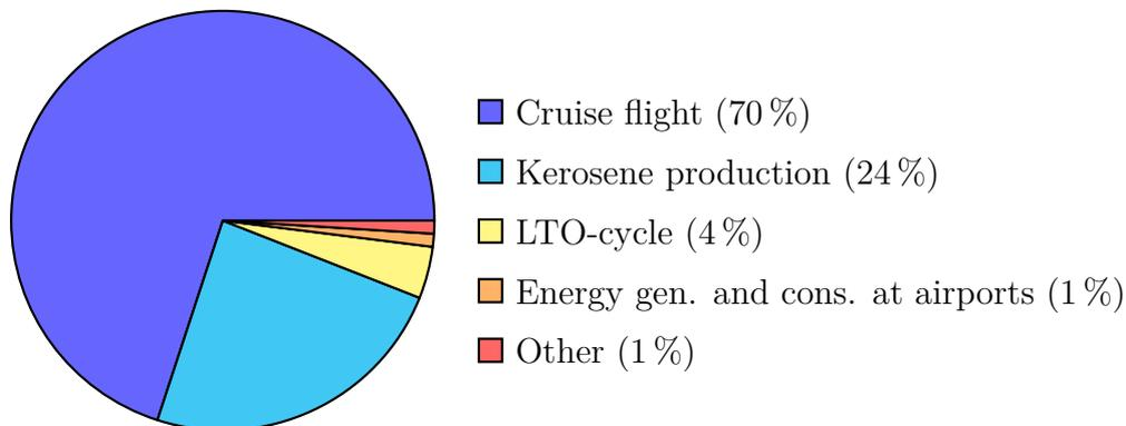
**Figure 3.2** Environmental impact of processes of an Airbus A320-200 using LCIA (Johanning 2014)
