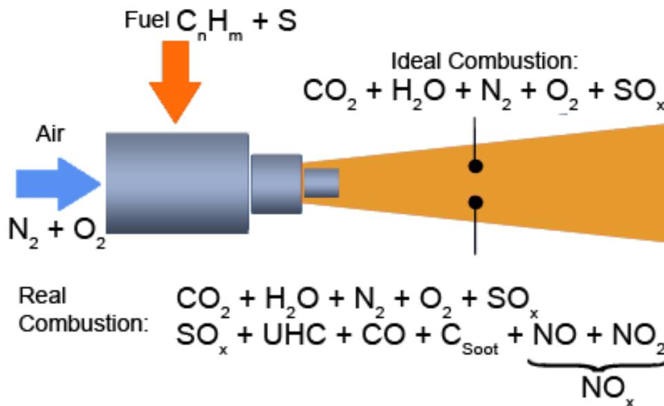
**Figure 3.4** Combustion products of a jet engine (adapted from Norman et al. 2003)
