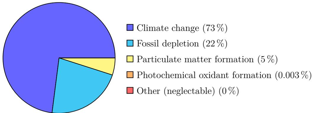
**Figure 3.3** Environmental impact by impact category of an Airbus A320-200 using LCIA (Johanning 2014)
