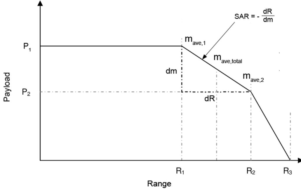
**Figure 4.3** Payload/range diagram with SAR
