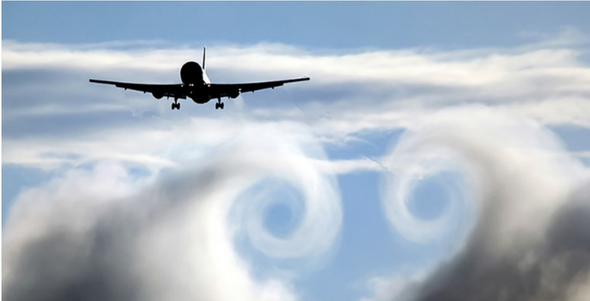
Figure 4.2 Formation of Wake Vortices Behind an Aircraft (Ewing 2025)
