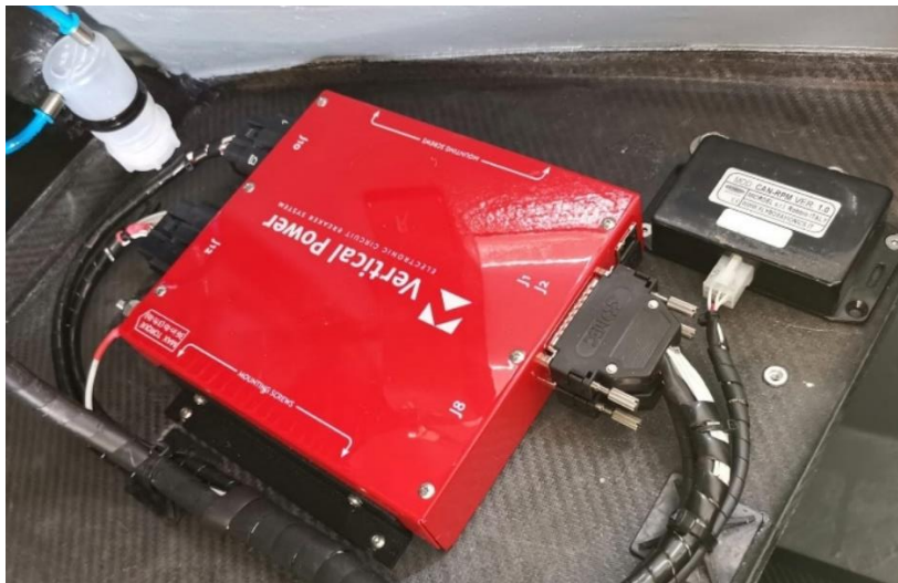
Figure 5.4 VP-X installed in the Flywhale
