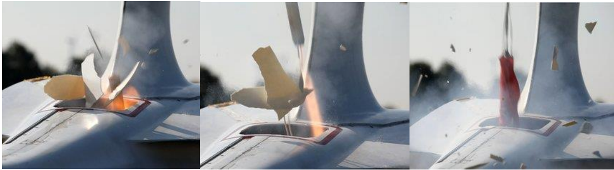
Figure 5.2 Flywhale rejection test of the BRS (2019-08-13)
