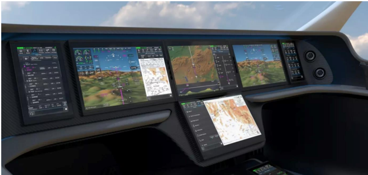
Figure 6.1 Anthem, scalable avionics system from Honeywell (Plane 2021)
