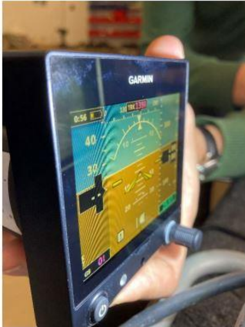
Figure 2.3 Garmin G5 reading angle at about 55°
