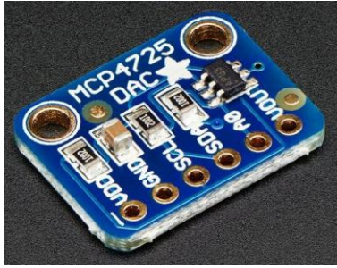
Figure 5.19 MCP4725 breakout board 12 bit DAC (Adafruit 2021)
