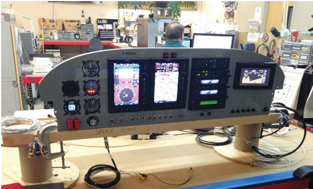
Figure 5.13 Mounted cockpit panel on a bench, front side (Bruch 2014)
