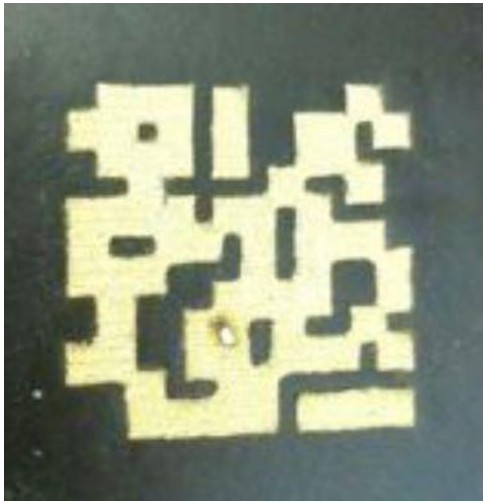
Figure 6.2 Genetically evolved patch antenna (Hope 2011, page 285)
