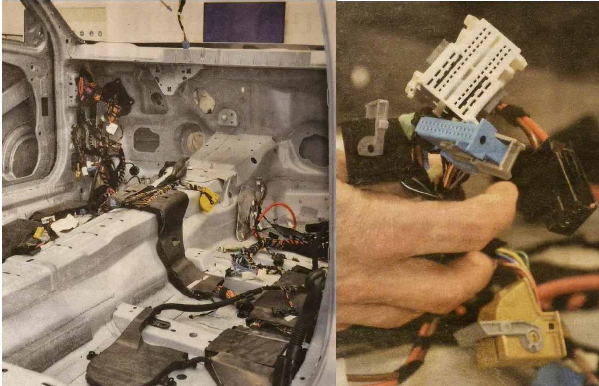
Figure 3.10 Car wiring harness (left) and plug connectors (right) (Spilok 2021)
