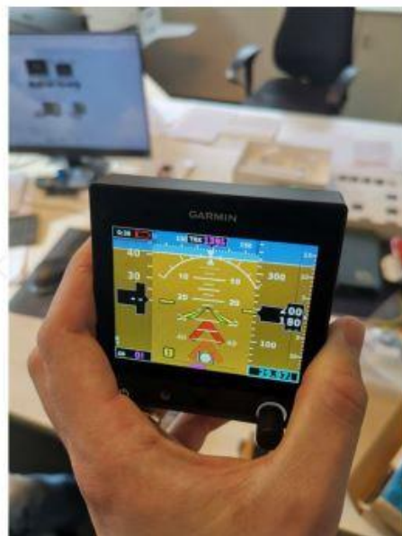
Figure 2.2 Garmin G5 at 16:44 with a with a remaining runtime of 38 min.
