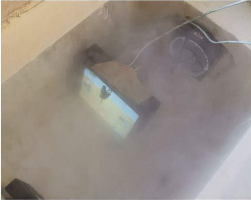
Figure 2.8 Garmin G5 in switched-on state with dry ice cooling
