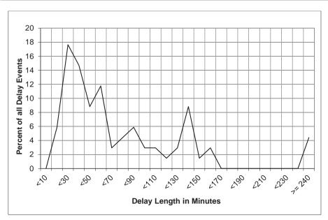
Figure 62: Delay length distribution of realistically preventable faults
