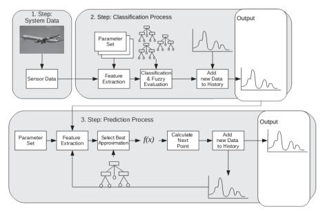
Figure 24: Monitoring and iterative prediction process
