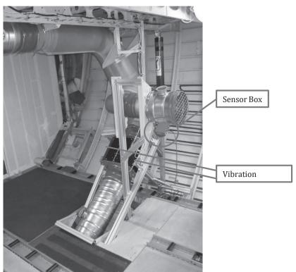
Figure 81: Airbus test rig for data recording
