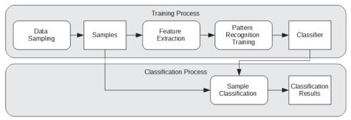
Figure 74: Condition monitoring process without optimization
