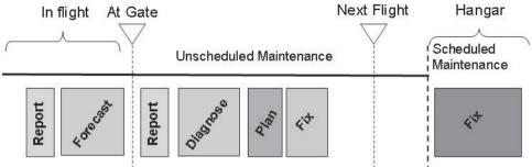
Figure 2: Unscheduled maintenance with failure forecasting
