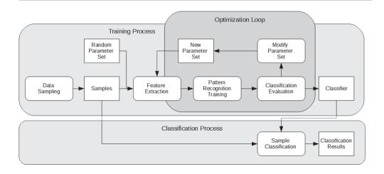
Figure 78: Condition monitoring process with parameter optimization
