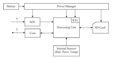
Figure 80: Data recording box architecture
