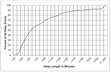
Figure 59: Cumulative delay probability of preventable faults
