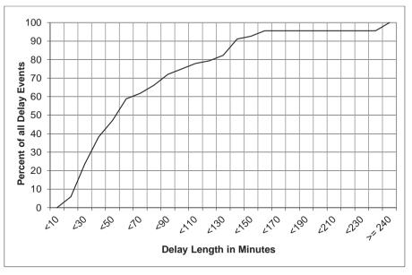
Figure 63: Cumulative delay probability of realistically preventable faults
