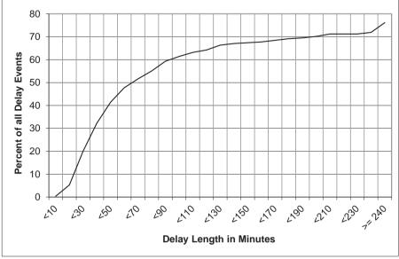
Figure 61: Cumulative delay probability of realistically non-preventable faults
