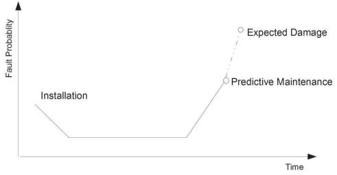
Figure 4: Machine/system condition over time (Kolerus & Wassermann, 2011)
