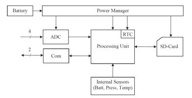
Figure 70: Data recording box architecture
