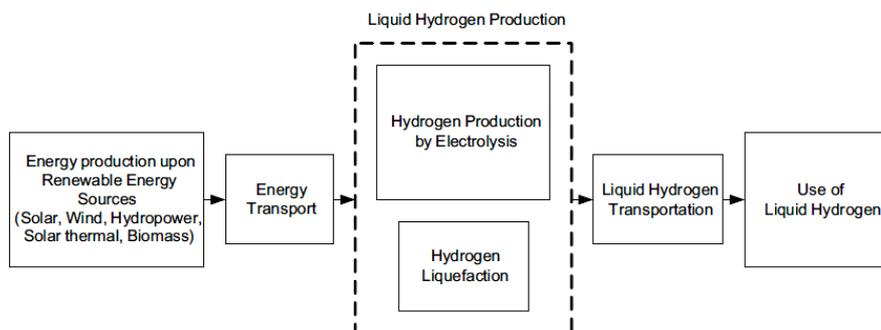
**Figure 3.4** Hydrogen liquid production based on renewable sources
