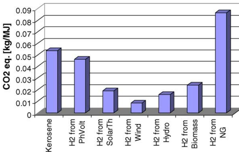
**Figure 3.3**  $CO_2$  equivalent emissions from hydrogen production (Westenberger 2003)
