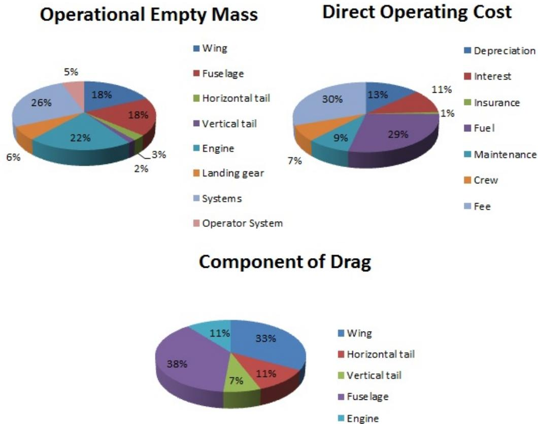
**Figure 6.1** Breakdown of the *OEW*, *DOC* and Drag Component for the A320-200
