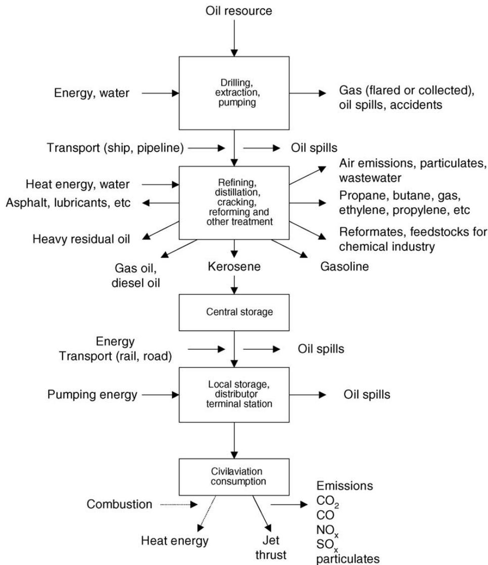
**Figure 3.2** Kerosene life cycle (Koroneos et al. 2005)
