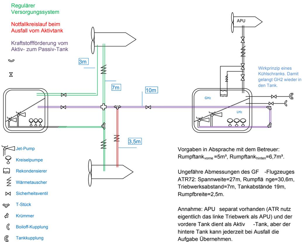
Figure 4.13 Hydrogen fuel system for ATR-72 (Batal 2010)
