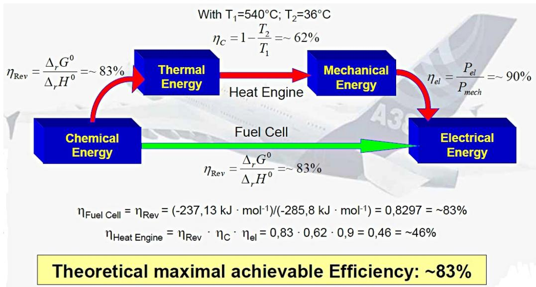
Figure A.2 Heat engine versus fuel cell (Volker 2006)
