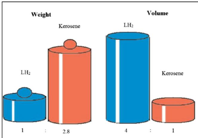
**Figure 2.12** Weight-volume comparison between hydrogen and kerosene
