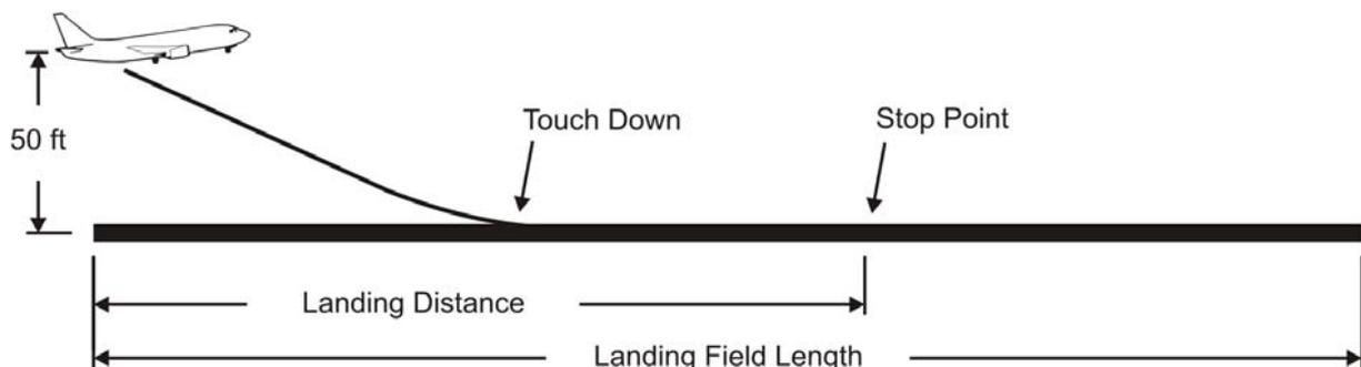
**Figure 5.1** Definition of landing field length according to CS-25 (**Scholz 2012**)
