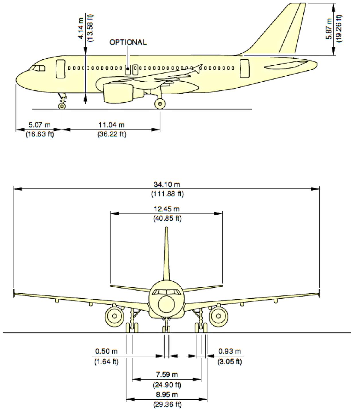
**Figure B.5** Side and front view of the A319-100 (A319 2014)
