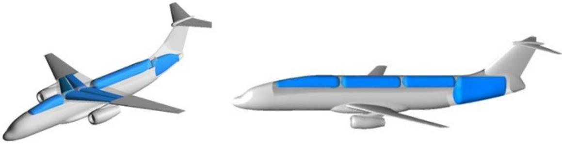
**Figure 4.9** Configurations studied during Cryoplane project (**Westenberger 2003**)
