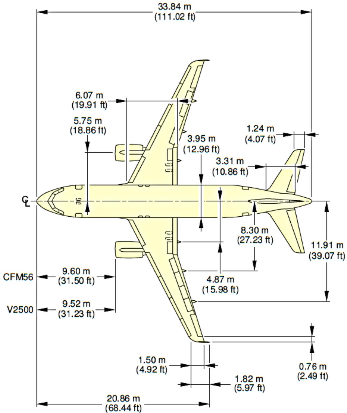
Figure B.6 Top view of the A319-100 (A319 2014)
