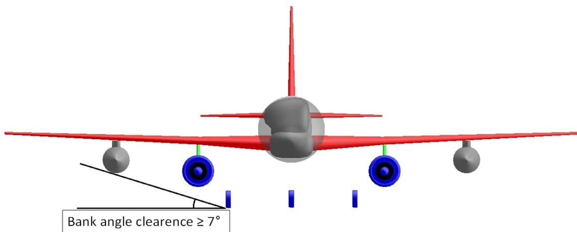
**Figure 6.9** Bank angle clearance for the wing tanks of A321-HW
