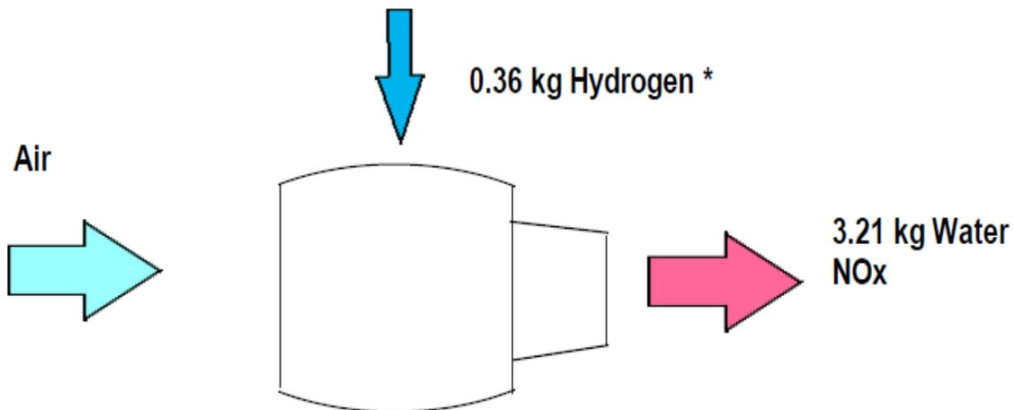
**Figure 2.11** Combustion of hydrogen in jet engine
