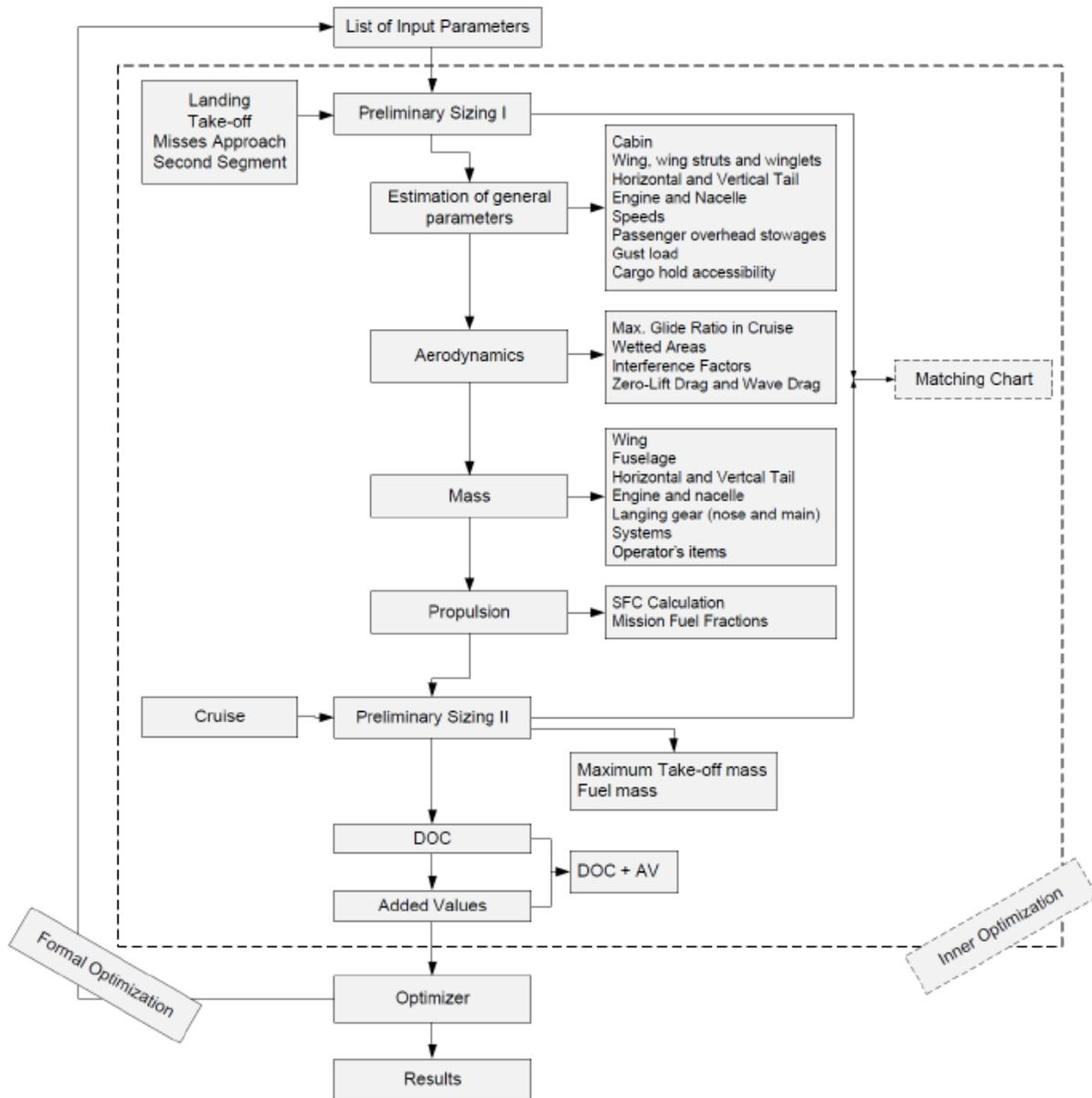
Figure 5.5 How OPerA works (Nita 2012)
