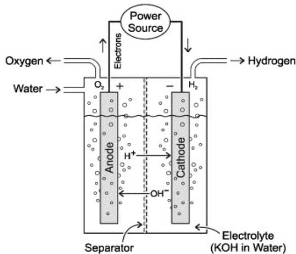
**Figure 3.5** Hydrogen production with electrolysis
