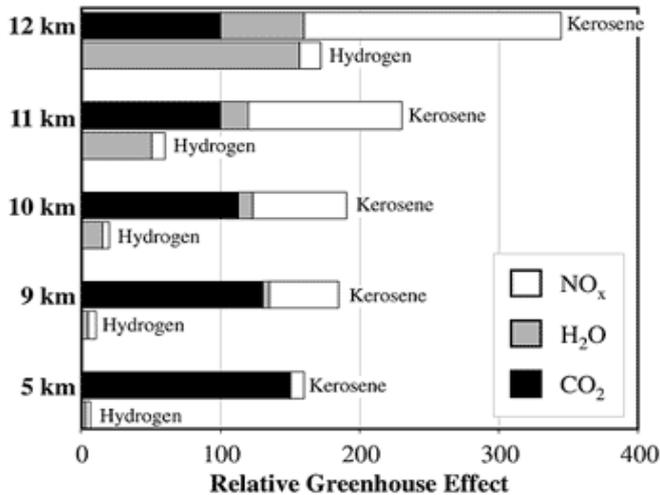
**Figure 2.14** Emissions by altitude of kerosene and hydrogen
