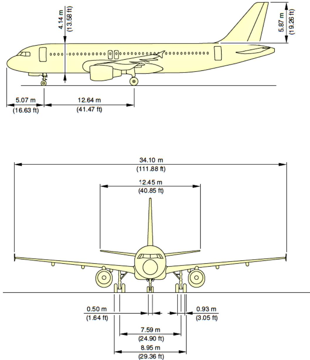
**Figure B.1** Side and front view of the A320-200 (A320 2014)
