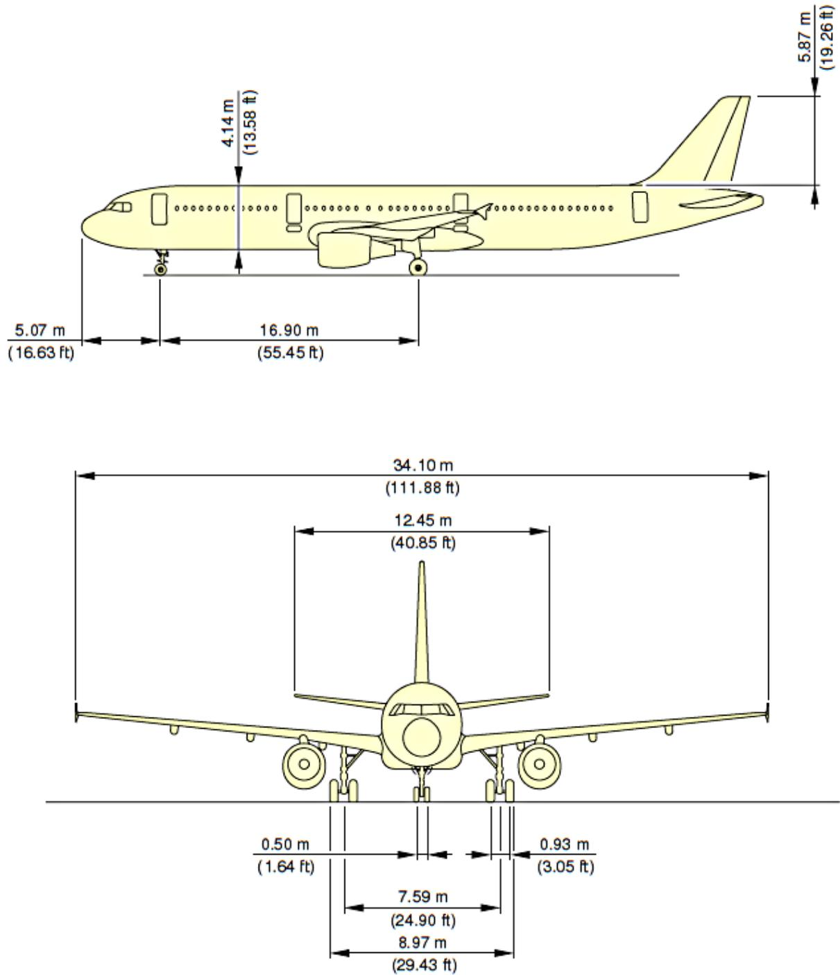
**Figure B.3** Side and front view of the A321-100 (A321 2014)
