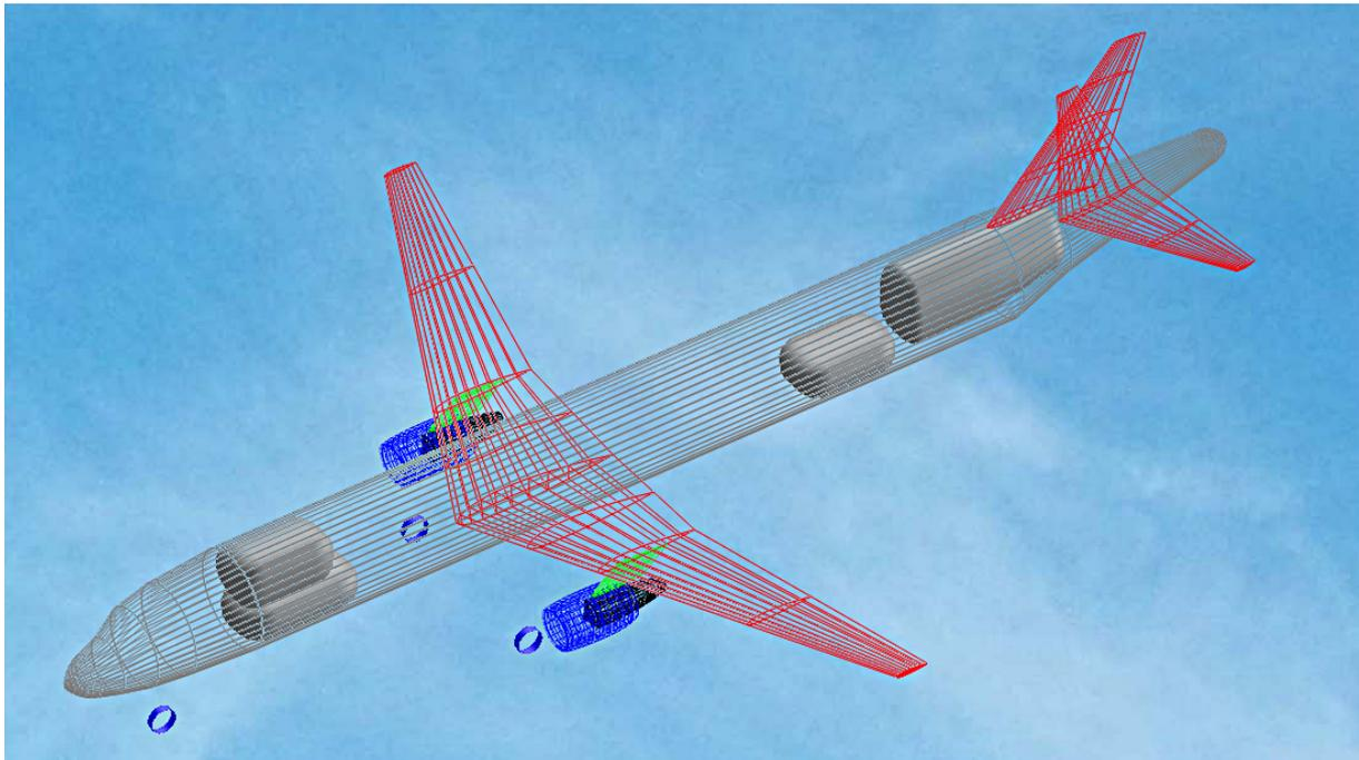
**Figure 4.10** Configuration with front and rear tanks
