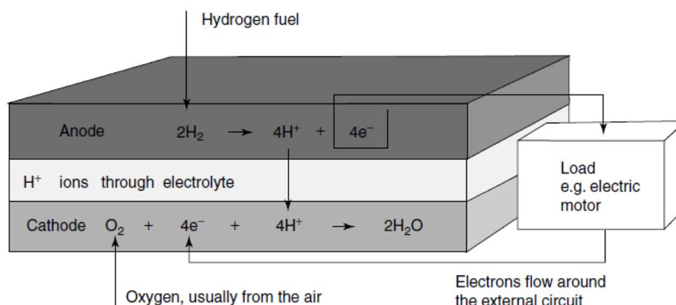
Figure A.1 Hydrogen acid electrolyte fuel cell (Larminie et al. 2003)
