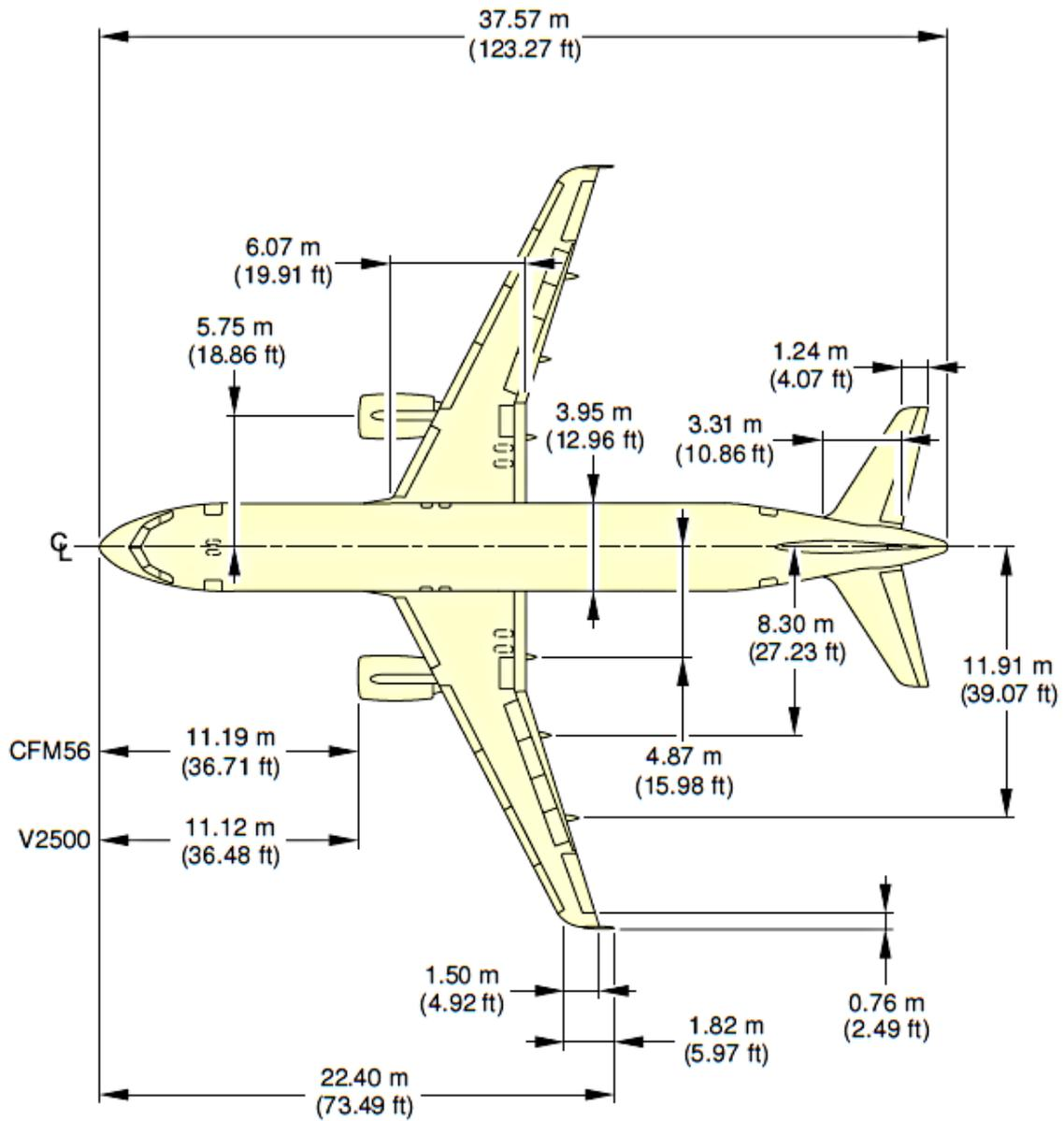
**Figure B.2** Top view of the A320-200 (A320 2014)
