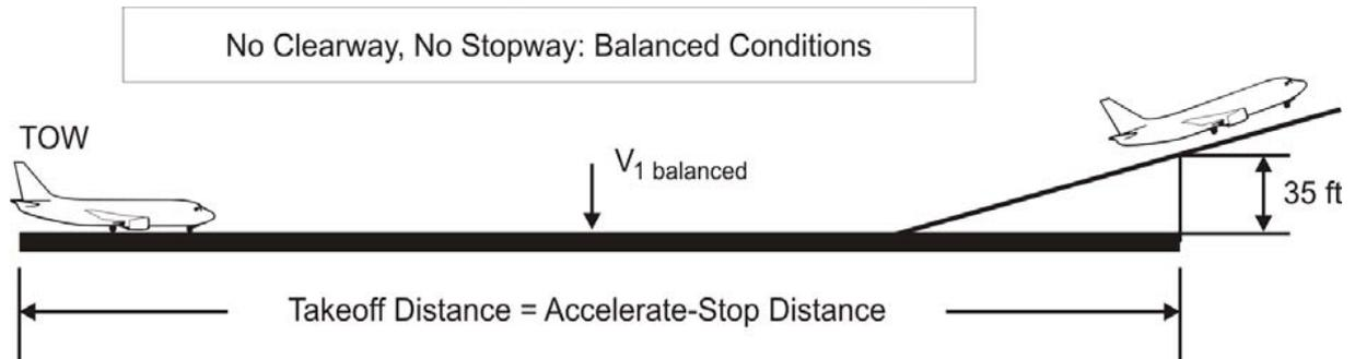
**Figure 5.2** Definition of balanced field length according to CS-25 (Scholz 2012)
