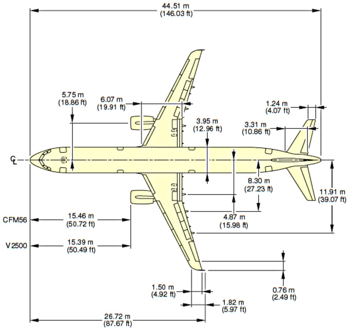
**Figure B.4** Top view of the A321-100 (A321 2014)
