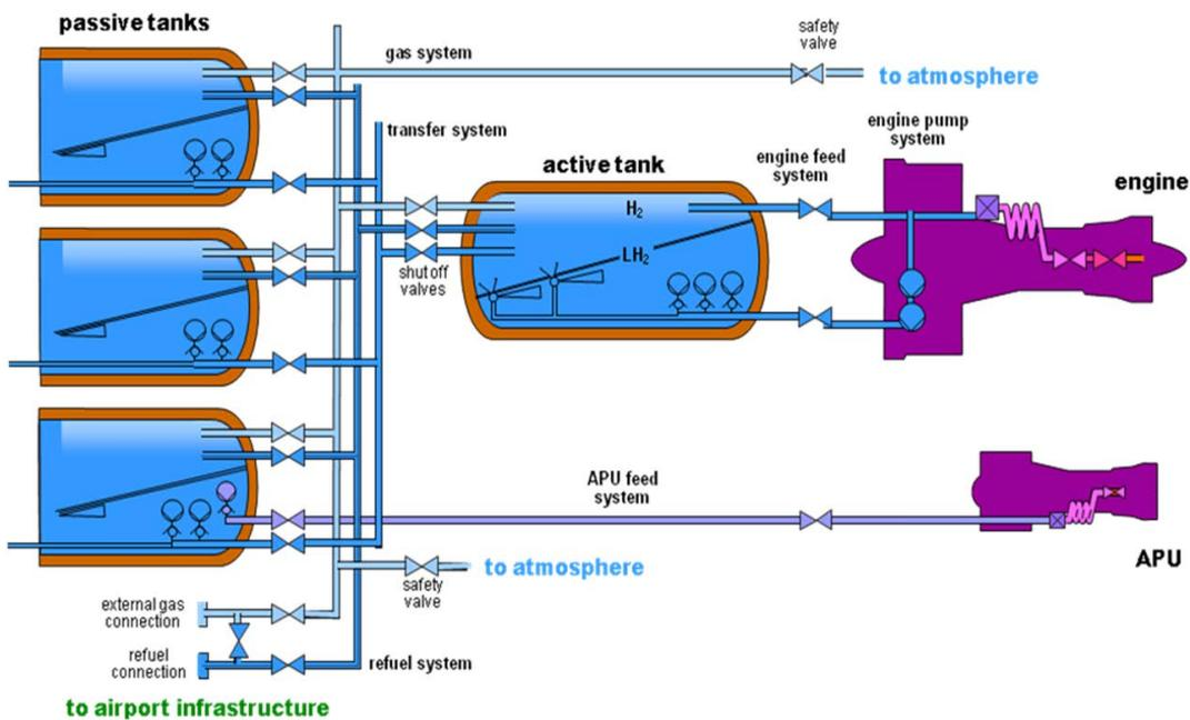
Figure 4.14 Hydrogen fuel system for A310 (Batal 2010)
