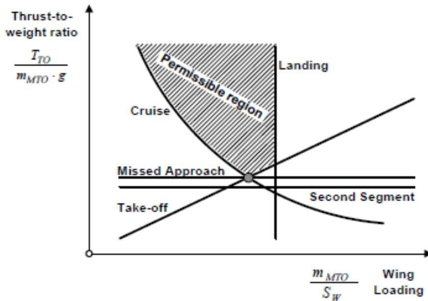
Figure 5.4 Typical Matching Chart with the design point (Nita 2012)
