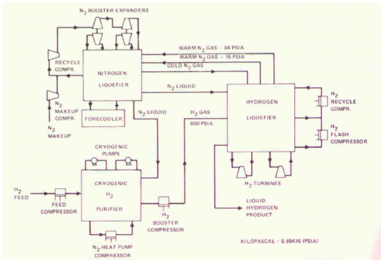
**Figure 3.6** Liquefaction process (Brewer 1991)
