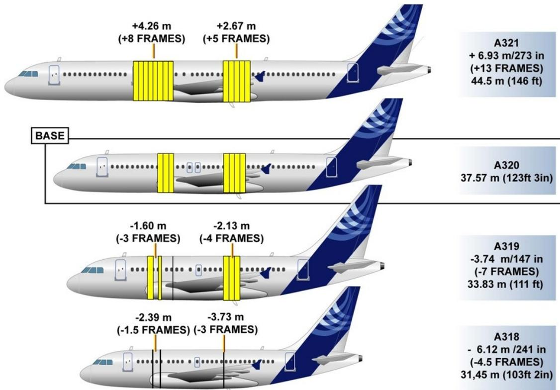
**Figure 6.3** Dimensions of the A320 family (Airbus Technical Data)
