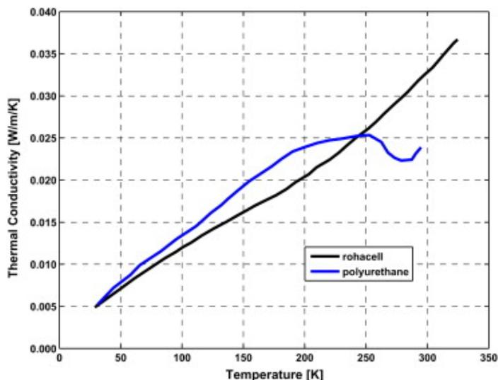
Figure 4.7 Foam thermal conductivity based on (Brewer 1991)
