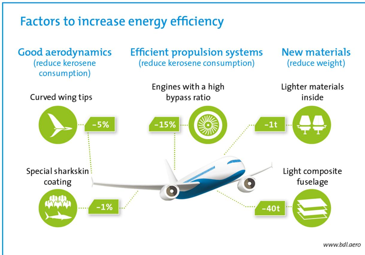
**Figure 2.10** Efficiency improvements in aircraft (BDL 2013)
