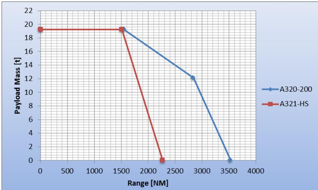
Figure 6.13 Payload-Range diagram comparison between a kerosene and a hydrogen-fueled aircraft
