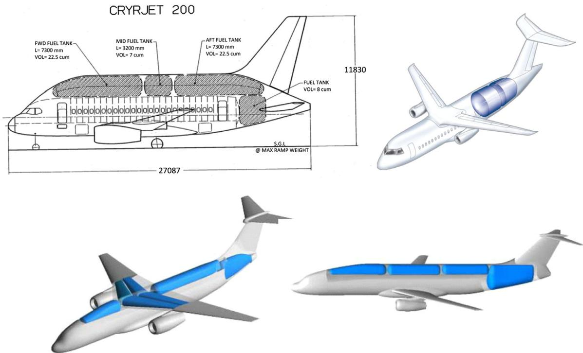
**Figure 4.3** Hydrogen aircraft with different tank configuration (Westenberger 2003)
