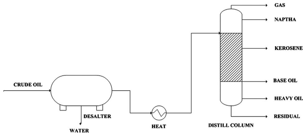
**Figure 3.1** Jet fuel process
