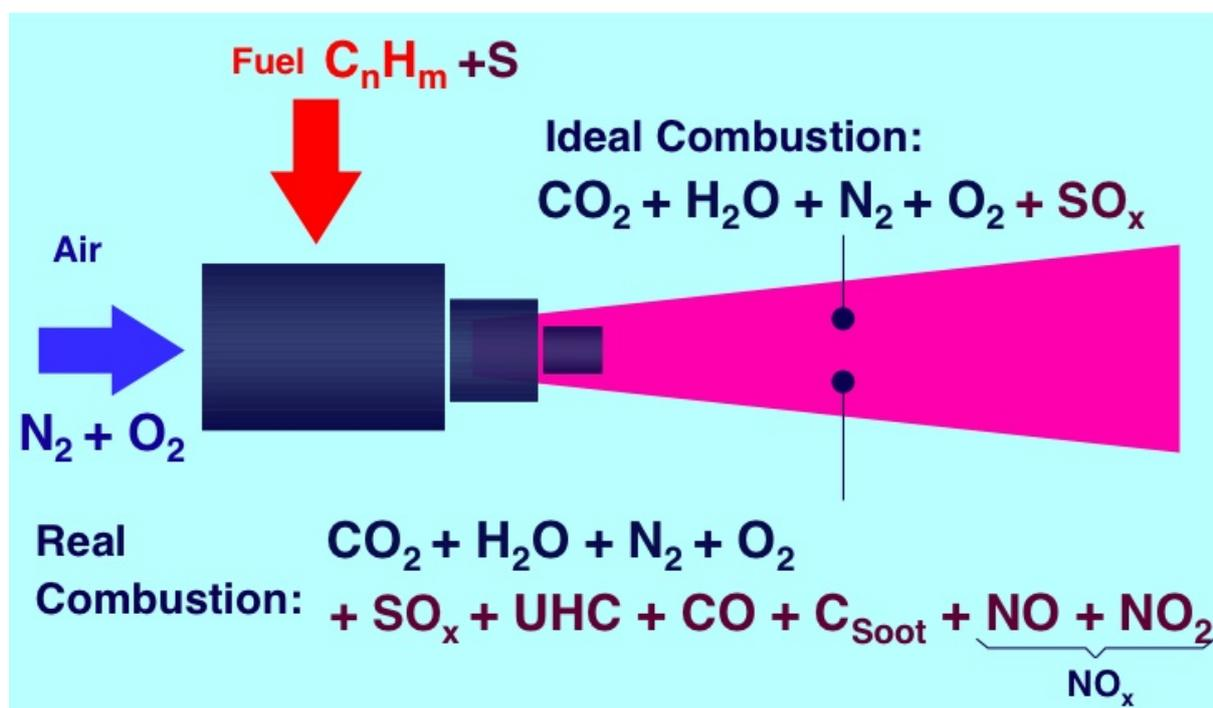
Figure 2.6 Kerosene combustion of an engine
