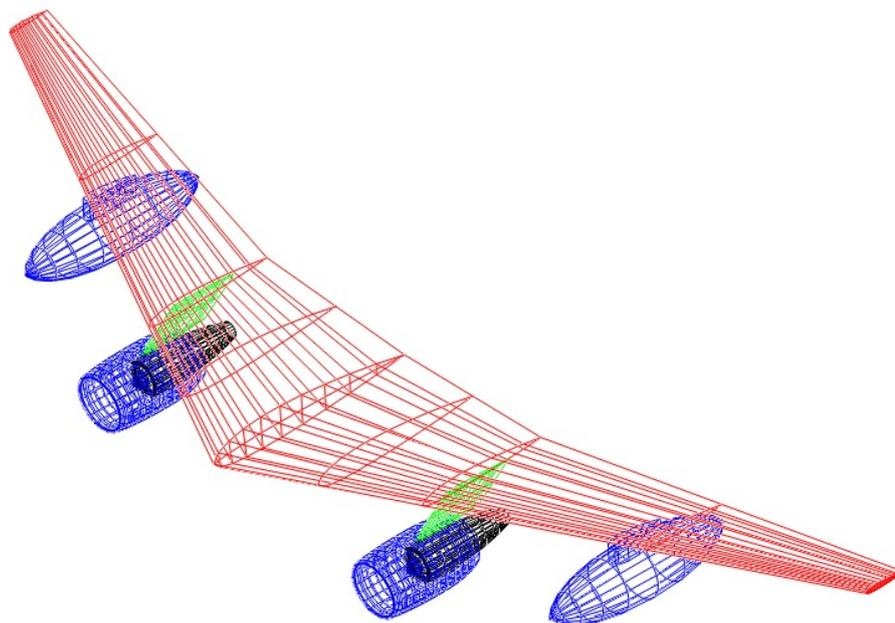
**Figure 6.6** Detailed configuration of the wing of A321-HW
