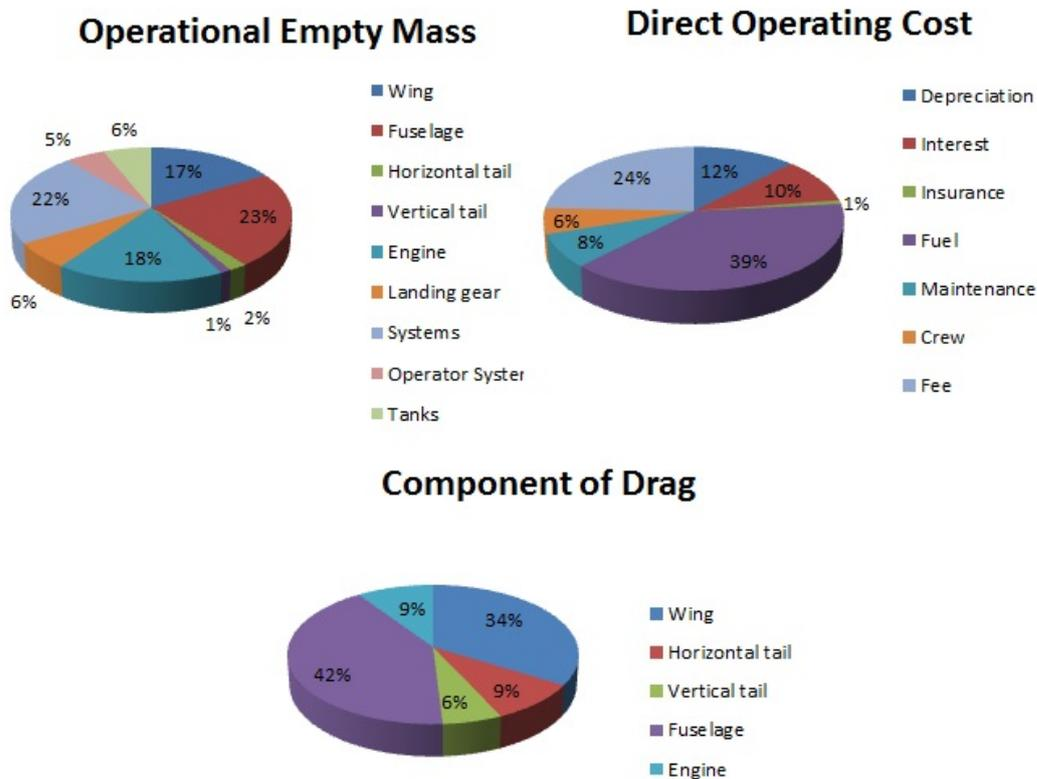
**Figure 6.5** Breakdown of the *OEW*, *DOC* and Drag Component for the A321-HS
