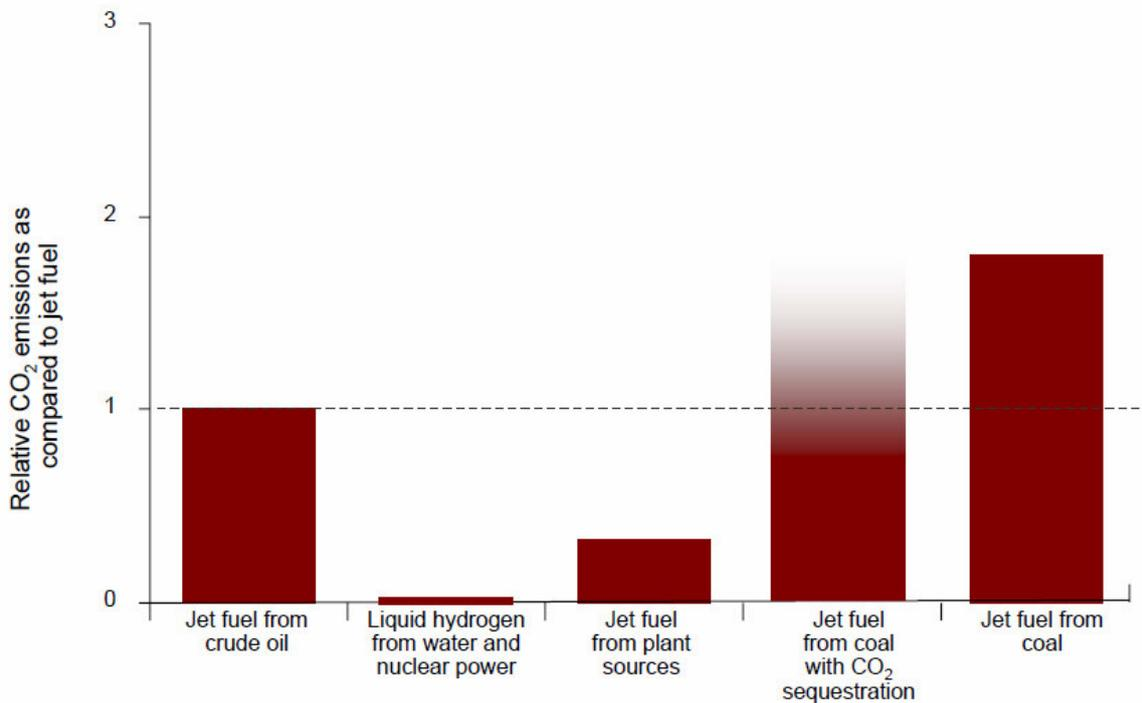
**Figure 2.13** Relative CO<sub>2</sub> emissions compared to jet fuel (Jahangir 2009)
