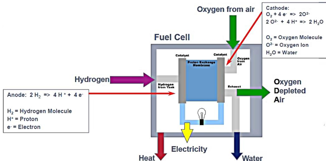
Figure A.3 PEM fuel cell scheme (Volker 2006)
