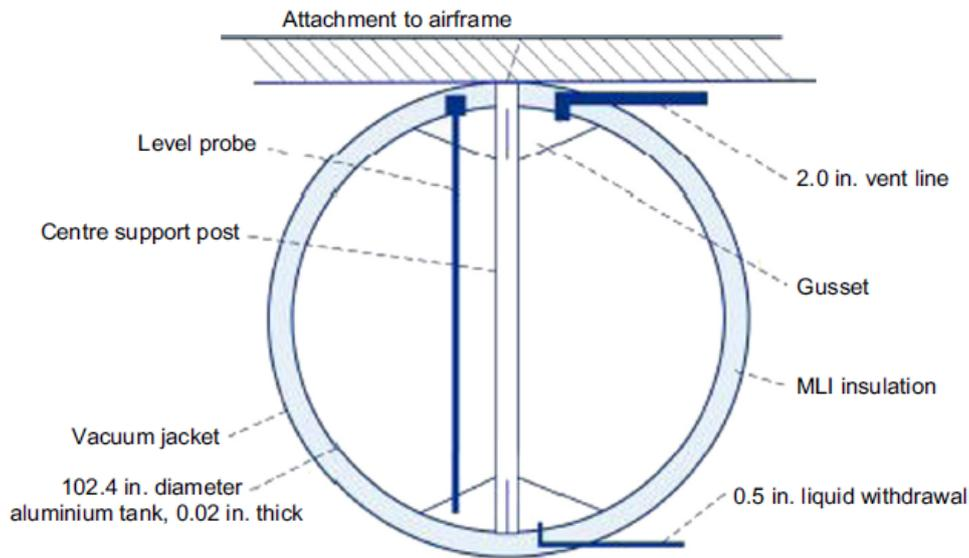
Fig. 12. Vacuum insulation system [43].
