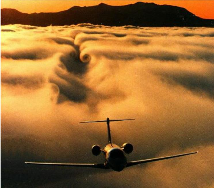
**Figure 3.2** Visible vortices behind a flying aircraft (Rill 1996)
