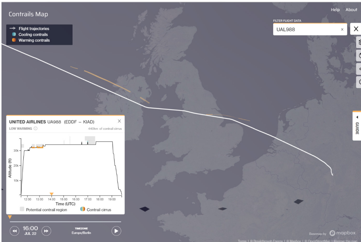
Figure 3.12: Clicking on a contrail the aircrafts track is shown in white color. Near the track some contrails can be seen colored orange. Source: Breakthrough Energy (2023b)
