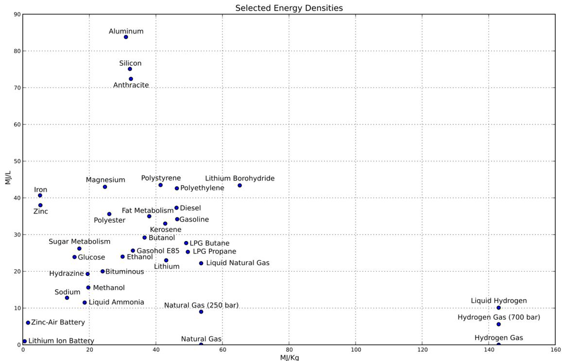
**Figure 2.2** Mass energy density vs. volume energy density (Yin 2016)
