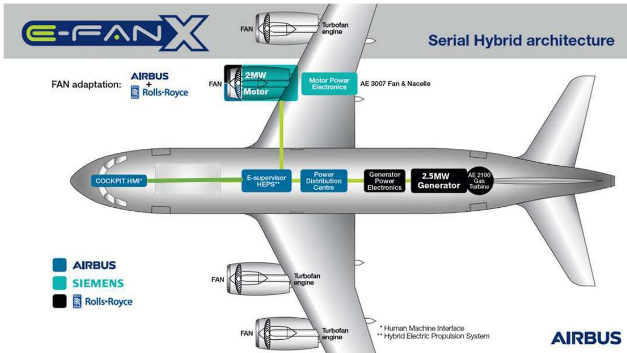
Figure 3.4 Scheme of the final configuration without battery (based on Bjorn 2017)
