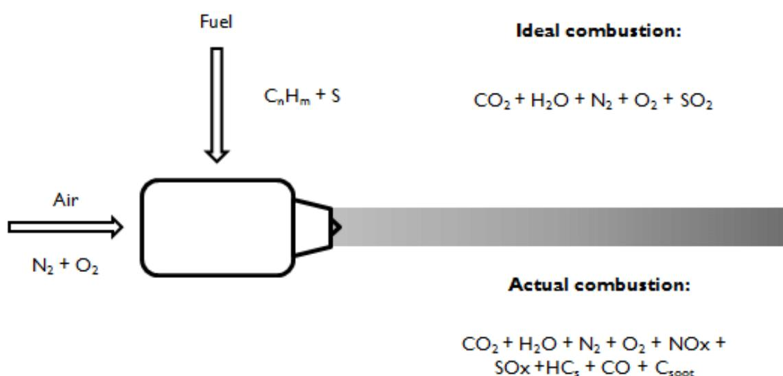
**Figure 5.1** Scheme of the jet fuel combustion (Timmis 2015)
