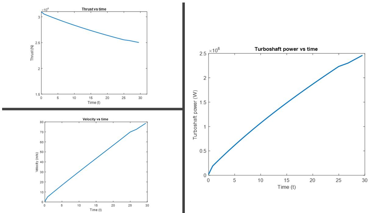
Figure 3.3 Values of velocity, thrust and power for a 2000m height take off
