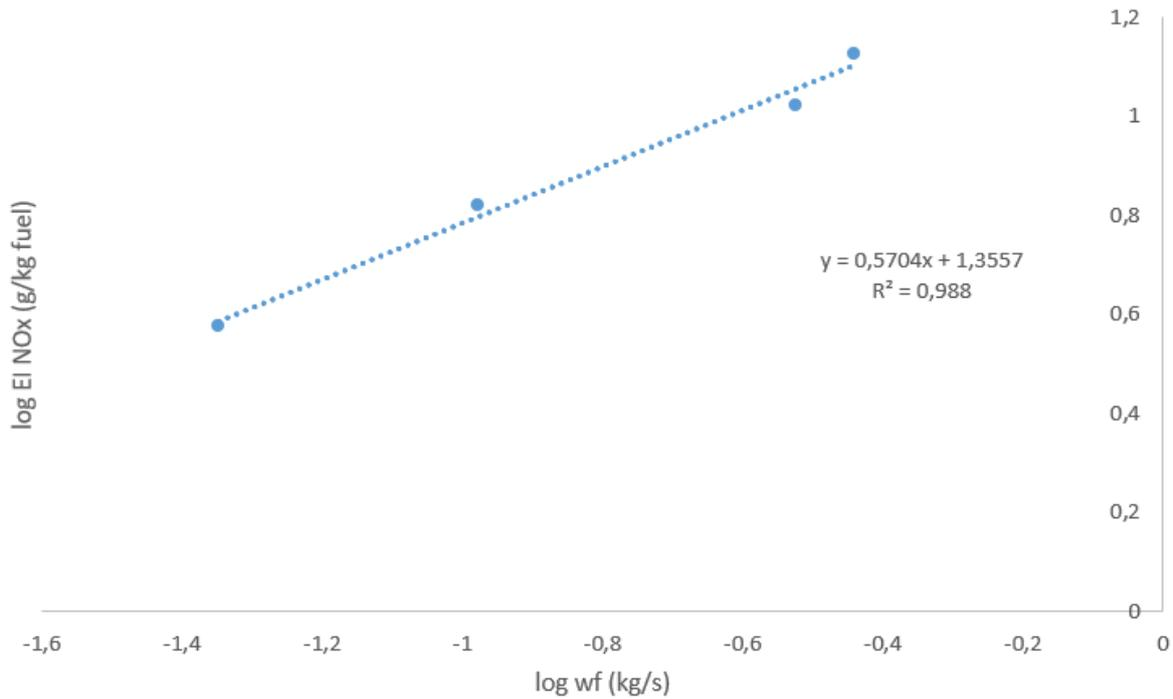
**Figure 5.5** Correlation between EI  $NO_x$  and adapted fuel flow
