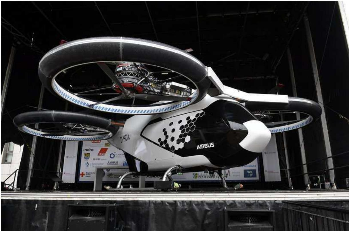
**Figure 2.5** *CityAirbus* design (Airbus 2019)
