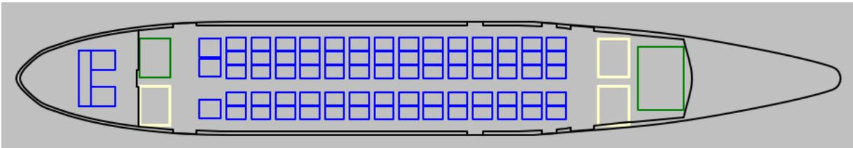
**Figure 3.7** Seat layout for the *E-FAN X* by AERO (2011)
