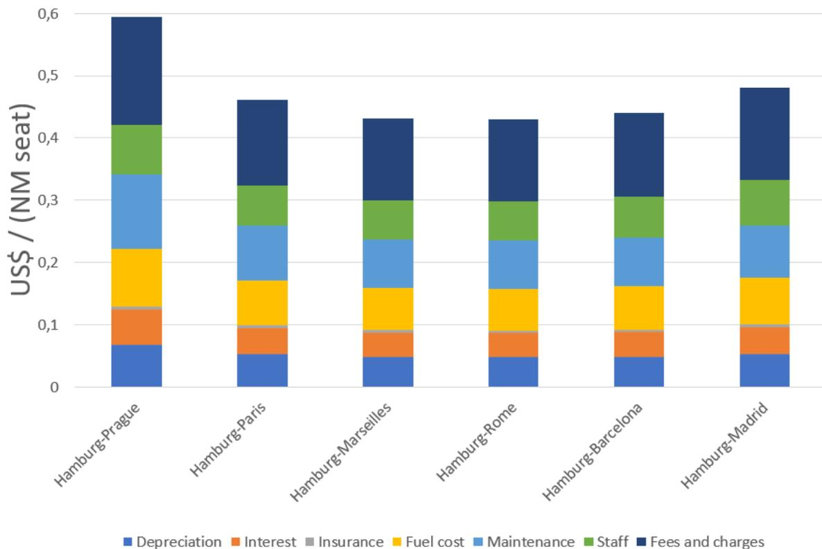
**Figure 4.5** DOC per seat mile for the *E-FAN X* with the real  $n_{pax,X}$
