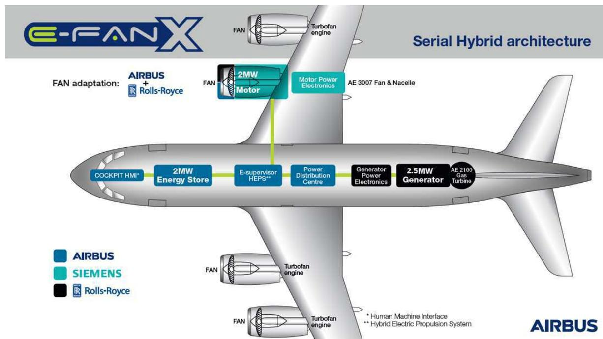
Figure 3.1 Internal configuration of the *E-FAN X* (Bjorn 2017)
