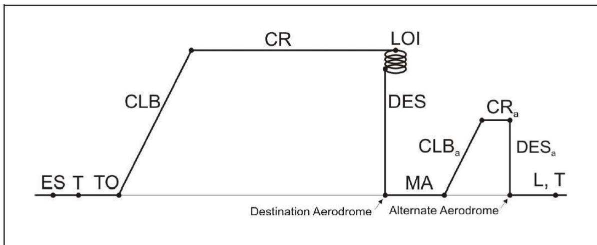
**Figure 3.5** Typical profile of a civil mission (Scholz 2019b)
