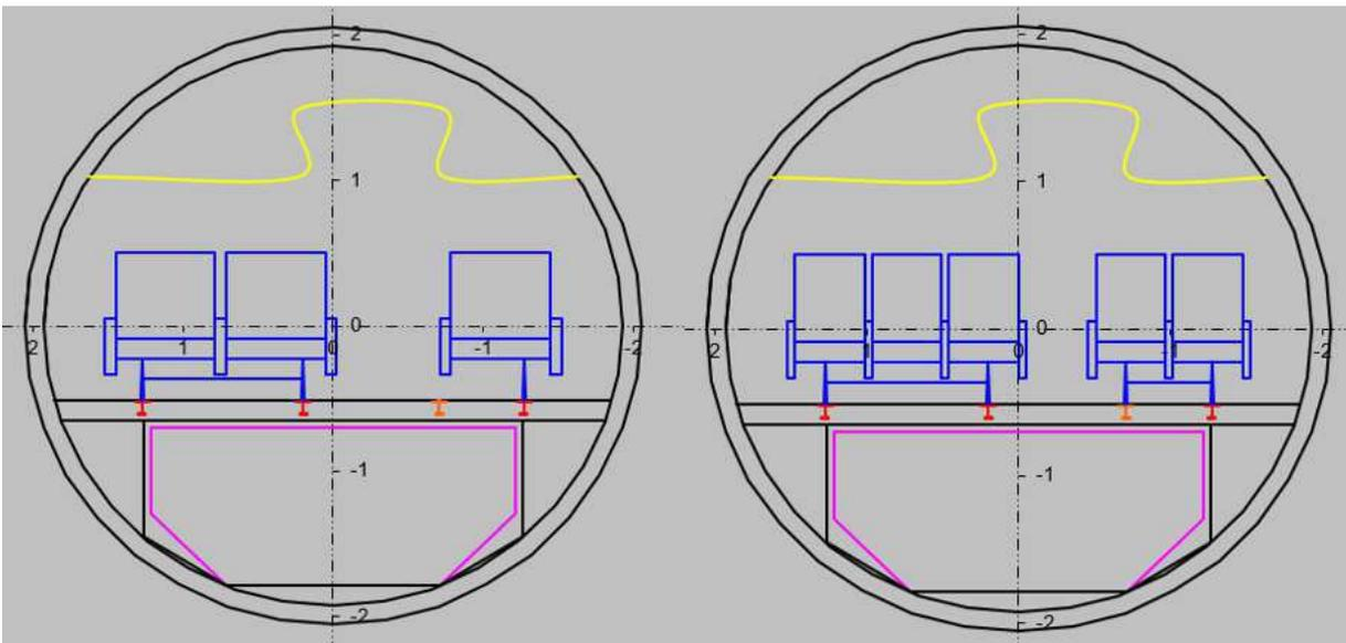
**Figure 3.8** Cross section for the *BAe 146-100* and *E-FAN X* by AERO (2011)
