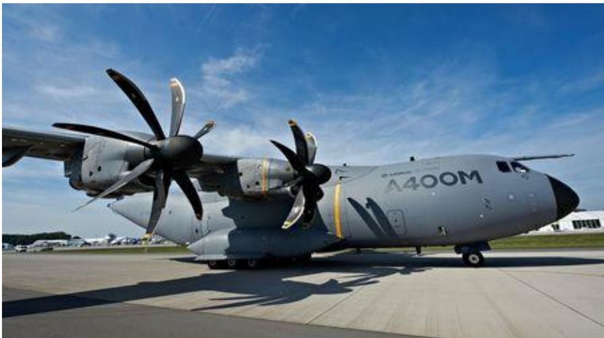
**Figure 2.2** Airbus A400M 8-blade propeller (MTU 2023)
