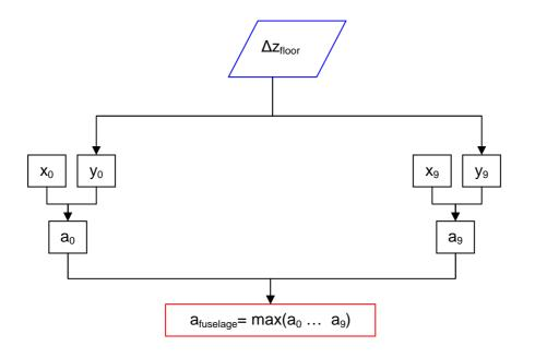
Fig. 2.54 Calculation of the *a* parameter depending on  $\Delta z_{floor}$
