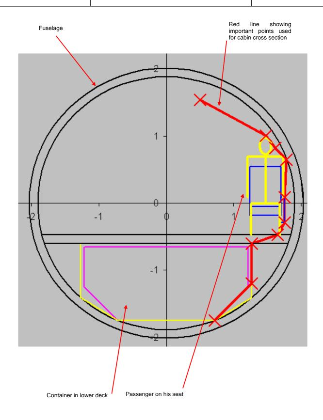
Fig. 2.11 Detailed view of the cabin cross section
