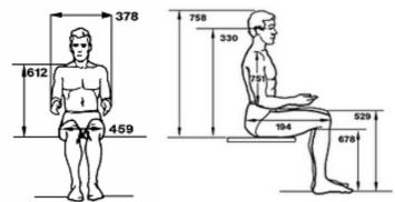
Fig. 1.8 Definition of anthropometric dimensions for American Male [NASA]
