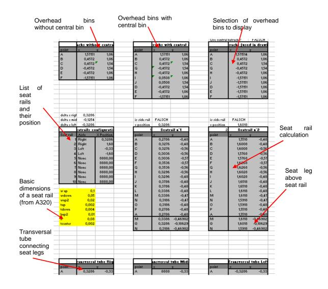
Fig. 2.38Calculation of various items coordinates for cross section display
