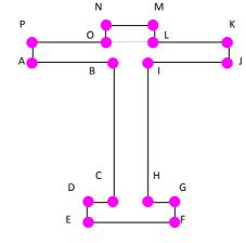
Fig. 2.36 Drawing of a seat rail
