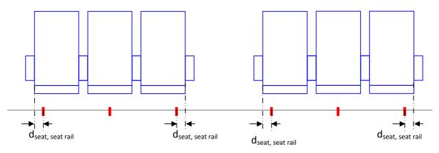
Fig. 1.13 Positioning of seat rails on a single aisle (using symmetry)
