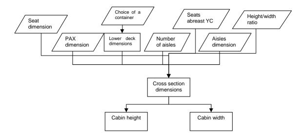
Fig. 1.11 shows how calculations are performed to find the cabin cross section dimensions.
