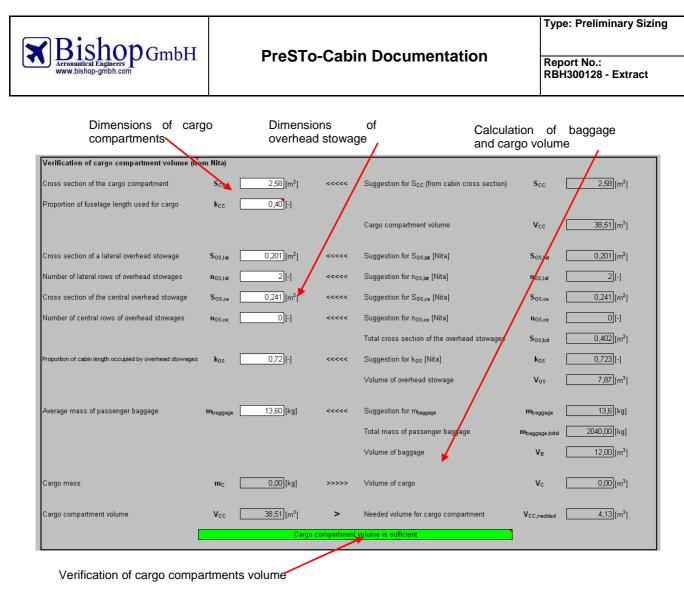
Fig. 2.23 Verification of cargo compartments volume
