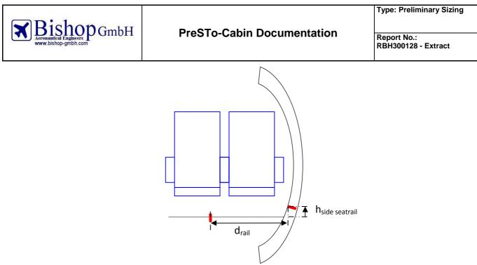
Fig. 1.14 Positioning of side seat rails
