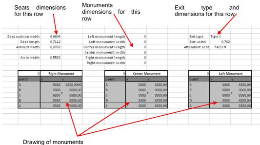
Fig. 2.44 Calculation of monuments position for cabin floor plan
