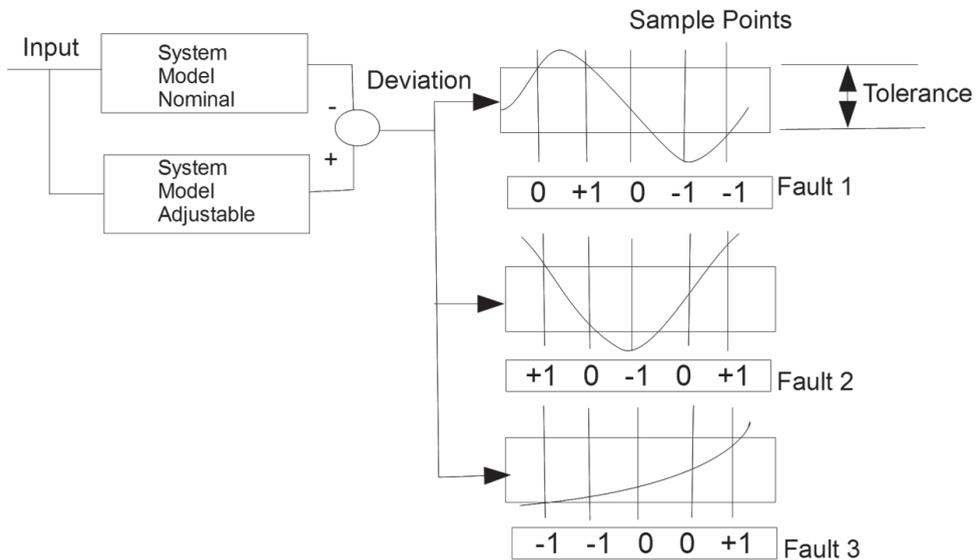
Figure 9: Fault detection with a system model (Williams, et al., 1994)
