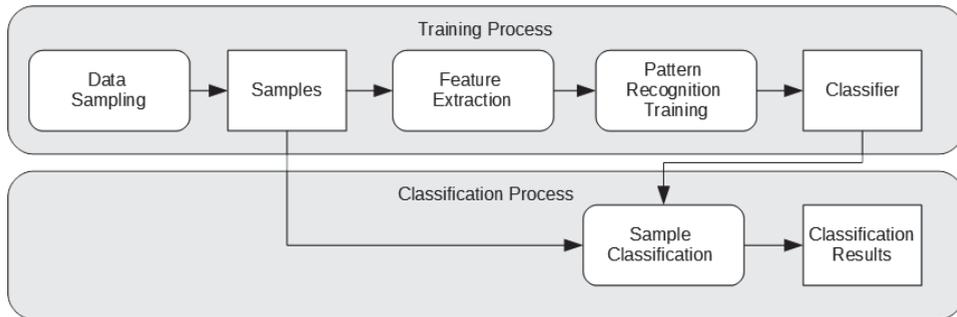
Figure 74: Condition monitoring process without optimization
