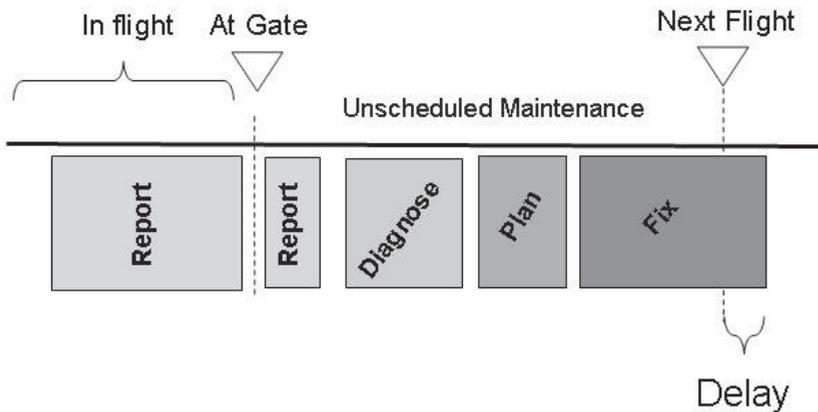
Figure 1: Unscheduled maintenance without failure forecasting
