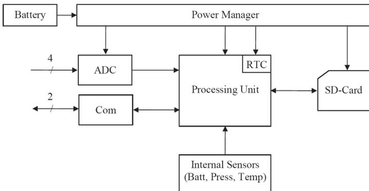
Figure 80: Data recording box architecture
