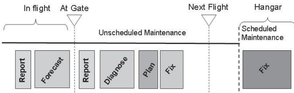
Figure 2: Unscheduled maintenance with failure forecasting
