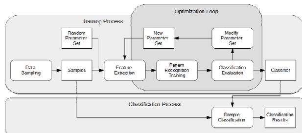
The complete process is shown in Fig. 1. The optimization takes part during the learning step, which is needed before any new data can be classified. The process starts by generating a random parameter set for the feature extraction. The calculated features are then fed into a pattern recognition algorithm that searches for patterns and learns these patterns..
