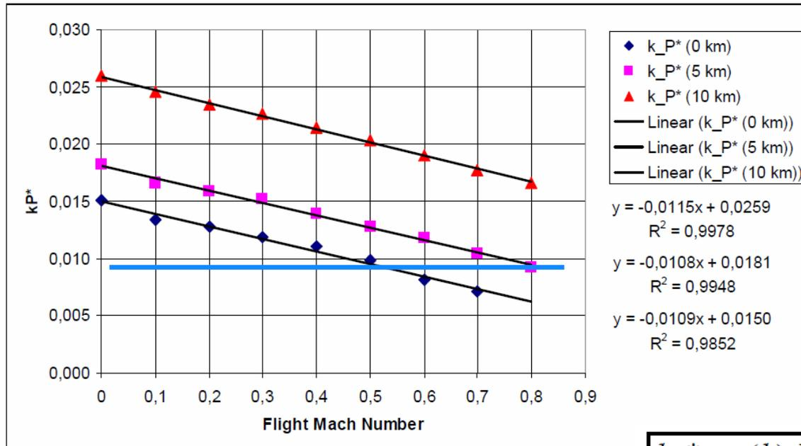
Unified  $k_P^*$  factor as function of **Mach number** and **altitude** calculated using RB211-524-D4 engine.
