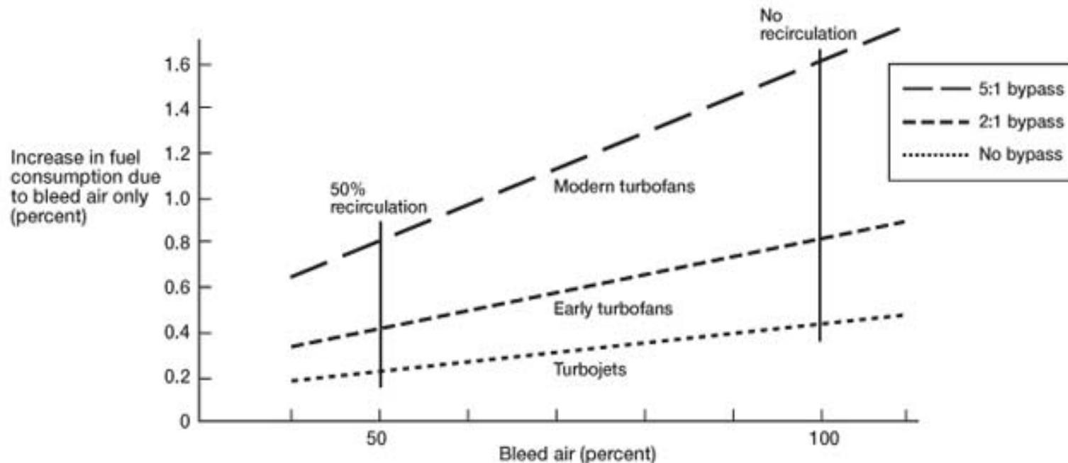
NOTE: Fuel consumption based on average performance for two engines at continuous cruise.
