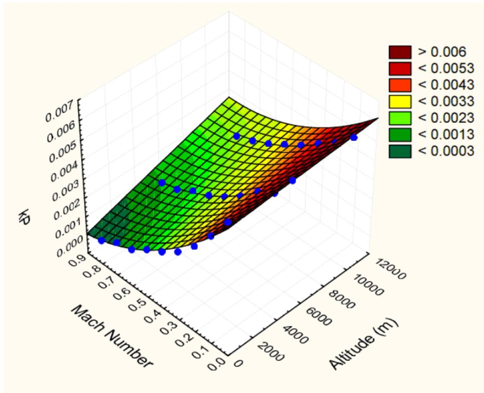
Unified  $k_p$  factor as function of **Mach number** and **altitude** calculated using RB211-524-D4 engine
