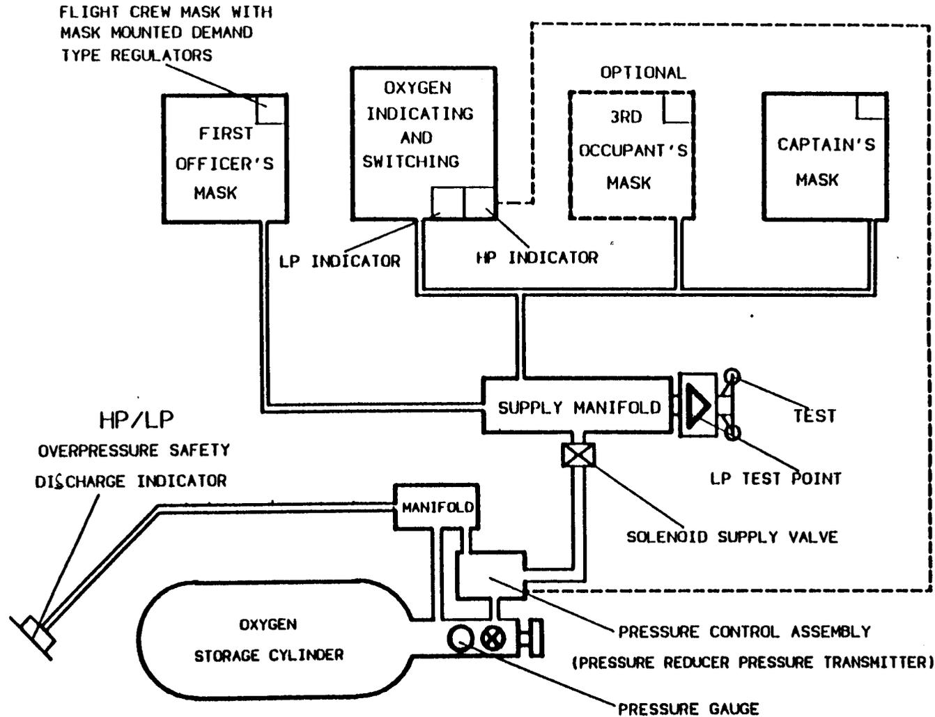
Figure 35-1 Crew Gaseous Oxygen System Schematic
