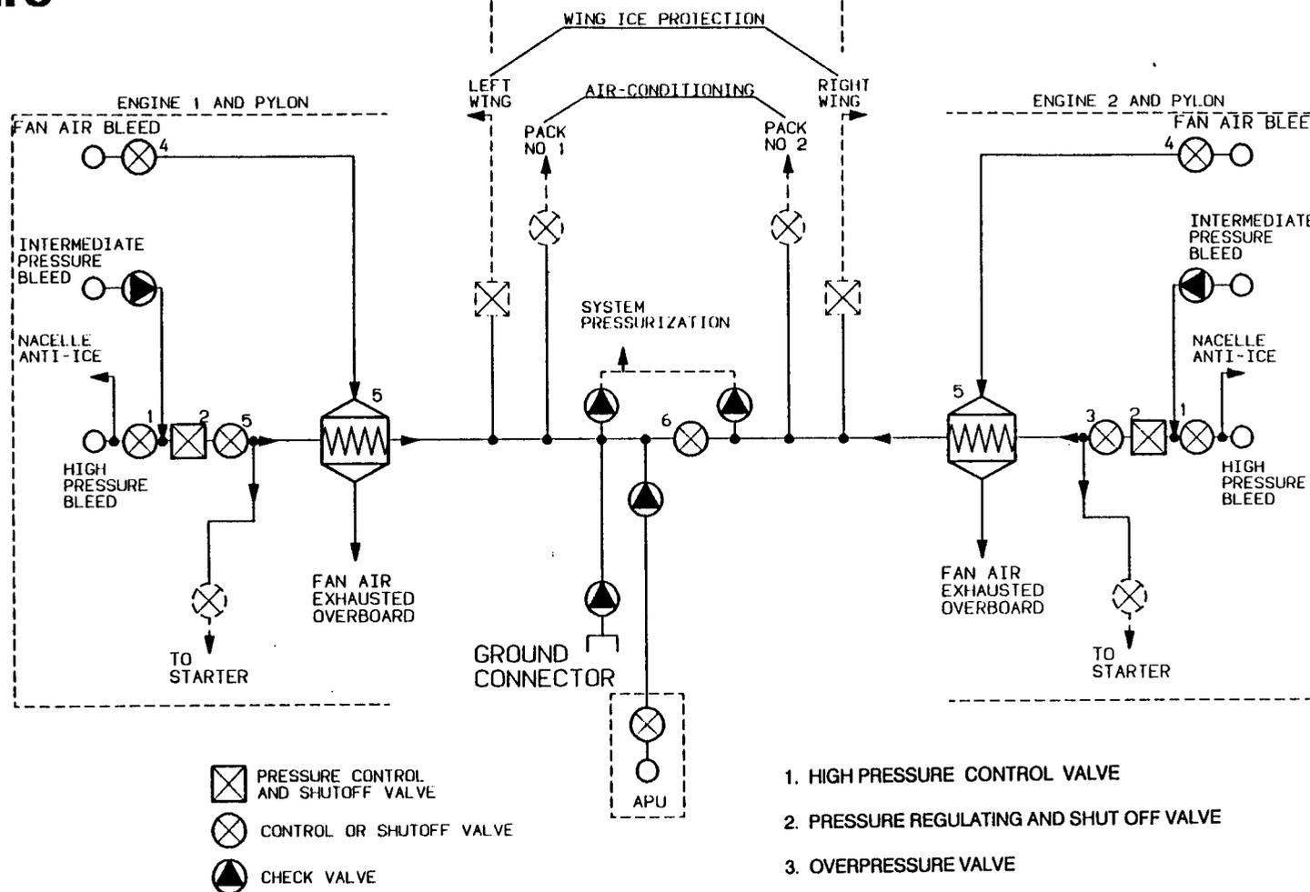
FIGURE 36.10: BLEED AIR SUPPLY-SCHEMATIC
